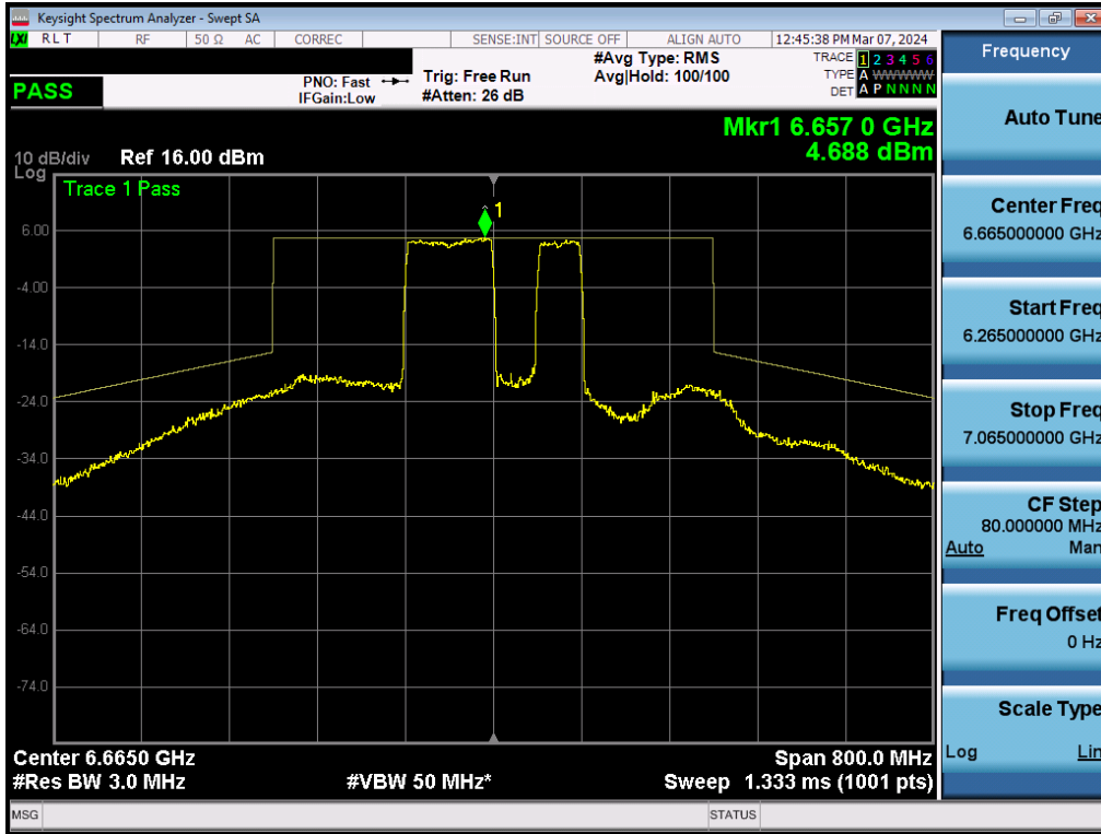
Plot 7-305. In-Band Emission Plot MIMO ANT1 (160MHz BW 802.11be (996+484 Tone) (UNII Band 7) – Ch. 143) - SP
