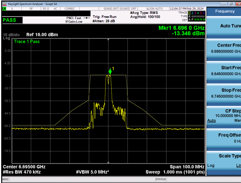
Plot 7-241. In-Band Emission Plot MIMO ANT1 (20MHz BW 802.11be (26 Tones) (UNII Band 7) – Ch. 149)
