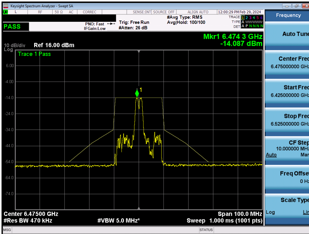
Plot 7-236. In-Band Emission Plot MIMO ANT1 (20MHz BW 802.11be (26 Tones) (UNII Band 6) – Ch. 105)
