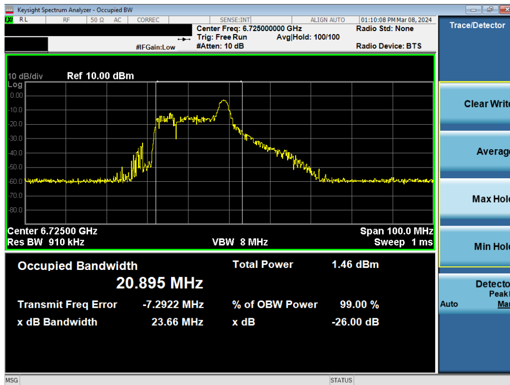
Plot 7-52. Occupied Bandwidth Plot MIMO ANT2 (40MHz BW 802. 11be (26 Tones) (UNII Band 7) – Ch. 155)
