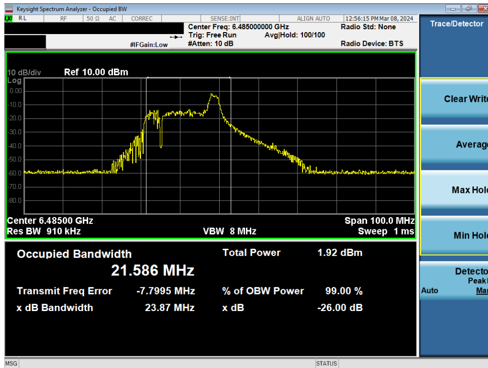
Plot 7-47. Occupied Bandwidth Plot MIMO ANT2 (40MHz BW 802. 11be (26 Tones) (UNII Band 6) – Ch. 107)
