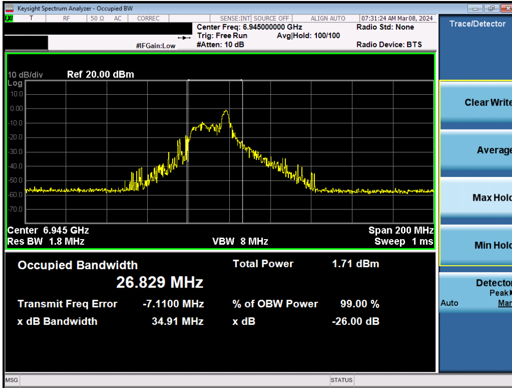
Plot 7-18. Occupied Bandwidth Plot MIMO ANT1 (80MHz BW 802. 11be (26 Tones) (UNII Band 8) – Ch. 199)
