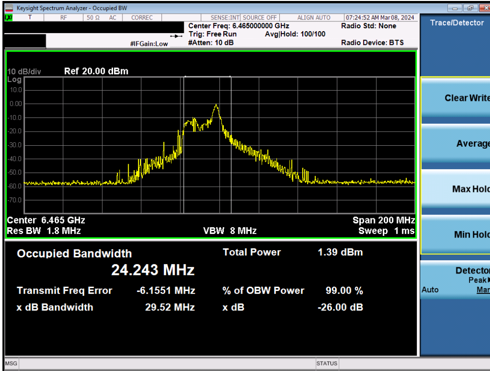
Plot 7-8. Occupied Bandwidth Plot MIMO ANT1 (80MHz BW 802. 11be (26 Tones) (UNII Band 6) – Ch. 103)
