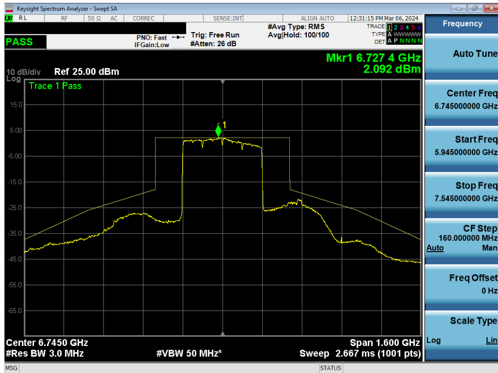
Plot 7-185. In-Band Emission MIMO ANT2 (320MHz 802.11ax/be (UNII Band 6/7) – Ch. 159) - SP
