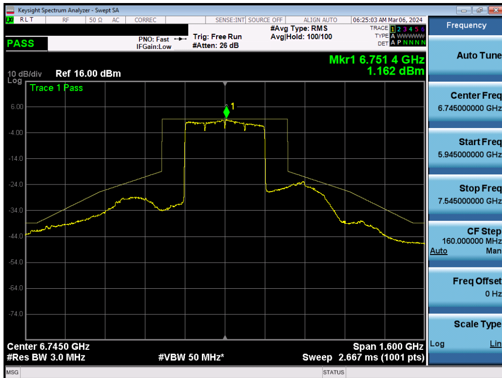
Plot 7-161. In-Band Emission MIMO ANT1 (320MHz 802.11ax/be (UNII Band 6/7) – Ch. 159) - SP
