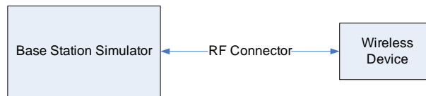
Figure 8-3 Power Measurement Setup – NR Online
