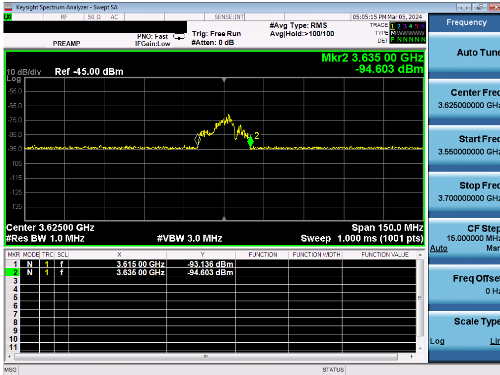
Plot 7-145. Run#1 End User Device Frequency of Operations
