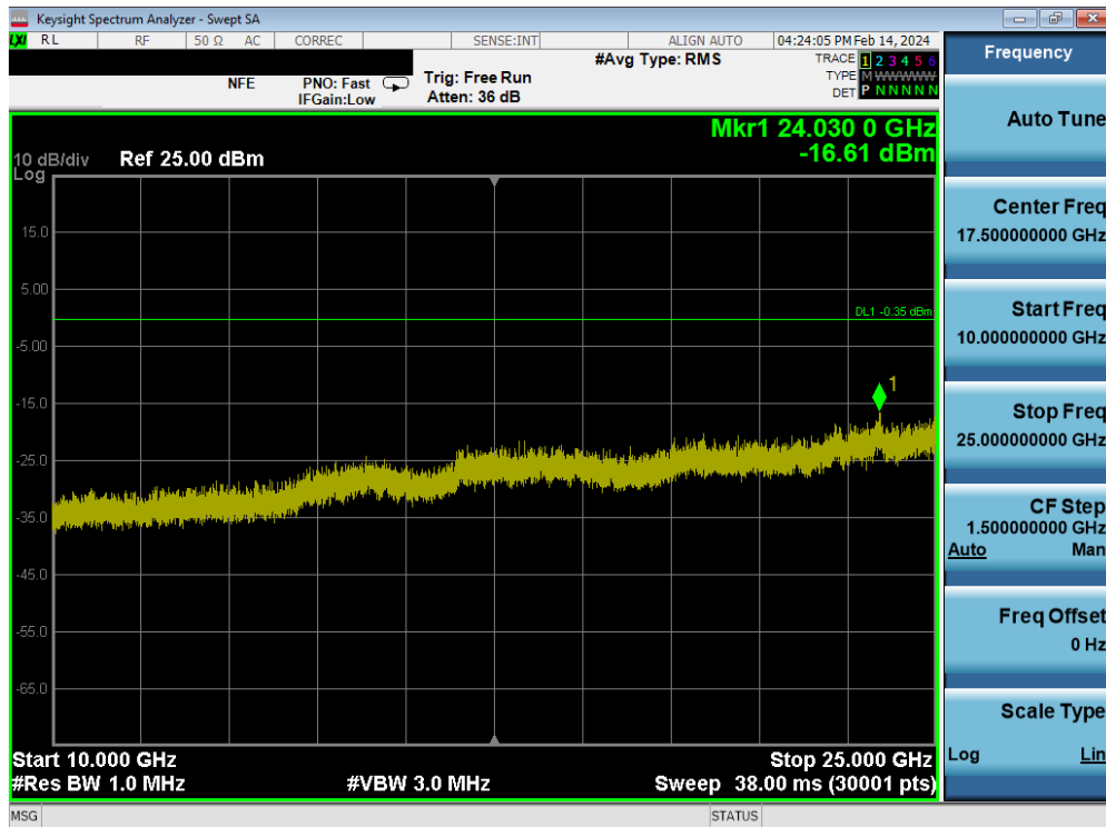
Plot 7-148. Conducted Spurious Plot (Bluetooth, 3Mbps – Ch. 0)
