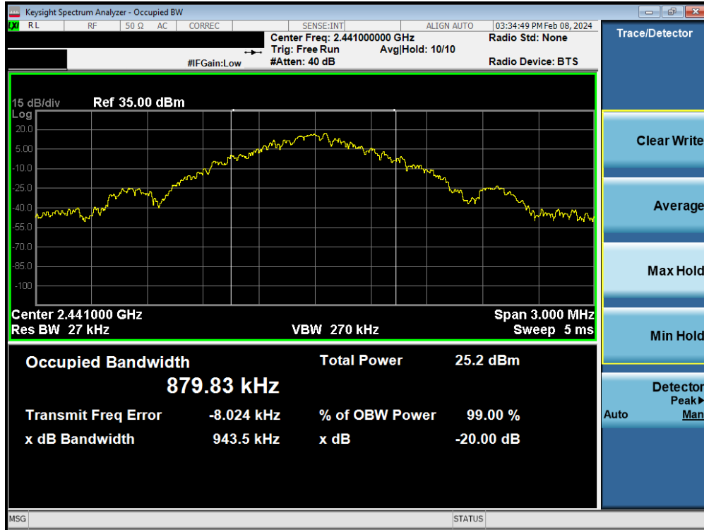
Plot 7-2. 20dB Bandwidth Plot (Bluetooth, 1Mbps – Ch. 39)
