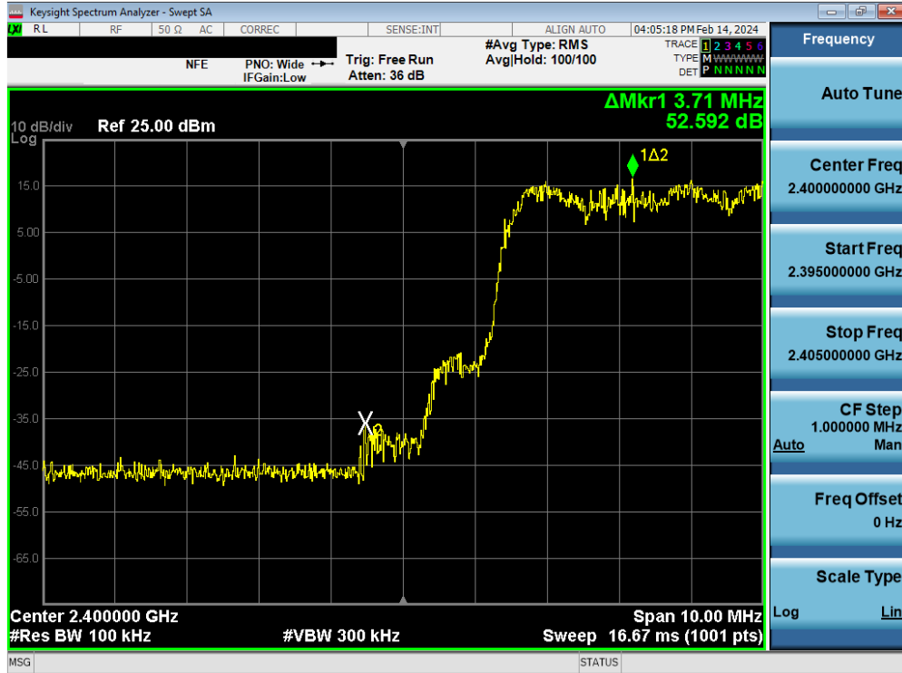
Plot 7-111. Band Edge Plot (Bluetooth with Hopping Enabled, 3 Mbps)
