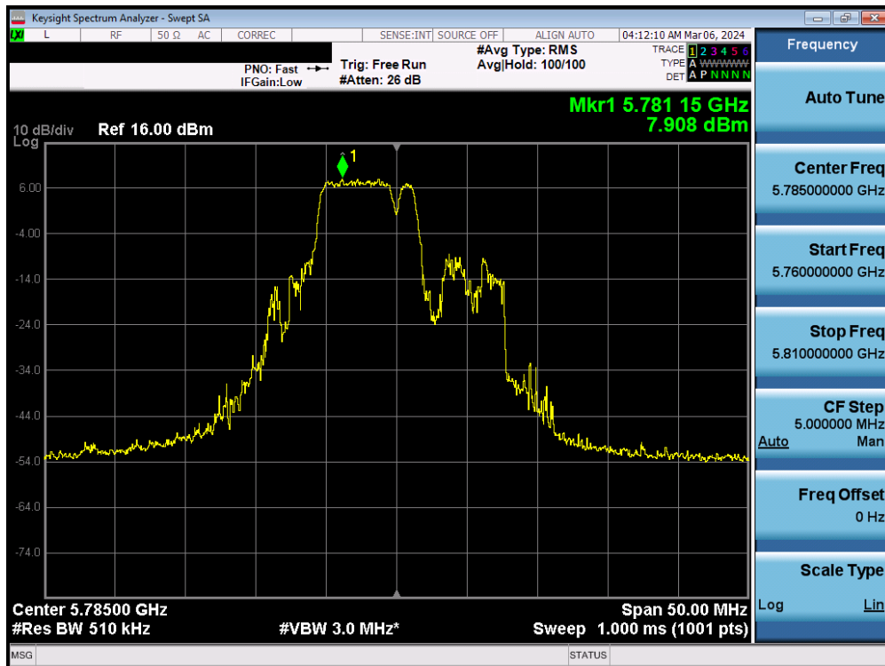
Plot 7-120. Power Spectral Density Plot MIMO ANT1 (20MHz BW 802.11be – 52+26 Tones (UNII Band 3) – Ch. 157)
