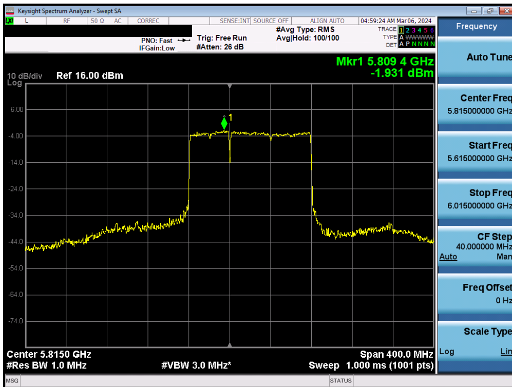
Plot 7-172. Power Spectral Density Plot MIMO ANT1 (160MHz BW 802.11be (UNII Band 3/4) – Ch. 163)
