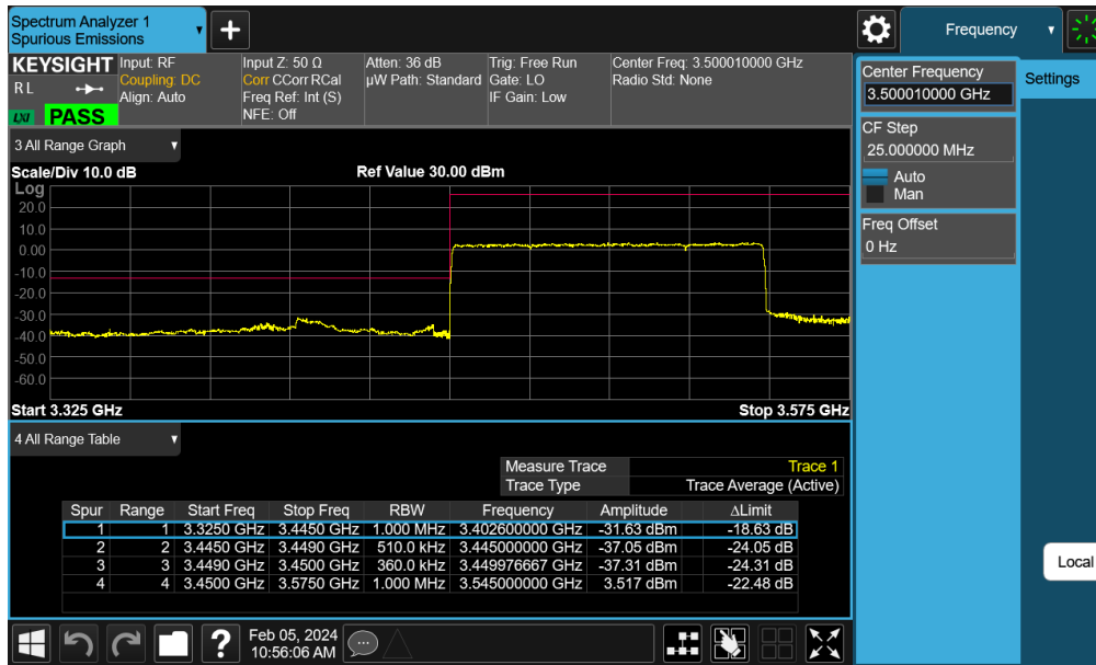
Plot 7-145. Lower ACP Plot (NR Band n77 - 100MHz DFT-s-OFDM-BPSK – Full RB – Ant8)
