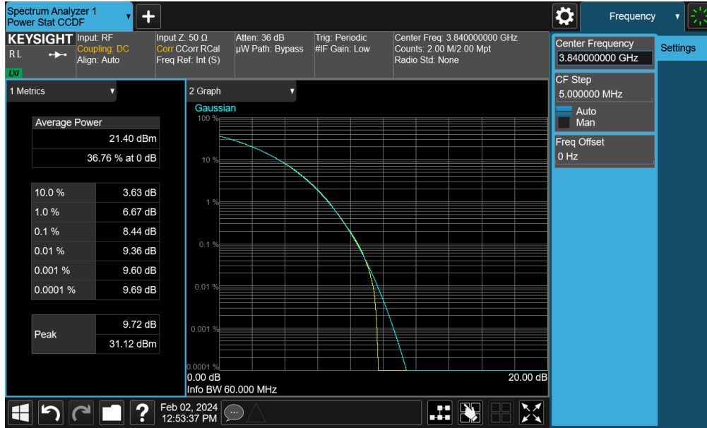
Plot 7-160. PAR Plot (NR Band n77 - 60MHz CP-OFDM-256QAM – Full RB – Ant3)
