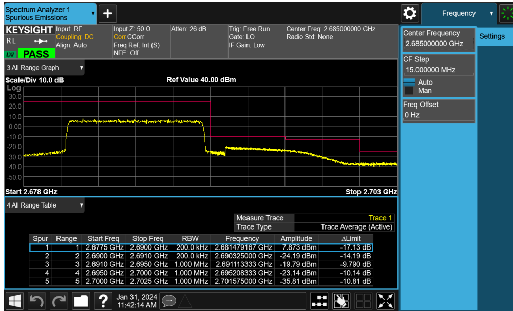
Plot 7-119. Upper ACP Plot (LTE Band 41(PC3) - 10MHz QPSK – Full RB - Ant1)
