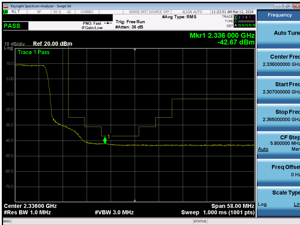
Plot 7-115. Extended Upper Band Edge Plot (LTE Band 30 - 10MHz QPSK – Full RB - Ant1)
