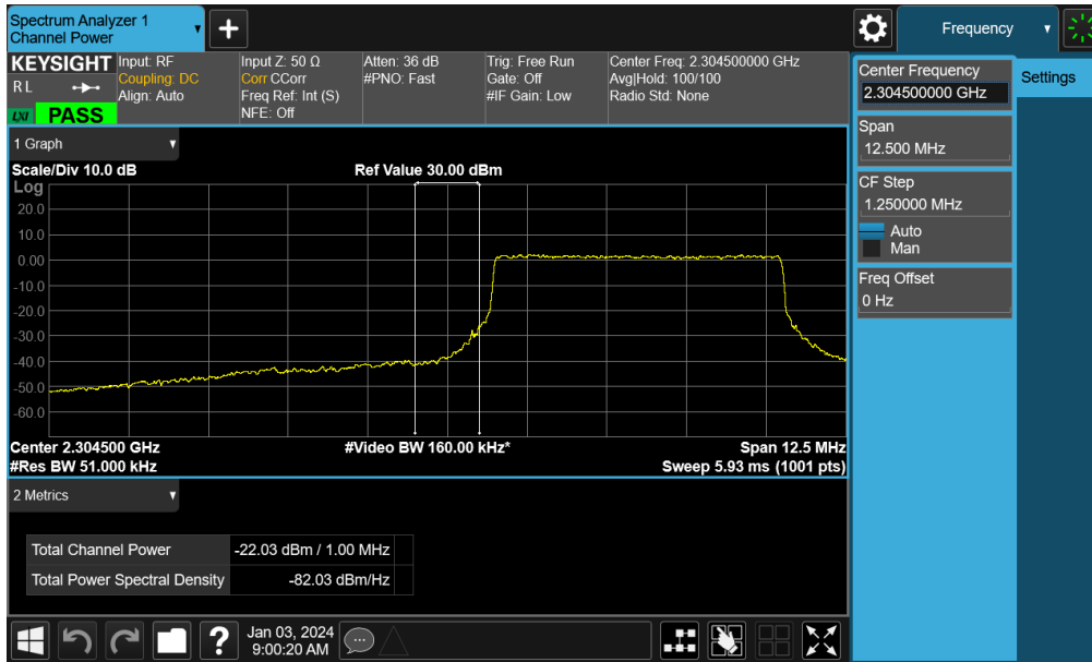
Plot 7-128. Lower Band Edge Plot (NR Band n30 - 5MHz CP-OFDM-QPSK – Full RB - Ant4)
