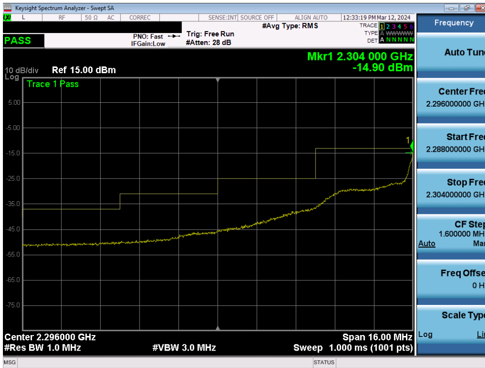
Plot 7-129. Extended Lower Band Edge Plot (NR Band n30 - 5MHz CP-OFDM-QPSK – Full RB - Ant4)
