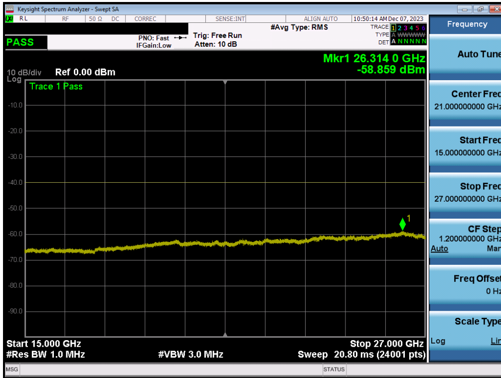
Plot 7-89. Conducted Spurious Plot (LTE Band 30 - 10MHz QPSK - RB Size 1, RB Offset 0 - Ant1)
