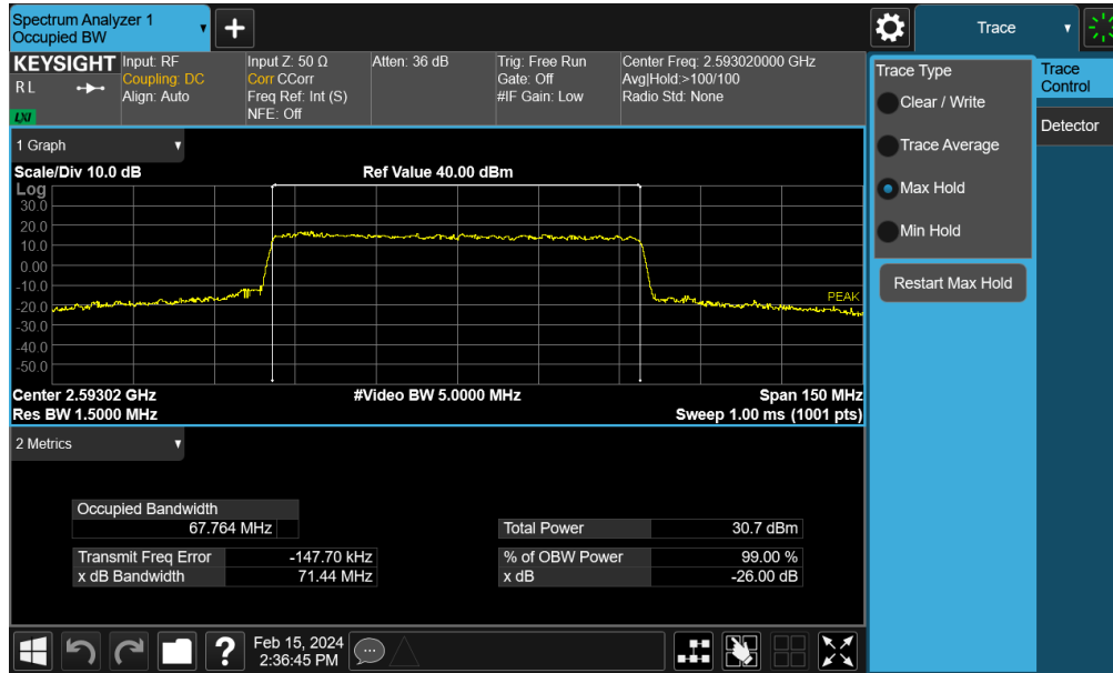
Plot 7-70. Occupied Bandwidth Plot (NR Band n41 - 70MHz QPSK - Full RB - Ant4)
