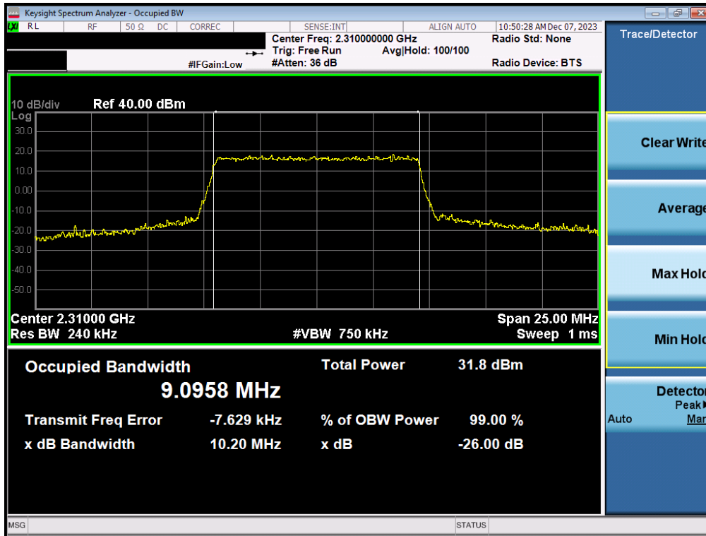
Plot 7-1. Occupied Bandwidth Plot (LTE Band 30 - 10MHz QPSK - Full RB - Ant1 – Ant1)
