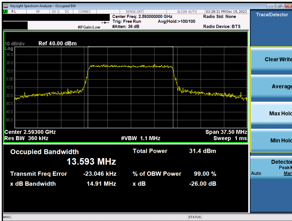
Plot 7-16. Occupied Bandwidth Plot (LTE Band 41(PC3) - 15MHz 16-QAM - Full RB - Ant1)
