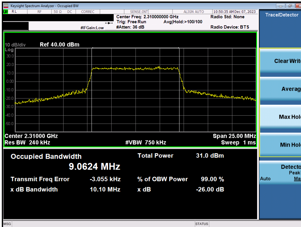
Plot 7-2. Occupied Bandwidth Plot (LTE Band 30 - 10MHz 16-QAM - Full RB - Ant1)
