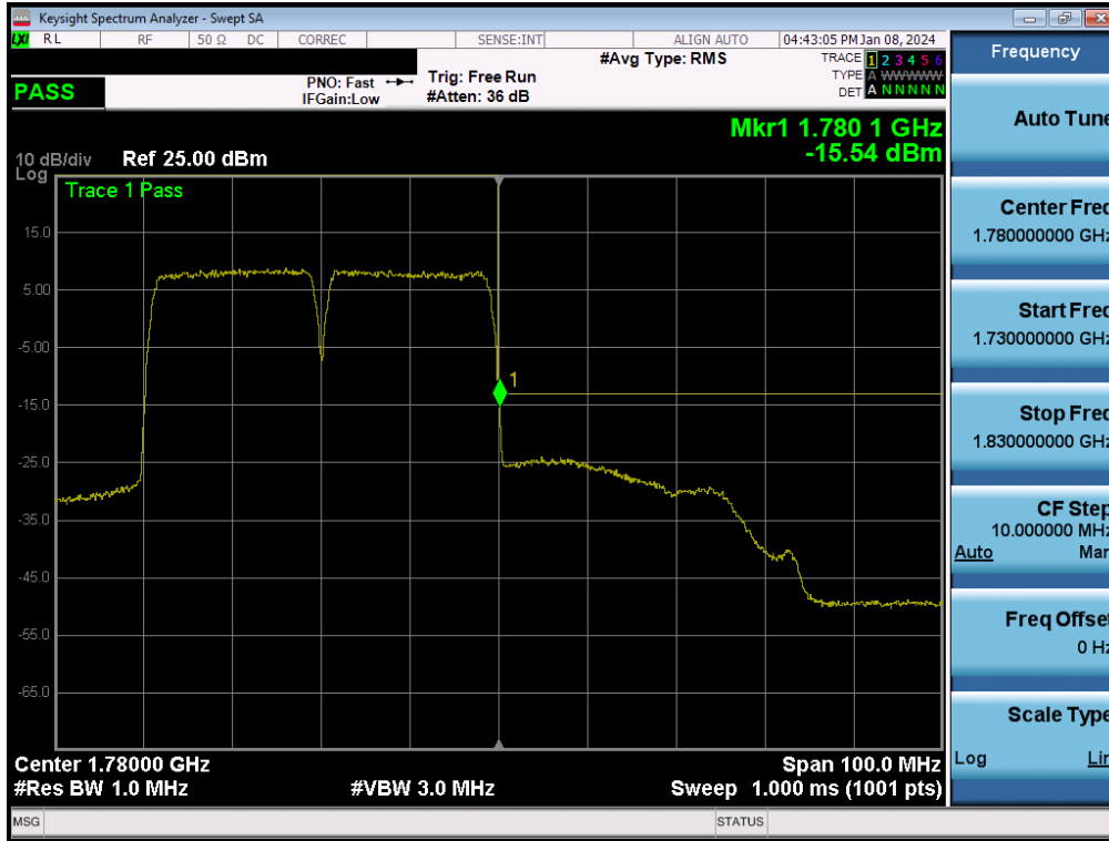
Plot 7-156. Upper Band Edge Plot (ULCA LTE Band 66 – 20+20MHz QPSK – Full RB - Ant1)
