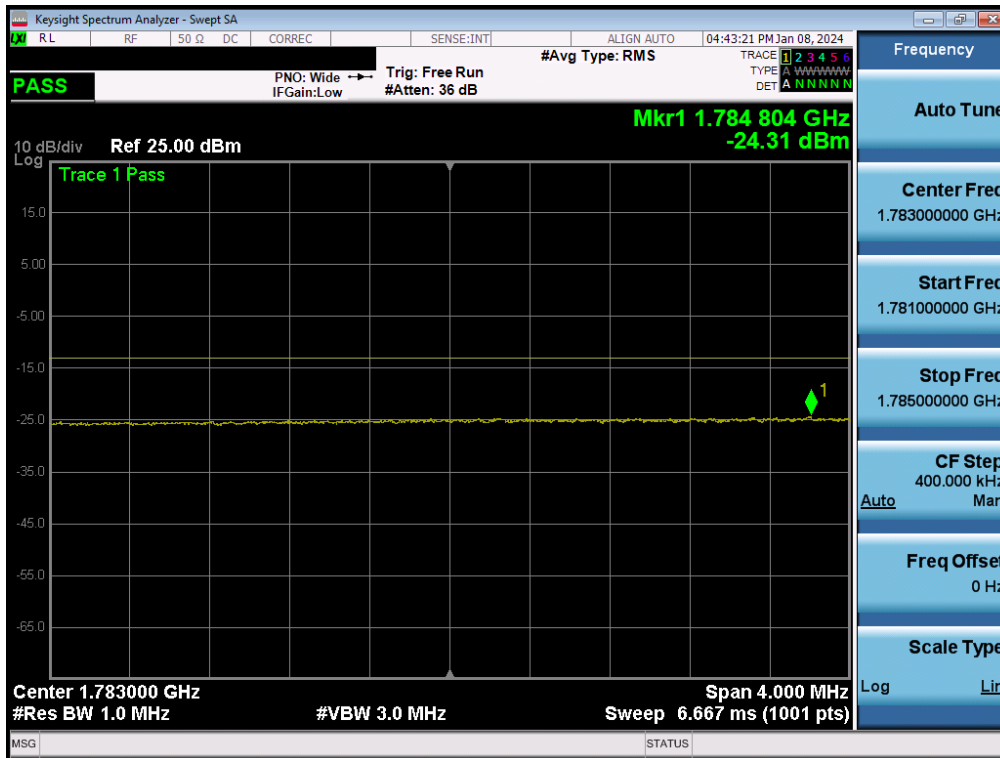
Plot 7-157. Upper Extended Band Edge Plot (ULCA LTE Band 66 – 20+20MHz QPSK – Full RB - Ant1)
