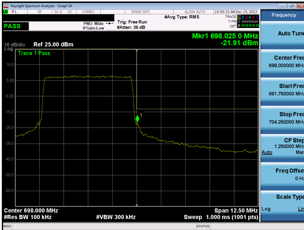
Plot 7-129. Upper Band Edge Plot (LTE Band 71 - 5MHz QPSK – Full RB - Ant4)
