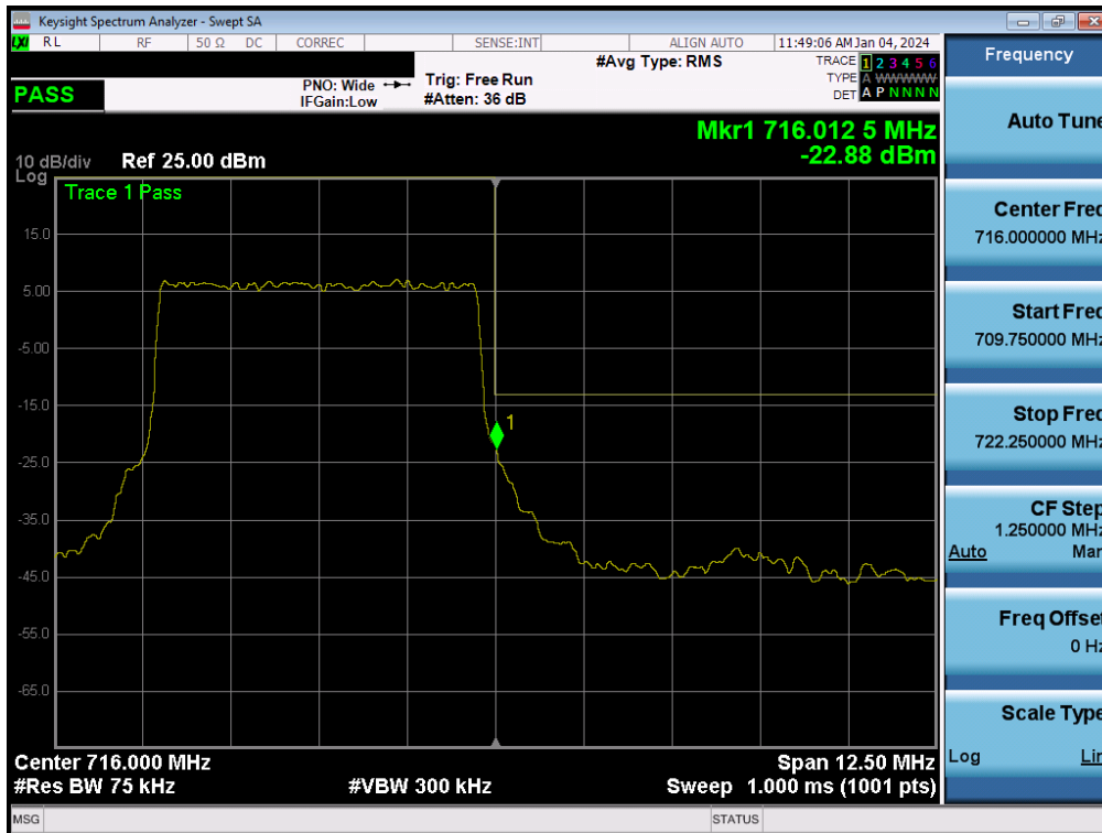
Plot 7-139. Upper Band Edge Plot (NR Band n12 – 5.0MHz - Full RB - Ant4)
