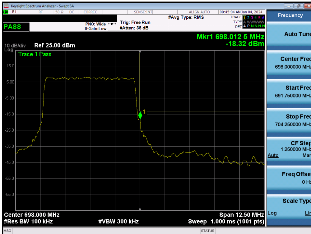
Plot 7-137. Upper Band Edge Plot (NR Band n71 – 5.0MHz - Full RB - Ant4)
