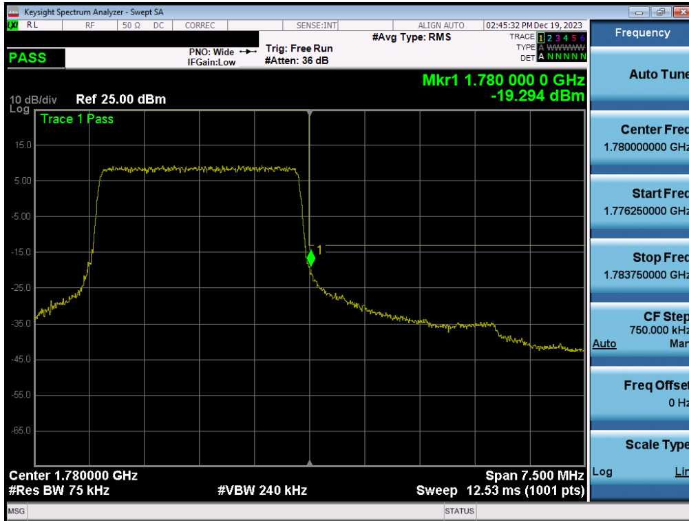
Plot 7-148. Upper Band Edge Plot (LTE Band 66 - 3MHz QPSK – Full RB - Ant1)
