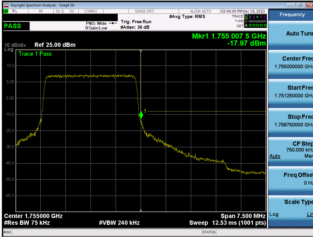
Plot 7-146. Upper Band Edge Plot (LTE Band 4 - 3MHz QPSK – Full RB - Ant1)
