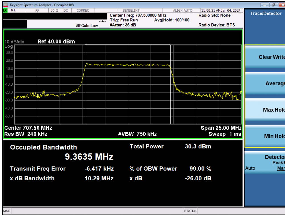
Plot 7-37. Occupied Bandwidth Plot (NR Band n12 - 10MHz CP-OFDM QPSK - Full RB - Ant4)
