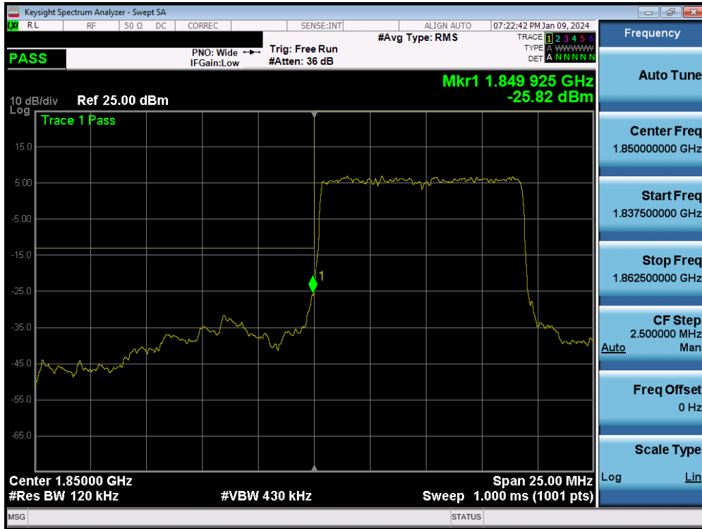
Plot 7-82. Lower Band Edge Plot (NR Band n25/2 - 10MHz QPSK – Full RB – Ant1)
