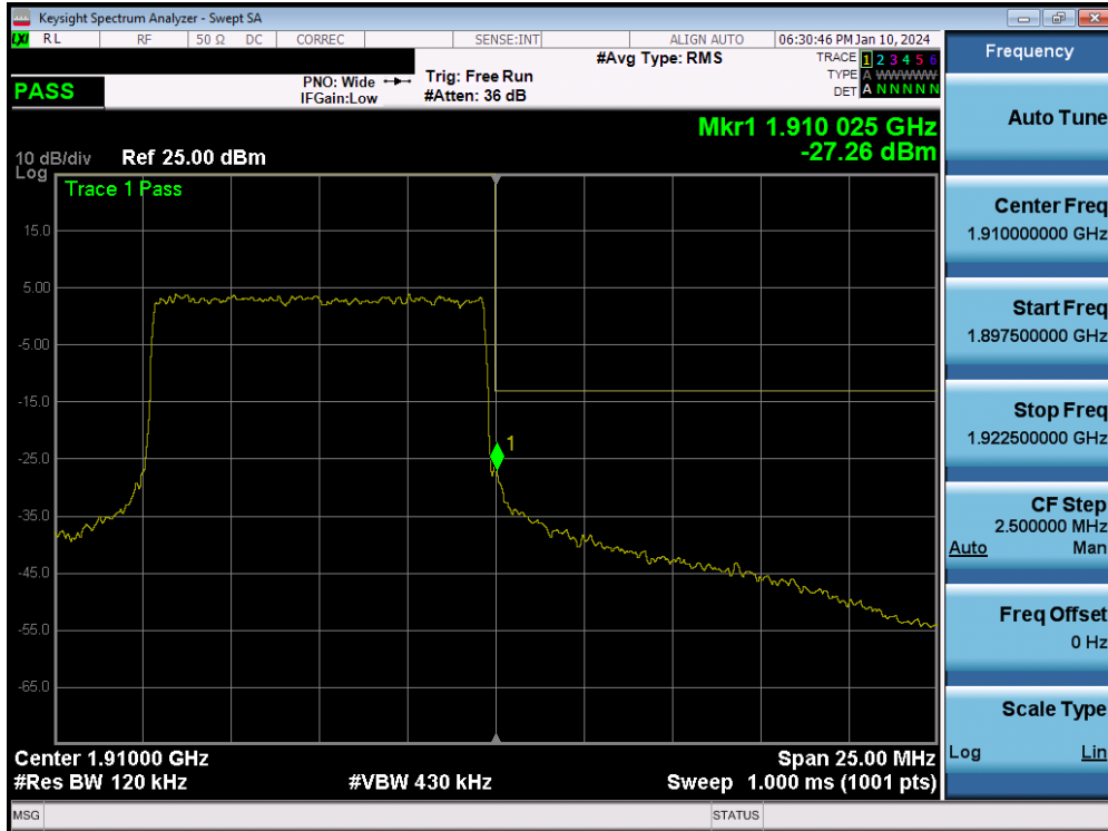
Plot 7-84. Upper Band Edge Plot (NR Band n2 - 10MHz QPSK – Full RB – Ant1)
