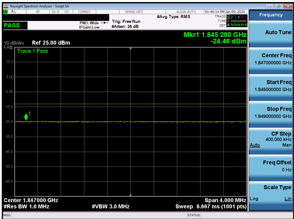
Plot 7-79. Extended Lower Band Edge Plot (ULCA LTE Band 2 – 20+20MHz QPSK – Full RB – Ant1)
