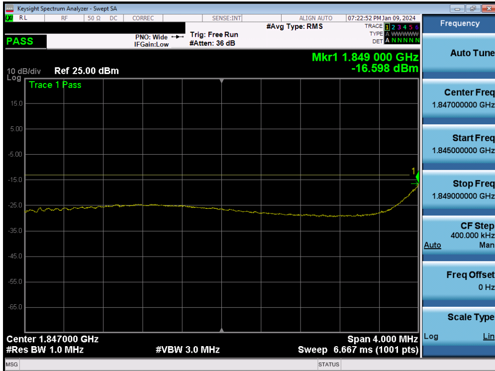
Plot 7-83. Extended Lower Band Edge Plot (NR Band n25/2 - 10MHz QPSK – Full RB – Ant1)
