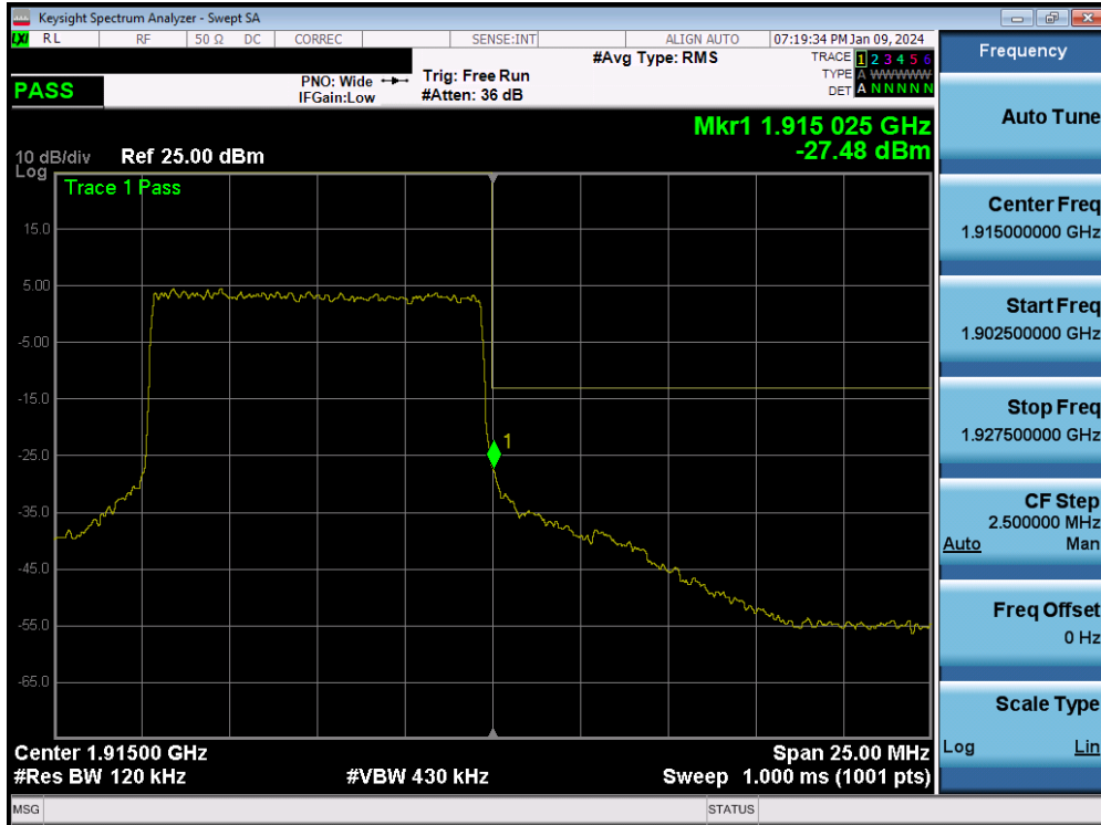
Plot 7-86. Upper Band Edge Plot (NR Band n25 - 10MHz QPSK – Full RB – Ant1)
