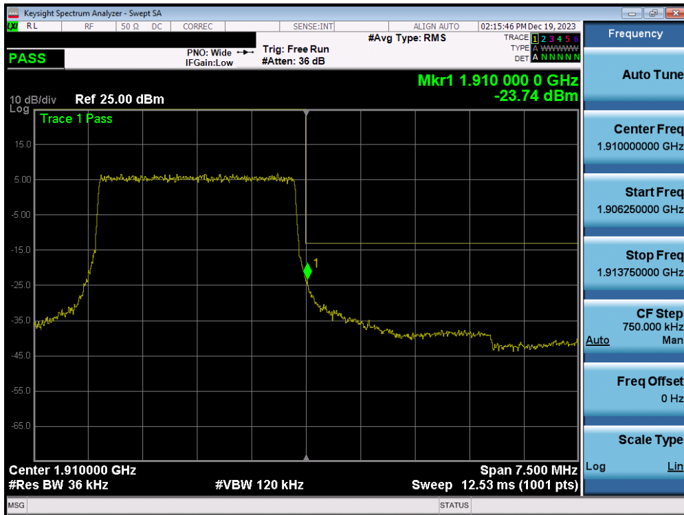
Plot 7-74. Upper Band Edge Plot (LTE Band 2 - 3MHz QPSK – Full RB – Ant1)
