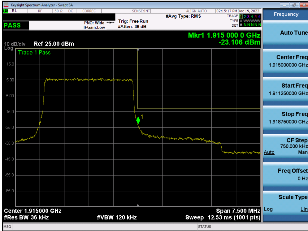
Plot 7-76. Upper Band Edge Plot (LTE Band 25 - 3MHz QPSK – Full RB – Ant1)
