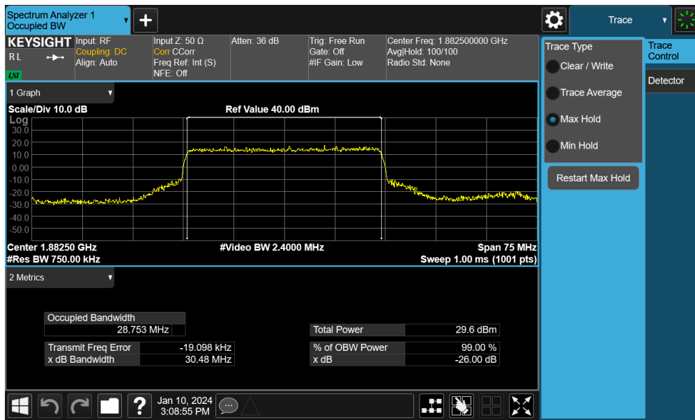
Plot 7-39. Occupied Bandwidth Plot (NR Band n25 - 30.0MHz CP-OFDM 16QAM - Full RB – Ant4)
