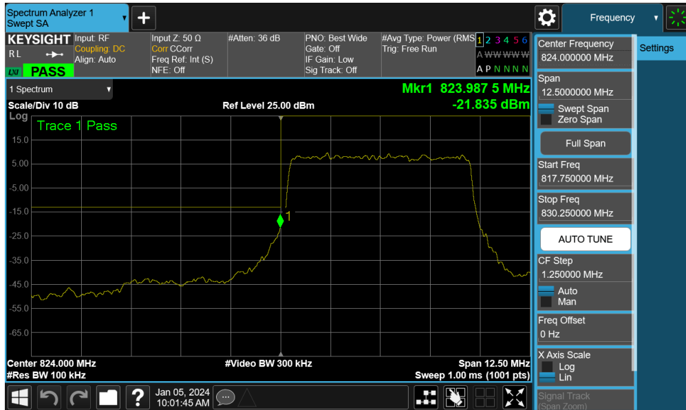
Plot 7-41. Lower Band Edge Plot (NR Band n26/5 – 5.0MHz - Full RB - Ant4)
