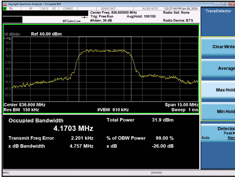
Plot 7-23. Occupied Bandwidth Plot (WCDMA, Ch. 4183 – Ant4)
