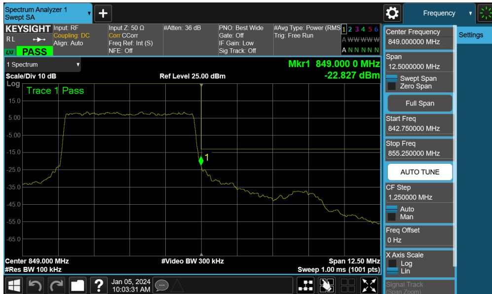
Plot 7-42. Upper Band Edge Plot (NR Band n26/5 – 5.0MHz - Full RB - Ant4)
