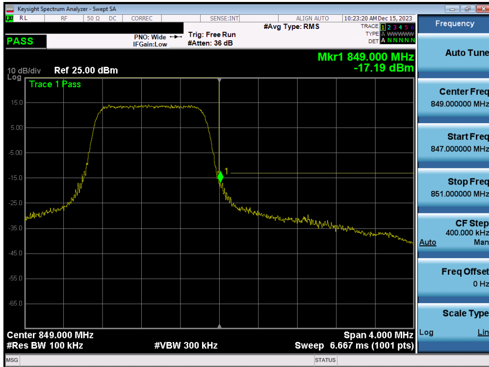
Plot 7-38. Upper Band Edge Plot (LTE Band 26/5 – 1.4MHz QPSK – Full RB - Ant4)
