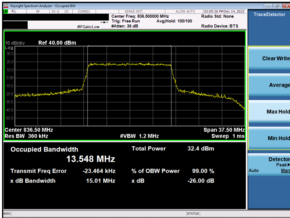
Plot 7-1. Occupied Bandwidth Plot (LTE Band 26 - 15MHz QPSK - Full RB - Ant4)
