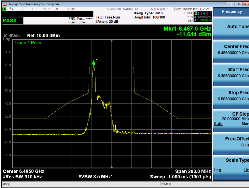
Plot 7-314. In-Band Emission Plot MIMO ANT2 (40MHz BW 802.11be (26 Tones) (UNII Band 6) – Ch. 107) - LPI
