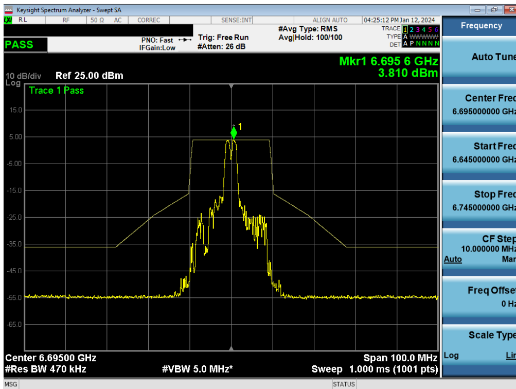
Plot 7-290. In-Band Emission Plot MIMO ANT1 (20MHz BW 802.11be (26 Tone) (UNII Band 7) – Ch. 149) – SP
