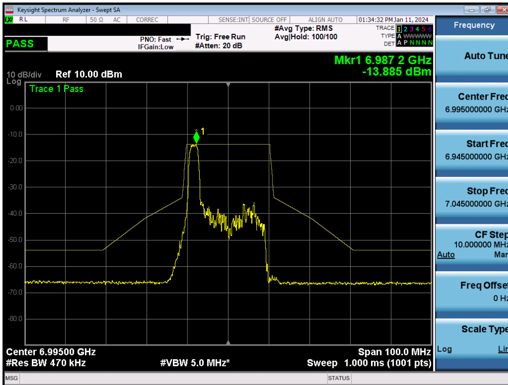
Plot 7-323. In-Band Emission Plot MIMO ANT2 (20MHz BW 802.11be (26 Tones) (UNII Band 8) – Ch. 209) - LPI
