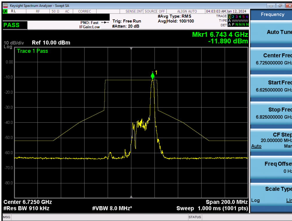
Plot 7-319. In-Band Emission Plot MIMO ANT2 (40MHz BW 802.11be (26 Tones) (UNII Band 7) – Ch. 155) - LPI
