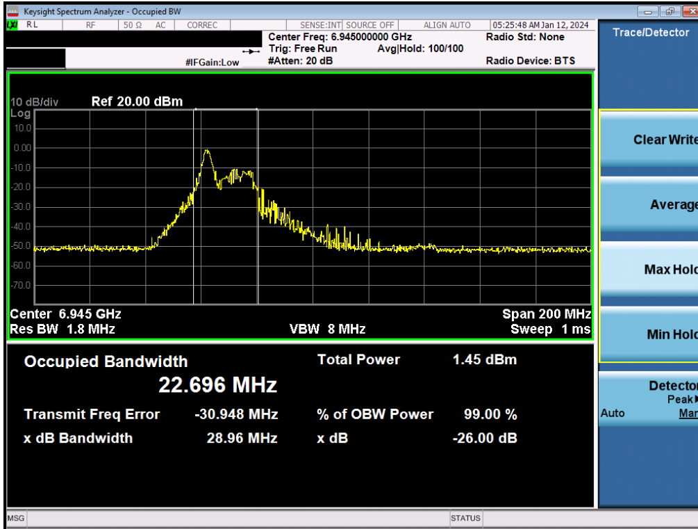
Plot 7-60. Occupied Bandwidth Plot MIMO ANT2 (80MHz BW 802. 11be (26 Tones) (UNII Band 8) – Ch. 199)
