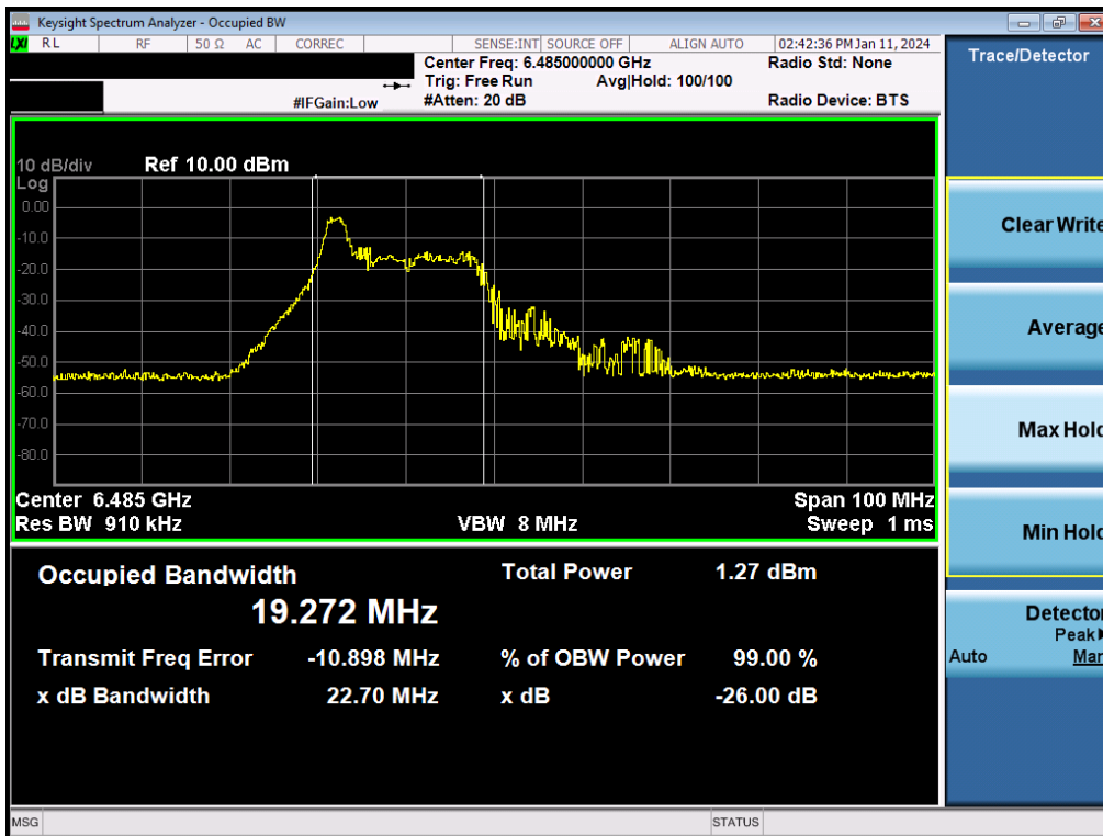
Plot 7-49. Occupied Bandwidth Plot MIMO ANT2 (40MHz BW 802. 11be (26 Tones) (UNII Band 6) – Ch. 107)
