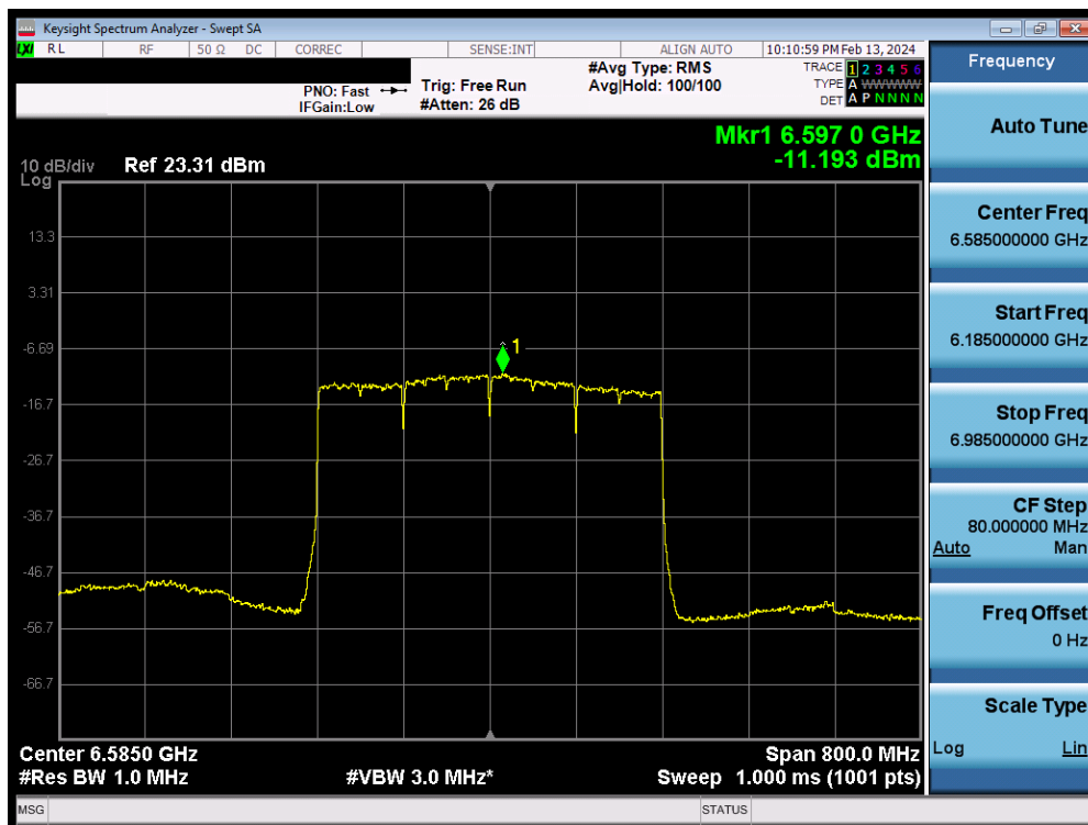
Plot 7-109. Power Spectral Density MIMO ANT2 (320MHz 802.11ax/be (UNII Band 6/7) – Ch. 127) - LPI
