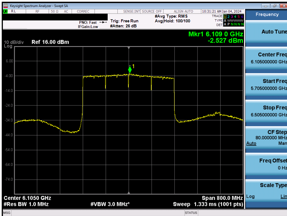
Plot 7-97. Power Spectral Density MIMO ANT2 (320MHz 802.11ax/be (UNII Band 5) – Ch.31) - SP
