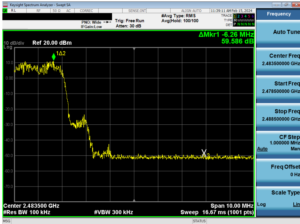
Plot 7-126. Band Edge Plot (Bluetooth with Hopping Enabled, 3 Mbps)
