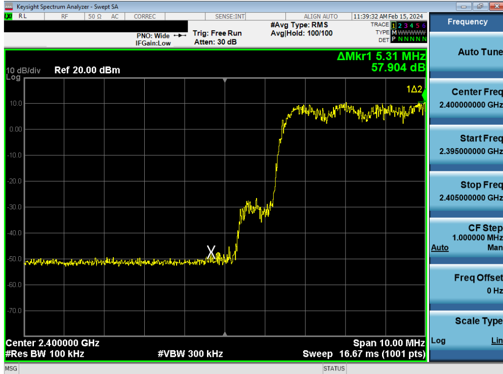
Plot 7-125. Band Edge Plot (Bluetooth with Hopping Enabled, 3 Mbps)
