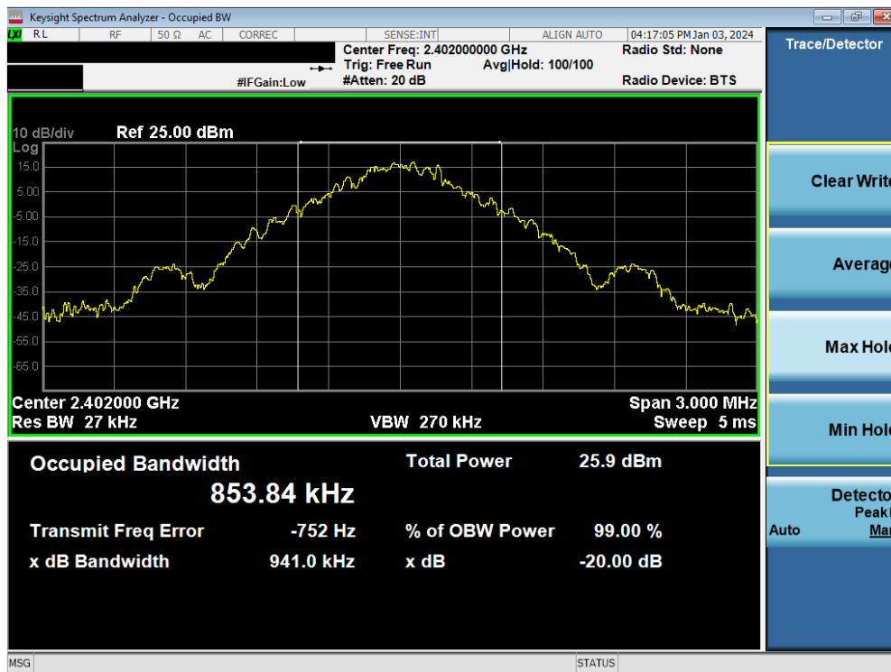
Plot 7-12. 20dB Bandwidth Plot (Bluetooth, 1Mbps – Ch. 0)
