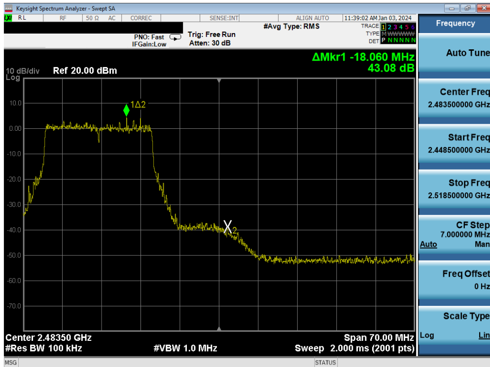
Plot 7-122. Band Edge Plot MIMO ANT2 (802.11be (2.4GHz) – Ch. 11)
