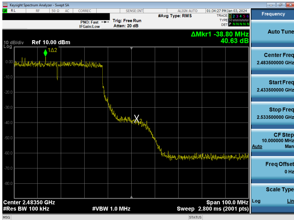
Plot 7-146. Band Edge Plot MIMO ANT2 (802.11be (2.4GHz) – Ch. 9)
