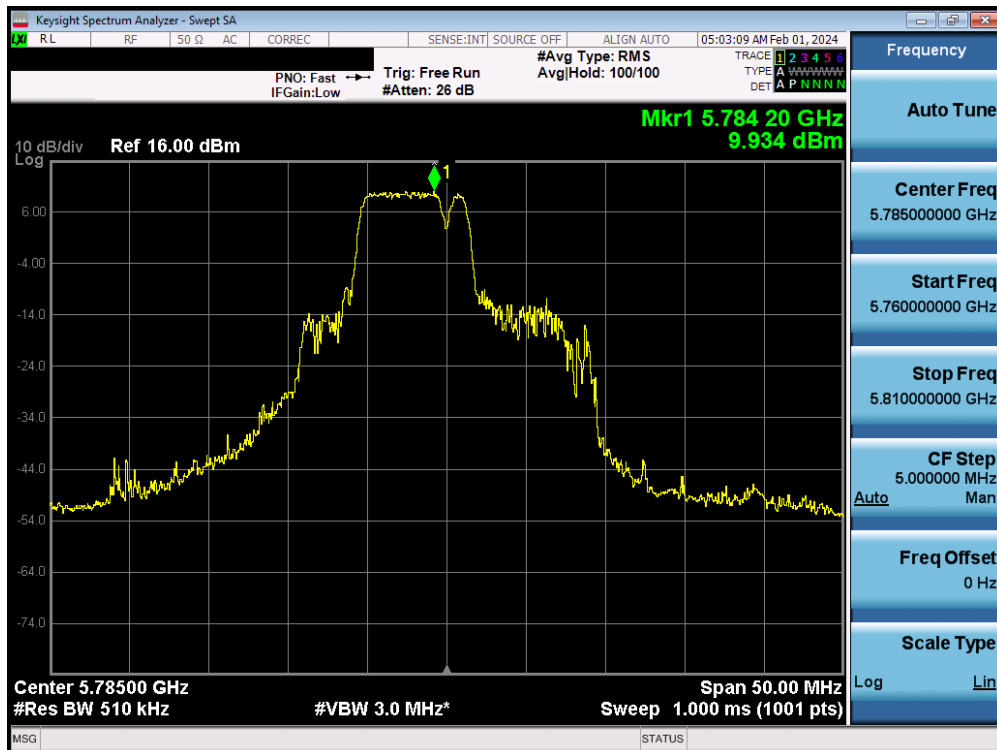
Plot 7-176. Power Spectral Density Plot MIMO ANT2 (20MHz BW 802.11be – 52+26 Tones (UNII Band 3) – Ch. 157)
