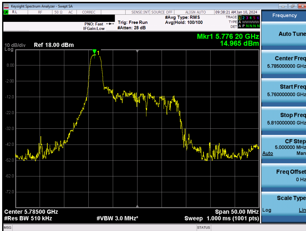
Plot 7-140. Power Spectral Density Plot MIMO ANT2 (20MHz BW 802.11be – 26 Tones (UNII Band 3) – Ch. 157)
