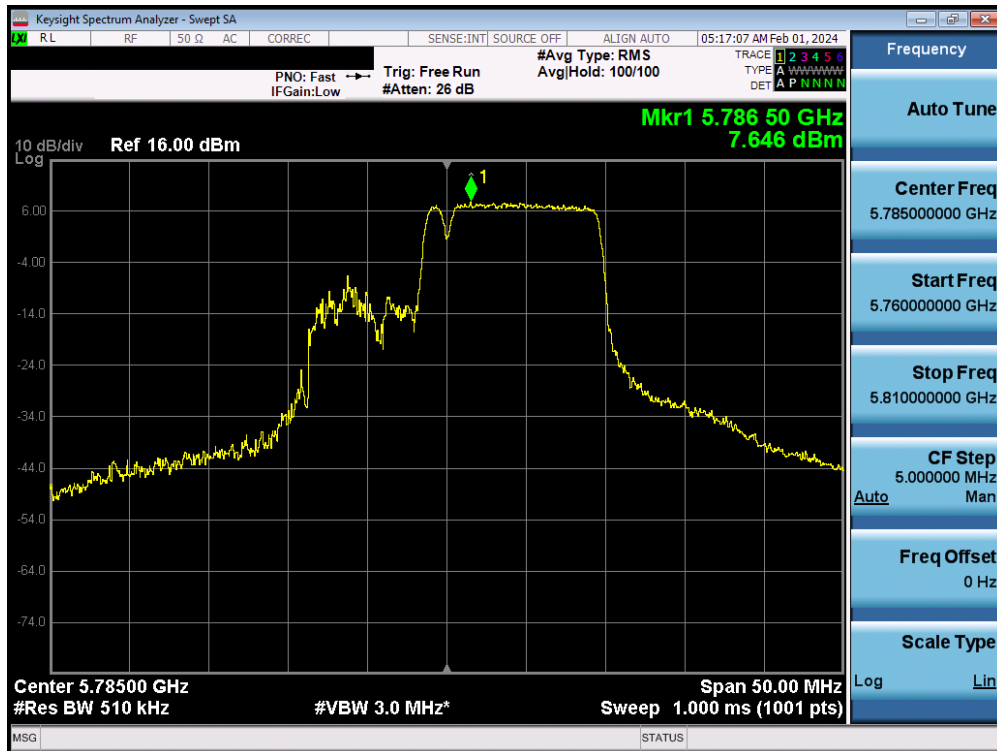
Plot 7-177. Power Spectral Density Plot MIMO ANT2 (20MHz BW 802.11be – 106+26 Tones (UNII Band 3) – Ch. 157)
