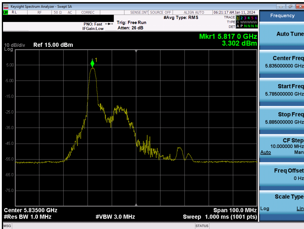
Plot 7-144. Power Spectral Density Plot MIMO ANT2 (40MHz BW 802.11be – 26 Tones (UNII Band 3/4) – Ch. 167)
