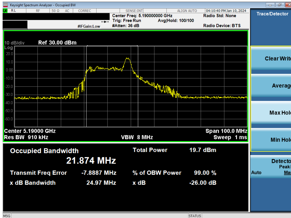
Plot 7-4. 26dB Bandwidth Plot MIMO ANT1 (40MHz BW 802.11be – 26 Tones (UNII Band 1) – Ch. 38)
