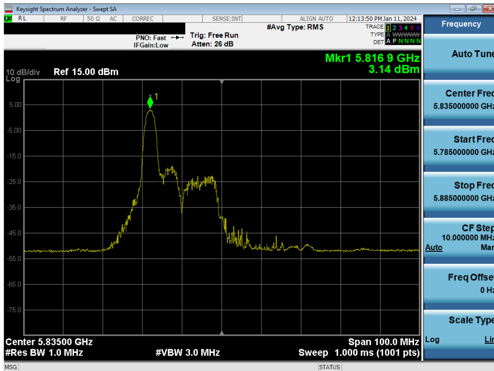
Plot 7-90. Power Spectral Density Plot MIMO ANT1 (40MHz BW 802.11be – 26 Tones (UNII Band 3/4) – Ch. 167)
