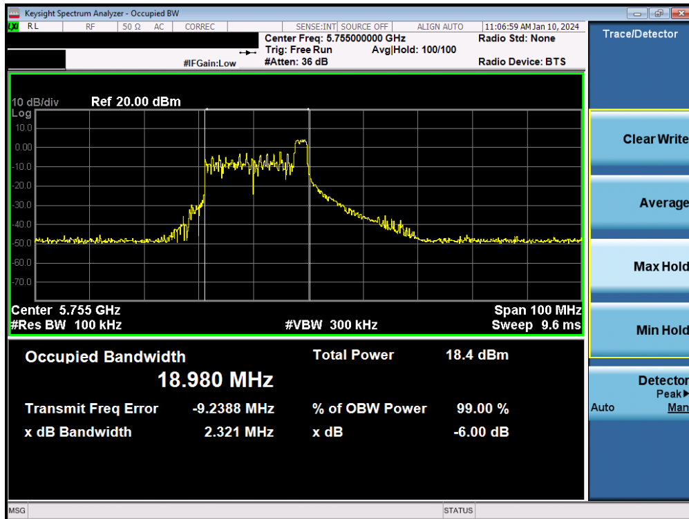
Plot 7-62. 6dB Bandwidth Plot MIMO ANT2 (40MHz BW 802.11be – 26 Tones (UNII Band 3) – Ch. 151)
