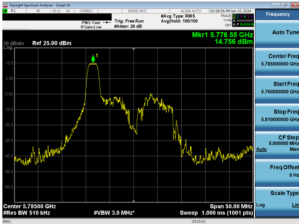
Plot 7-86. Power Spectral Density Plot MIMO ANT1 (20MHz BW 802.11be – 26 Tones (UNII Band 3) – Ch. 157)
