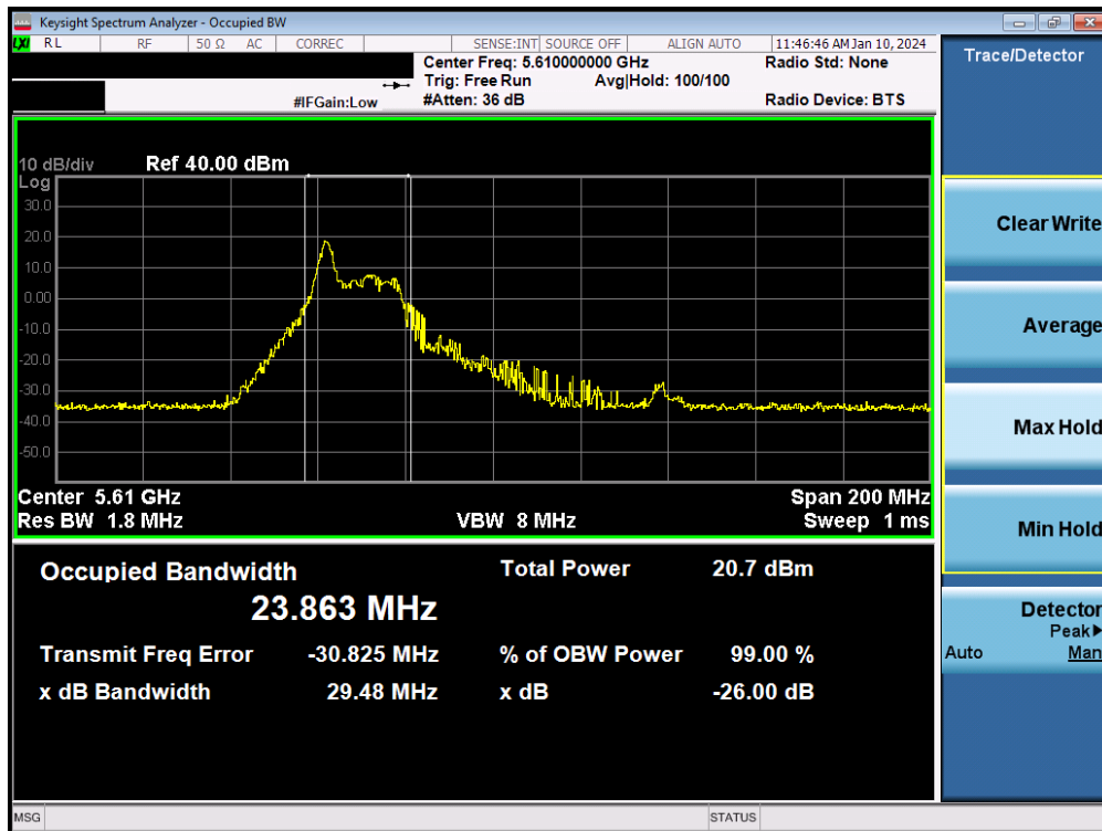
Plot 7-34. 26dB Bandwidth Plot MIMO ANT2 (80MHz BW 802.11be – 26 Tones (UNII Band 2C) – Ch. 122)
