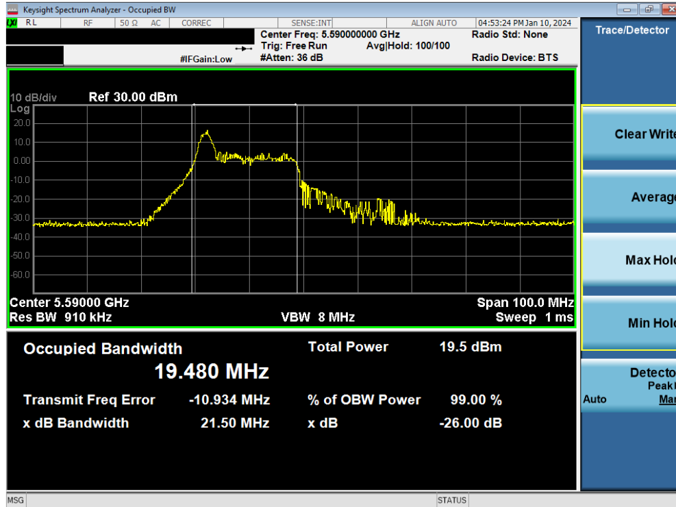
Plot 7-11. 26dB Bandwidth Plot MIMO ANT1 (40MHz BW 802.11be – 26 Tones (UNII Band 2C) – Ch. 118)
