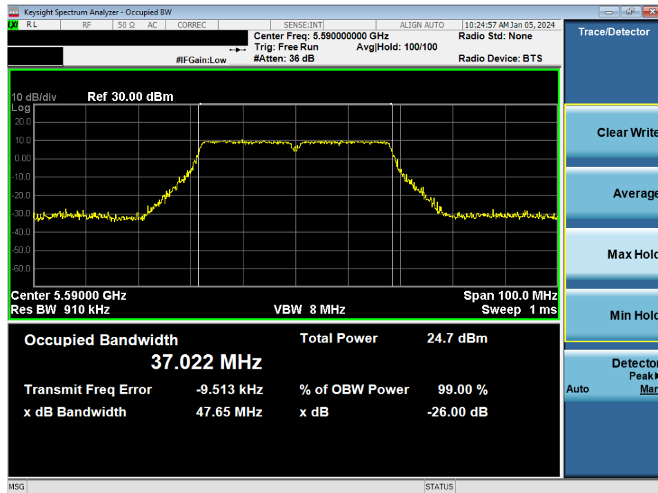
Plot 7-22. 26dB Bandwidth Plot MIMO ANT1 (40MHz BW 802.11n (UNII Band 2C) – Ch. 118)
