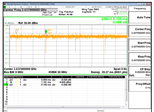
DUTY CYCLE 802.11be EHT20 52T MODE, 2TX
