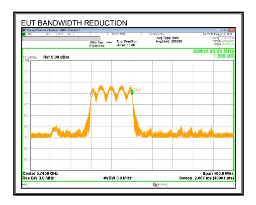
With the Incumbent Signal set to the Lower Edge  $f_{c2}$  the EUT continues to operate at a reduced 80MHz bandwidth.
