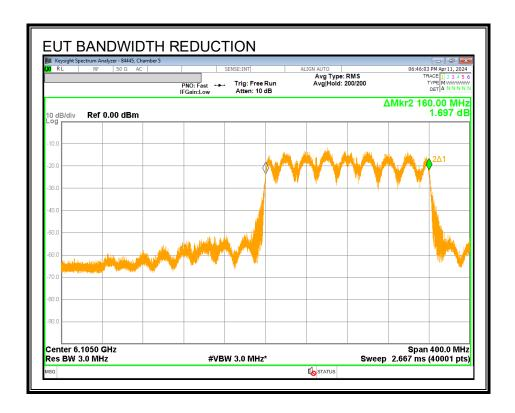
With the Incumbent Signal set to the Lower Edge  $f_{c2}$  the EUT continues to operate at a reduced 160MHz bandwidth.
