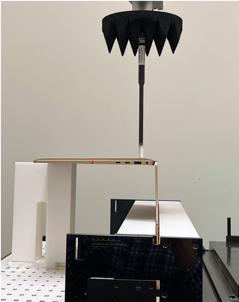
Note: Protrusions (rubber feet) were removed during scan to avoid collision with probe
