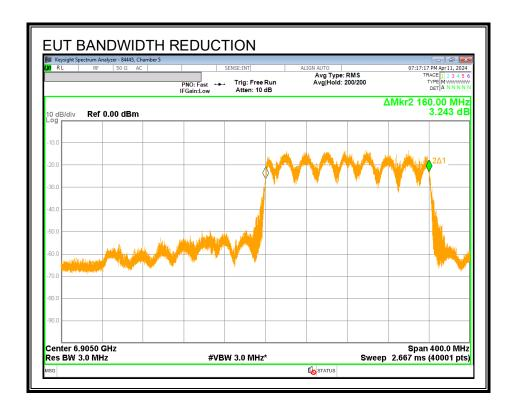
With the Incumbent Signal set to the Lower Edge  $f_{c2}$  the EUT continues to operate at a reduced 160MHz bandwidth.
