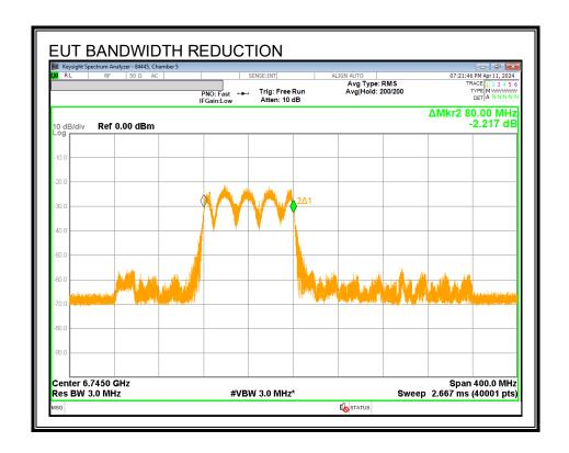
With the Incumbent Signal set to the Lower Edge  $f_{c2}$  the EUT continues to operate at a reduced 80MHz bandwidth.
