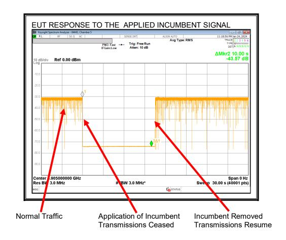
Transmissions cease while the Incumbent AWGN Signal is present and resume after it is removed.
