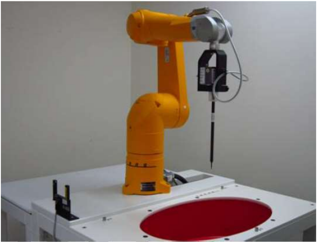
Fig.1 Photograph of the SAR measurement system
