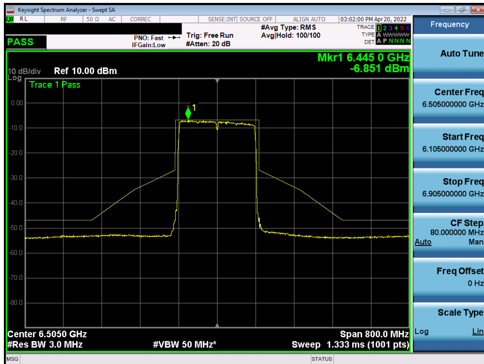
Plot 7-940. In-Band Emission Plot MIMO ANT2 (160MHz BW 802.11ax (Full Tone) (UNII Band 6) – Ch. 111)
