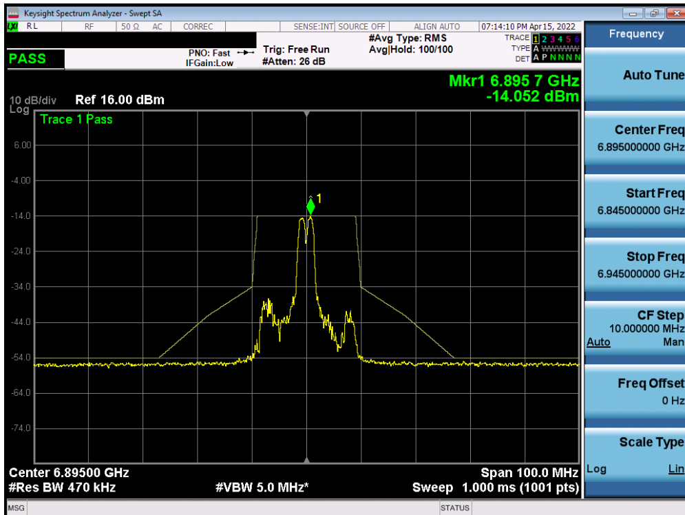
Plot 7-912. In-Band Emission Plot MIMO ANT2 (20MHz BW 802.11ax (26 Tones) (UNII Band 8) – Ch. 189)
