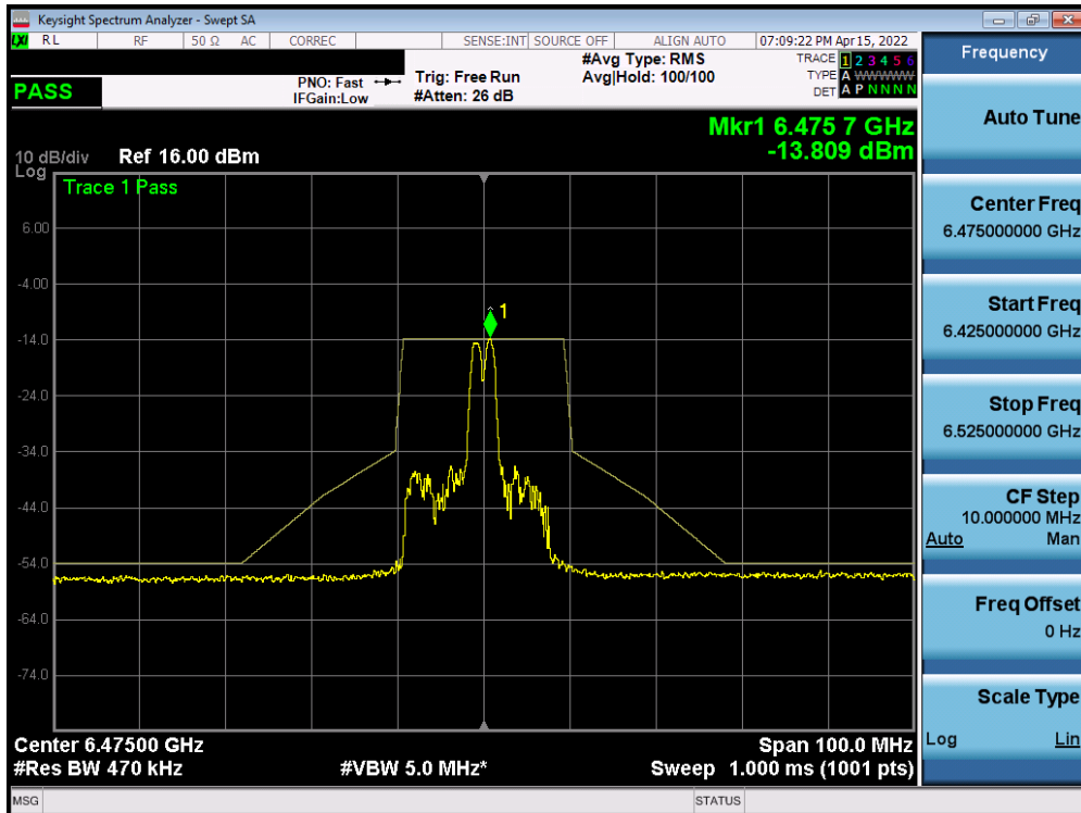
Plot 7-894. In-Band Emission Plot MIMO ANT2 (20MHz BW 802.11ax (26 Tones) (UNII Band 6) – Ch. 105)
