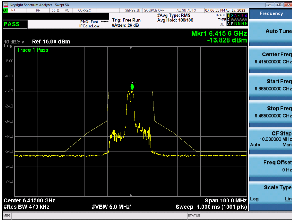
Plot 7-883. In-Band Emission Plot MIMO ANT2 (20MHz BW 802.11ax (26 Tones) UNII Band 5) – Ch. 93)
