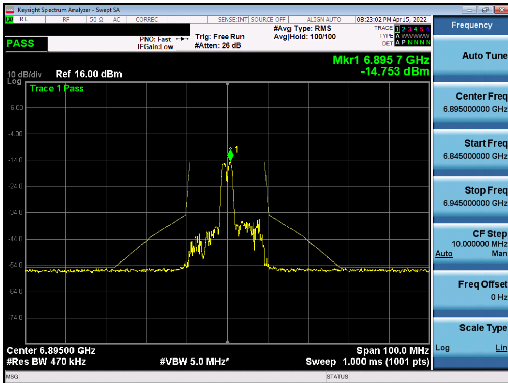
Plot 7-832. In-Band Emission Plot MIMO ANT1 (20MHz BW 802.11ax (26 Tones) (UNII Band 8) – Ch. 189)
