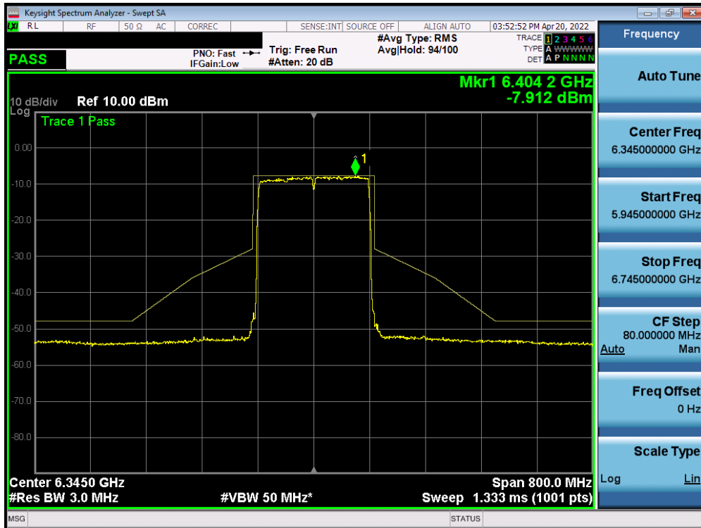
Plot 7-852. In-Band Emission Plot MIMO ANT1 (160MHz BW 1602.11ax (Full Tone) (UNII Band 5) – Ch. 79)
