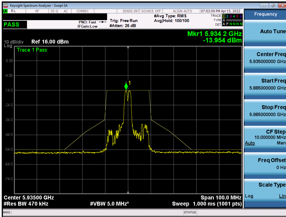
Plot 7-881. In-Band Emission Plot MIMO ANT2 (20MHz BW 802.11ax (26 Tones) UNII Band 5) – Ch. 2
