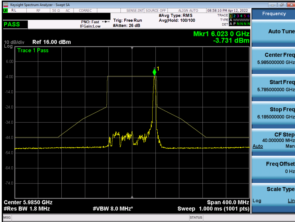
Plot 7-727. In-Band Emission Plot SISO ANT2 (80MHz BW 802.11ax (26 Tones) (UNII Band 5) – Ch. 7)
