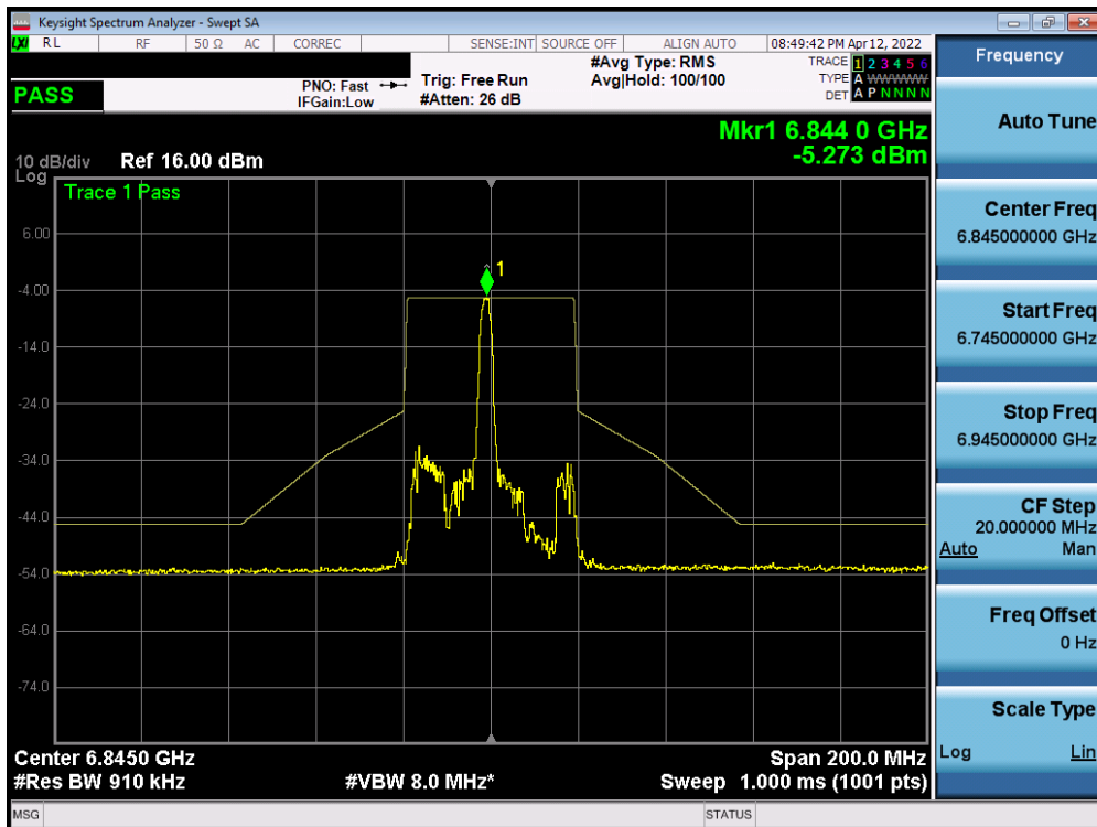
Plot 7-746. In-Band Emission Plot SISO ANT2 (40MHz BW 802.11ax (26 Tones) (UNII Band 7) – Ch. 179)
