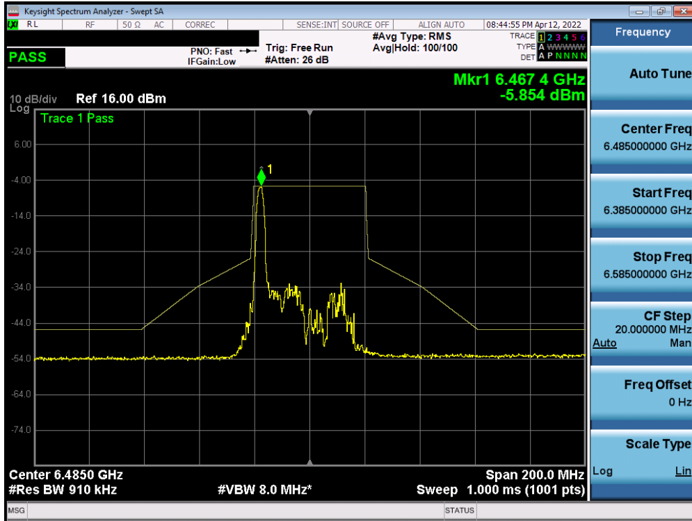
Plot 7-737. In-Band Emission Plot SISO ANT2 (40MHz BW 802.11ax (26 Tones) (UNII Band 6) – Ch. 107)
