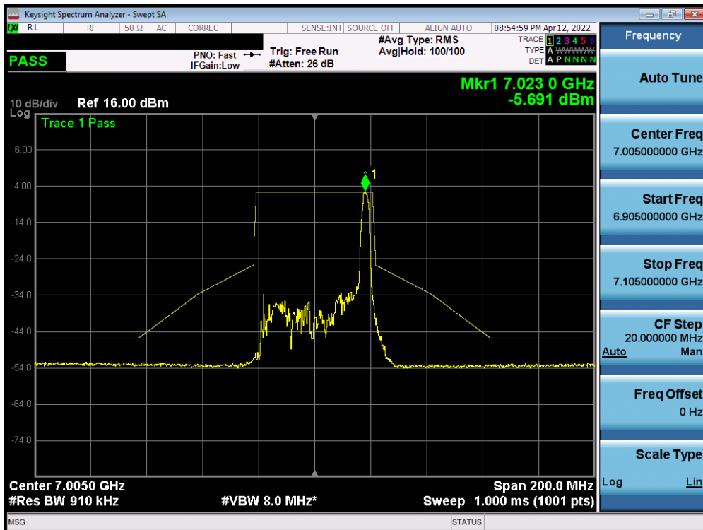
Plot 7-756. In-Band Emission Plot SISO ANT2 (40MHz BW 802.11ax (26 Tones) (UNII Band 8) – Ch. 211)
