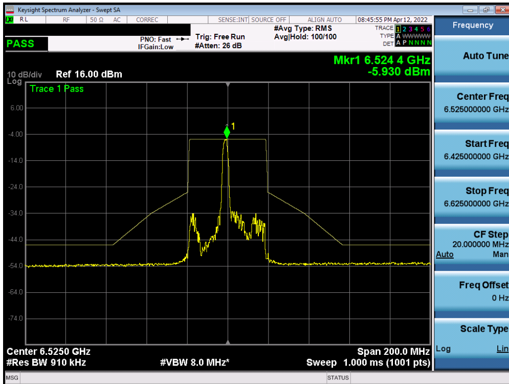
Plot 7-738. In-Band Emission Plot SISO ANT2 (40MHz BW 802.11ax (26 Tones) (UNII Band 6) – Ch. 115)
