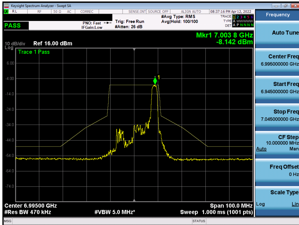
Plot 7-753. In-Band Emission Plot SISO ANT2 (20MHz BW 802.11ax (26 Tones) (UNII Band 8) – Ch. 209)
