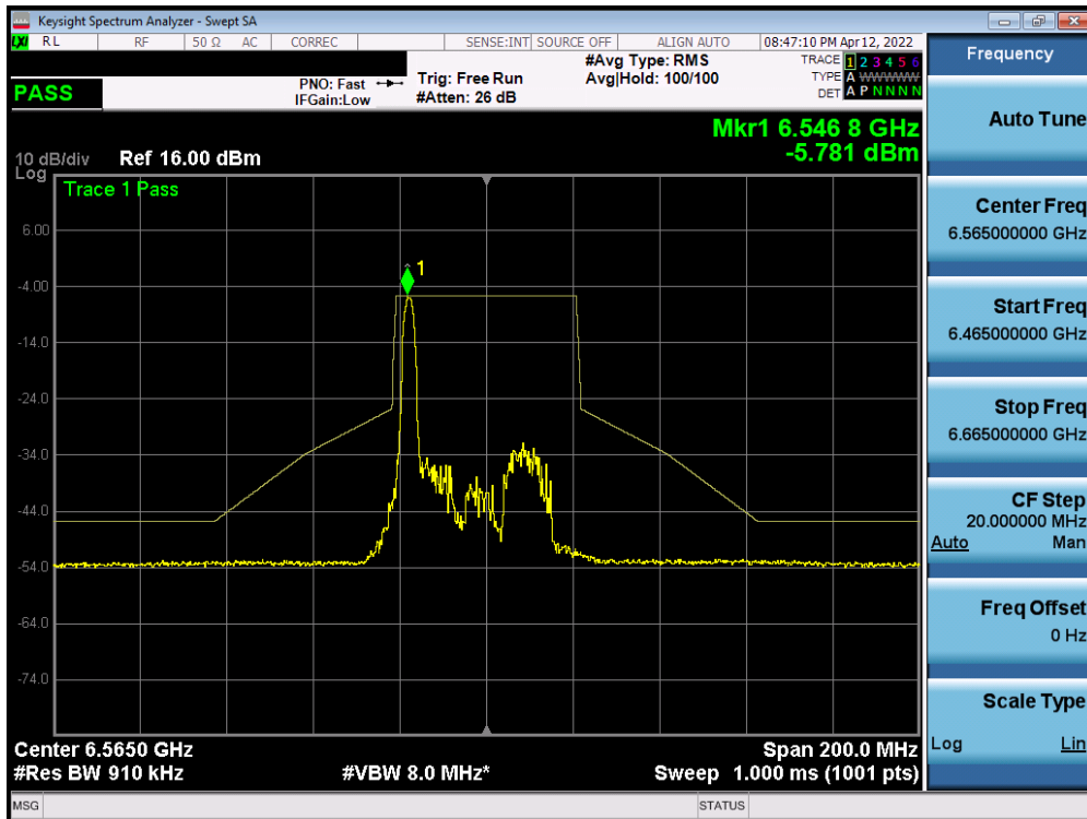
Plot 7-744. In-Band Emission Plot SISO ANT2 (40MHz BW 802.11ax (26 Tones) (UNII Band 7) – Ch. 123)
