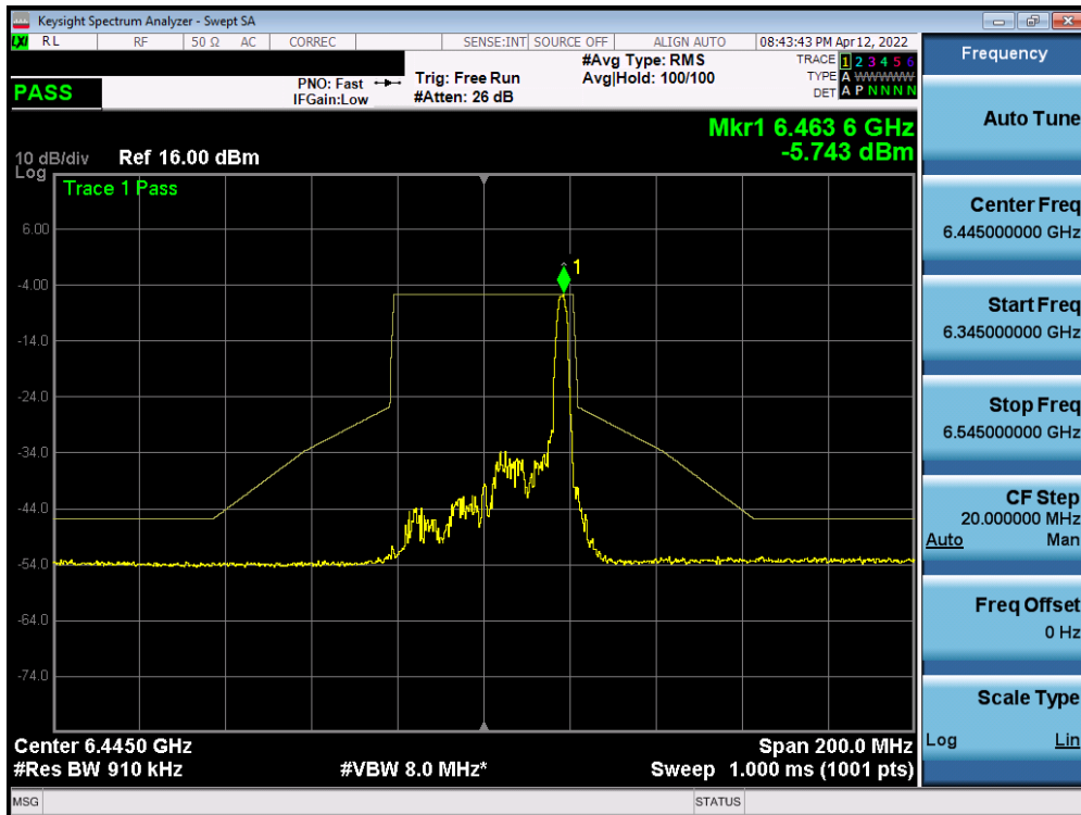
Plot 7-736. In-Band Emission Plot SISO ANT2 (40MHz BW 802.11ax (26 Tones) (UNII Band 6) – Ch. 99)
