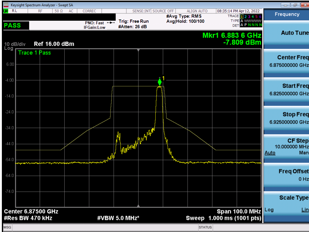
Plot 7-743. In-Band Emission Plot SISO ANT2 (20MHz BW 802.11ax (26 Tones) (UNII Band 7) – Ch. 185)
