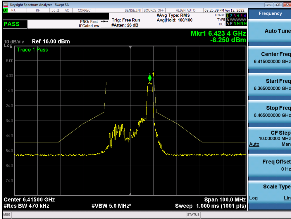
Plot 7-723. In-Band Emission Plot SISO ANT2 (20MHz BW 802.11ax (26 Tones) UNII Band 5) – Ch. 93)
