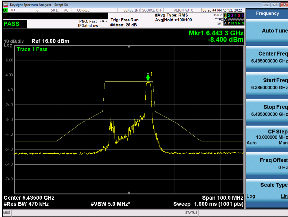
Plot 7-733. In-Band Emission Plot SISO ANT2 (20MHz BW 802.11ax (26 Tones) (UNII Band 6) – Ch. 97)
