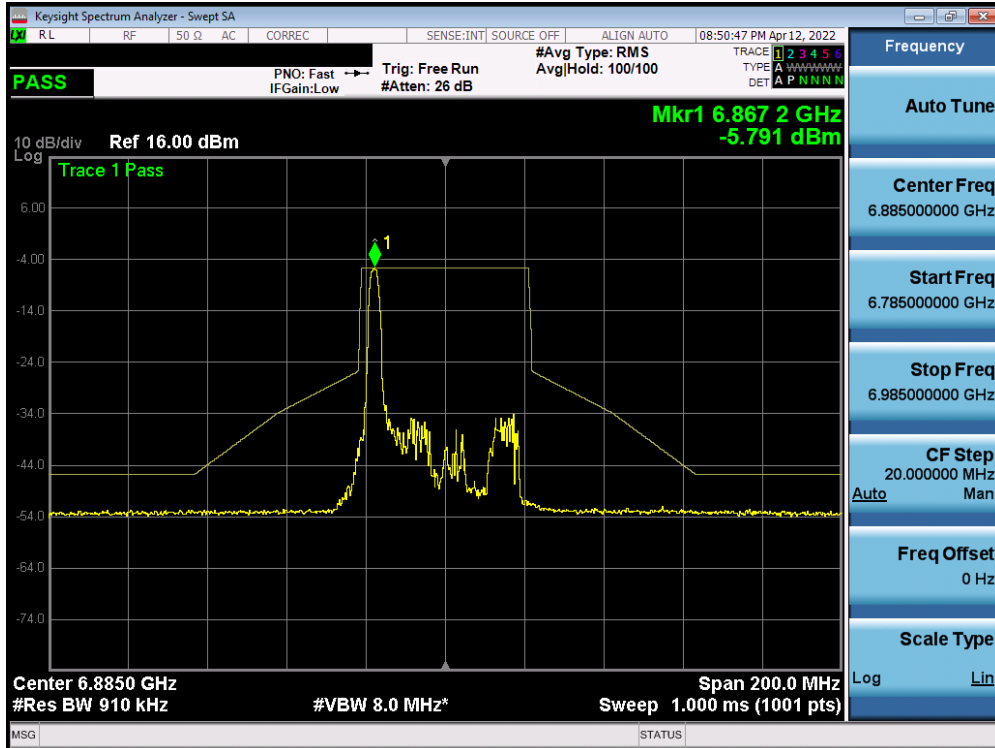
Plot 7-755. In-Band Emission Plot SISO ANT2 (40MHz BW 802.11ax (26 Tones) (UNII Band 8) – Ch. 187)
