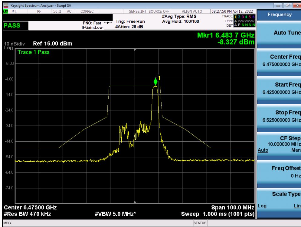
Plot 7-734. In-Band Emission Plot SISO ANT2 (20MHz BW 802.11ax (26 Tones) (UNII Band 6) – Ch. 105)
