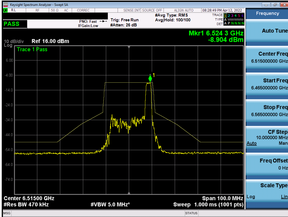
Plot 7-735. In-Band Emission Plot SISO ANT2 (20MHz BW 802.11ax (26 Tones) (UNII Band 6) – Ch. 113)
