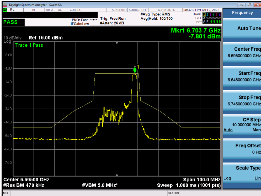
Plot 7-742. In-Band Emission Plot SISO ANT2 (20MHz BW 802.11ax (26 Tones) (UNII Band 7) – Ch. 149)
