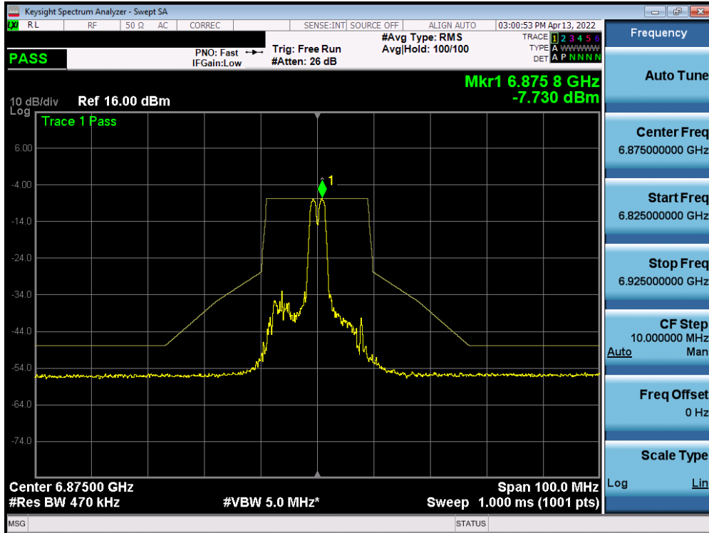
Plot 7-663. In-Band Emission Plot SISO ANT1 (20MHz BW 802.11ax (26 Tones) (UNII Band 7) – Ch. 185)
