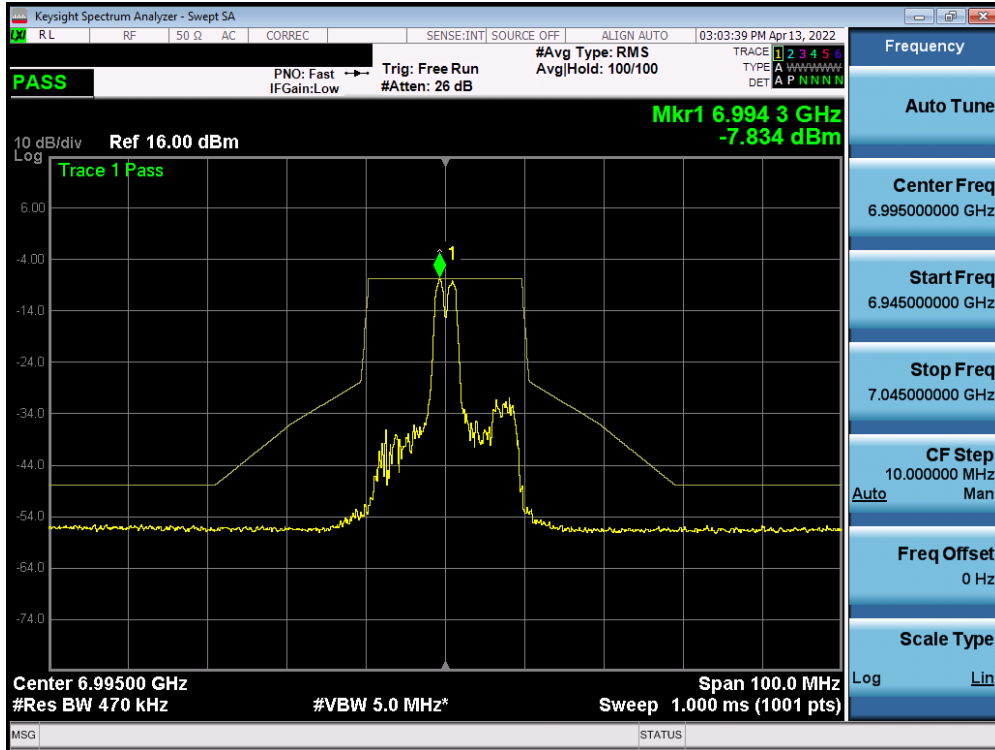
Plot 7-673. In-Band Emission Plot SISO ANT1 (20MHz BW 802.11ax (26 Tones) (UNII Band 8) – Ch. 209)
