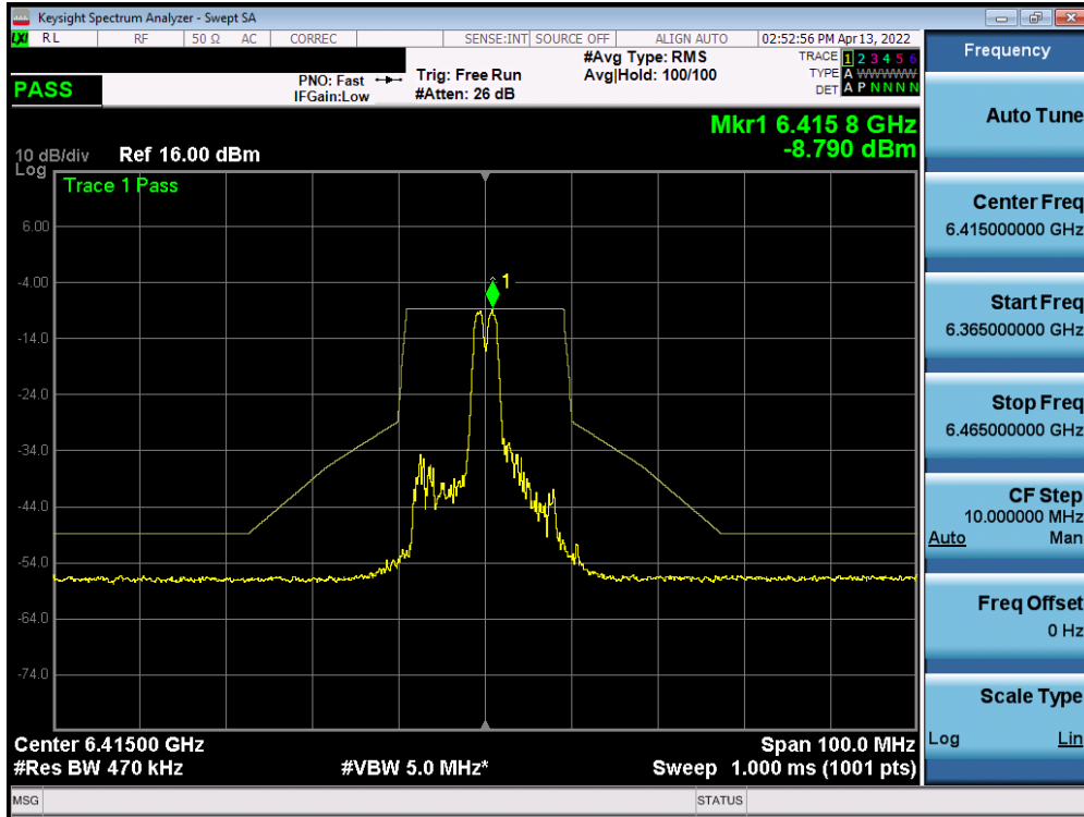
Plot 7-643. In-Band Emission Plot SISO ANT1 (20MHz BW 802.11ax (26 Tones) UNII Band 5) – Ch. 93)
