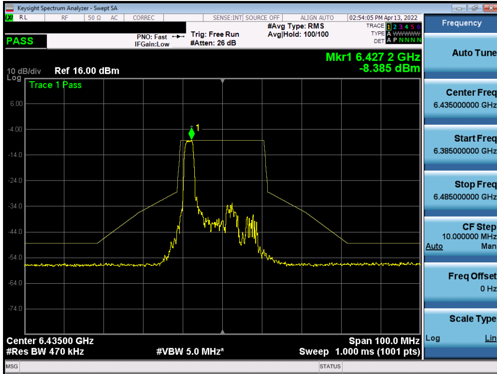
Plot 7-653. In-Band Emission Plot SISO ANT1 (20MHz BW 802.11ax (26 Tones) (UNII Band 6) – Ch. 97)
