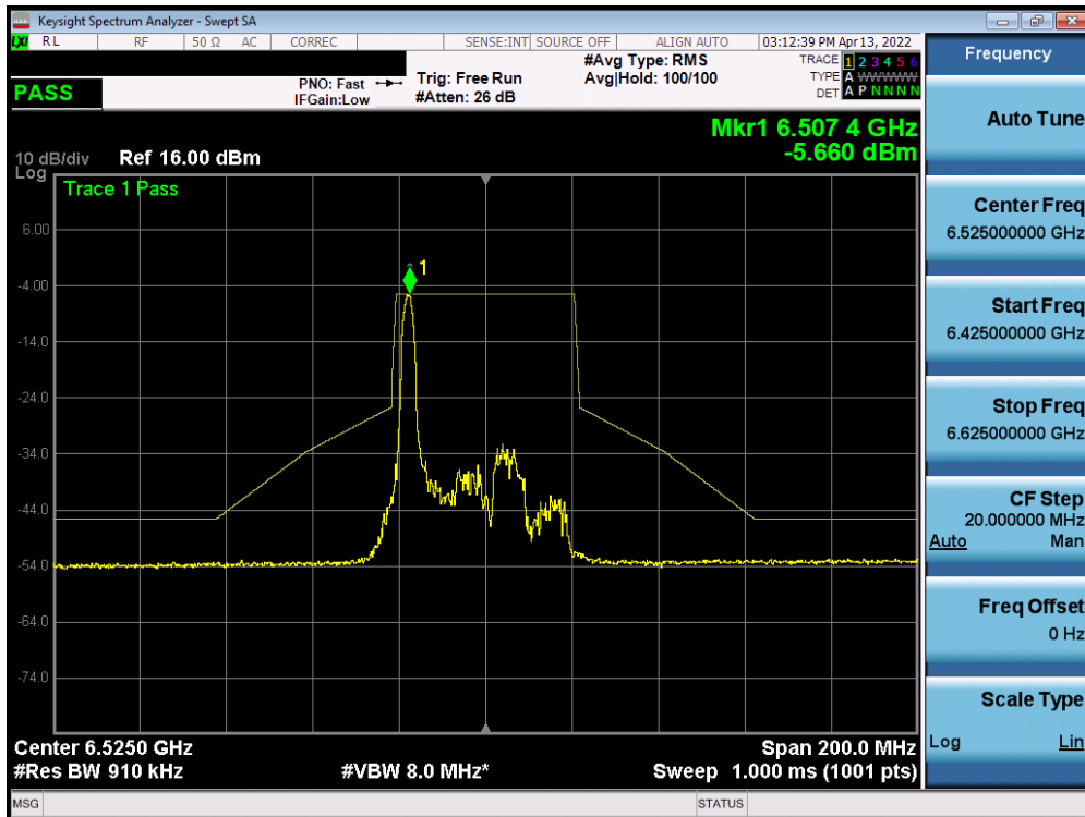
Plot 7-658. In-Band Emission Plot SISO ANT1 (40MHz BW 802.11ax (26 Tones) (UNII Band 6) – Ch. 115)
