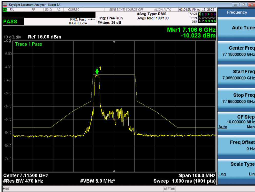
Plot 7-674. In-Band Emission Plot SISO ANT1 (20MHz BW 802.11ax (26 Tones) (UNII Band 8) – Ch. 233)
