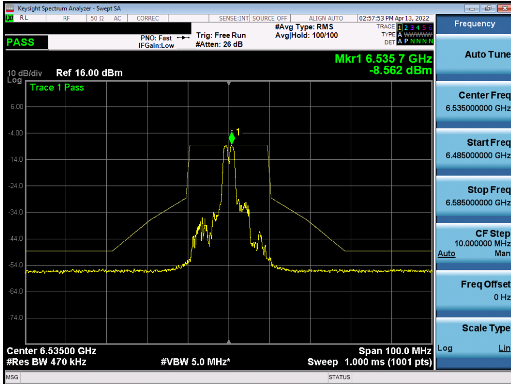
Plot 7-661. In-Band Emission Plot SISO ANT1 (20MHz BW 802.11ax (26 Tones) (UNII Band 7) – Ch. 117)
