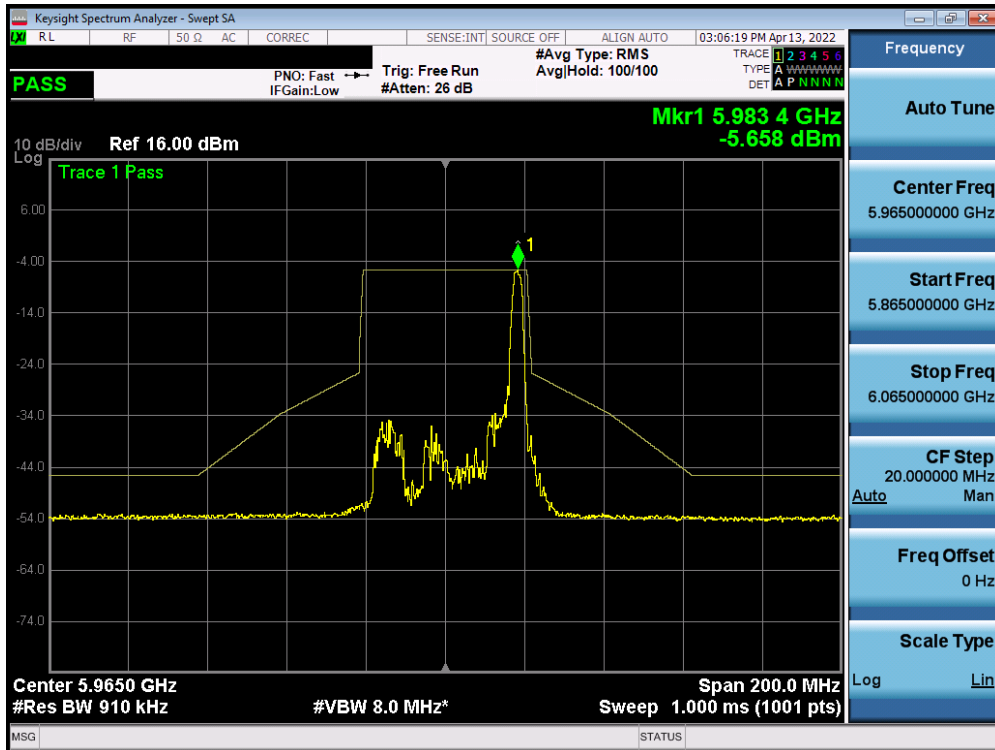
Plot 7-644. In-Band Emission Plot SISO ANT1 (40MHz BW 802.11ax (26 Tones) (UNII Band 5) – Ch. 3)
