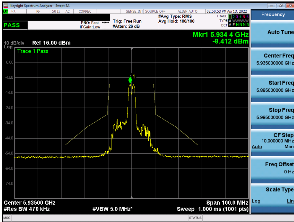
Plot 7-641. In-Band Emission Plot SISO ANT1 (20MHz BW 802.11ax (26 Tones) UNII Band 5) – Ch. 2
