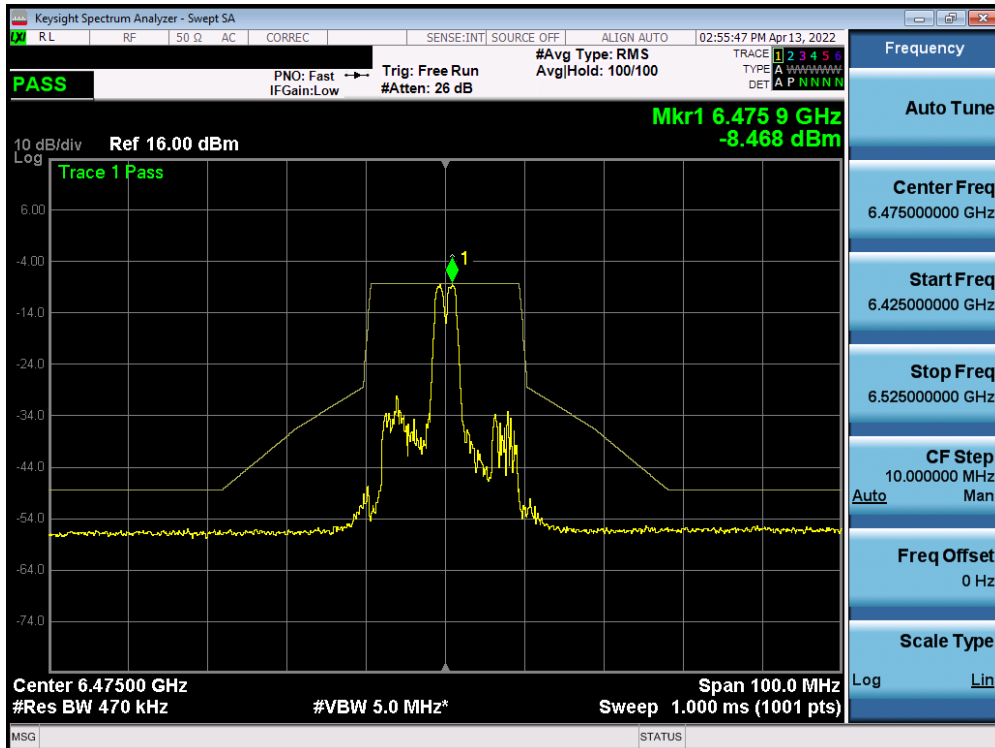
Plot 7-654. In-Band Emission Plot SISO ANT1 (20MHz BW 802.11ax (26 Tones) (UNII Band 6) – Ch. 105)
