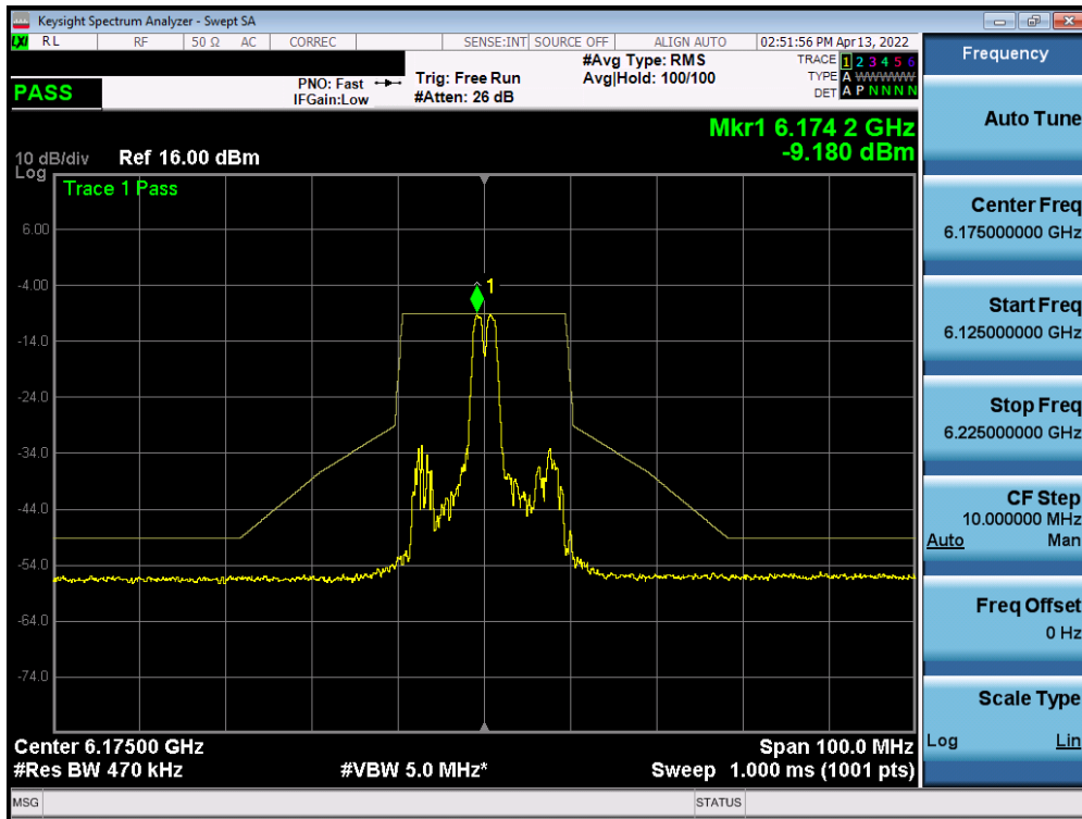
Plot 7-642. In-Band Emission Plot SISO ANT1 (20MHz BW 802.11ax (26 Tones) (UNII Band 5) – Ch. 45)
