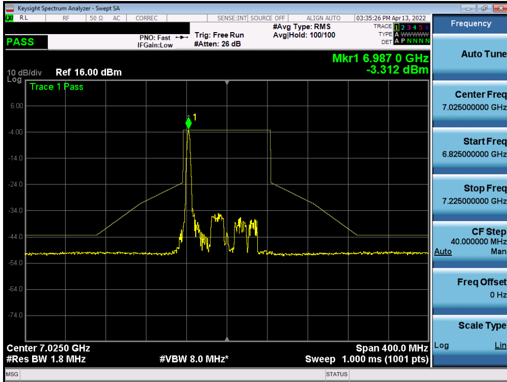
Plot 7-679. In-Band Emission Plot SISO ANT1 (80MHz BW 802.11ax (26 Tones) (UNII Band 8) – Ch. 215)
