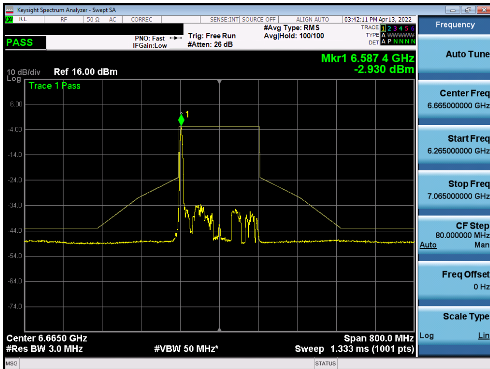
Plot 7-670. In-Band Emission Plot SISO ANT1 (160MHz BW 802.11ax (26 Tones) (UNII Band 7) – Ch. 143)
