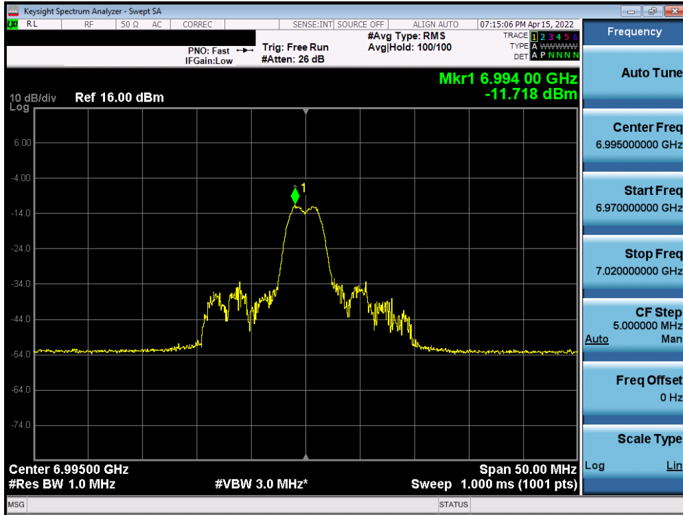
Plot 7-593. Power Spectral Density Plot MIMO ANT2 (20MHz BW 802.11ax (26 Tones) (UNII Band 8) – Ch. 209)
