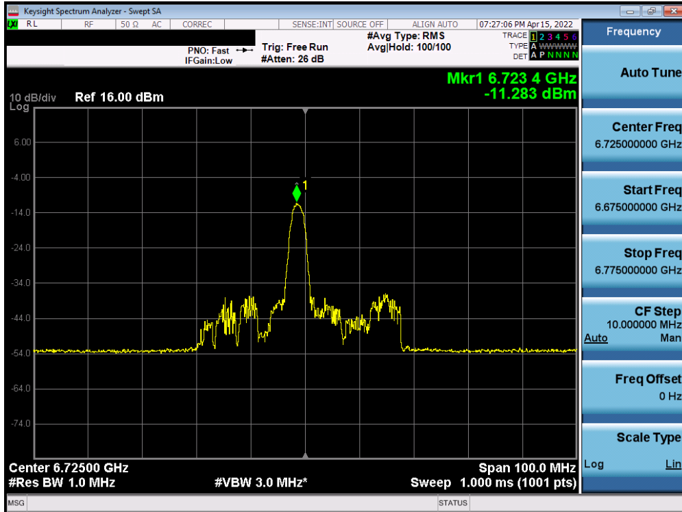
Plot 7-585. Power Spectral Density Plot MIMO ANT2 (40MHz BW 802.11ax (26 Tones) (UNII Band 7) – Ch. 155)
