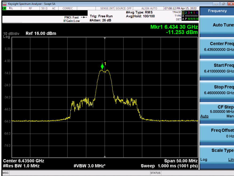
Plot 7-573. Power Spectral Density Plot MIMO ANT2 (20MHz BW 802.11ax (26 Tones) (UNII Band 6) – Ch. 97)
