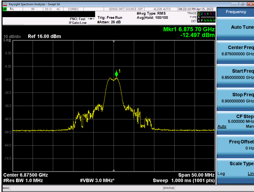
Plot 7-503. Power Spectral Density Plot MIMO ANT1 (20MHz BW 802.11ax (26 Tones) (UNII Band 7) – Ch. 185)
