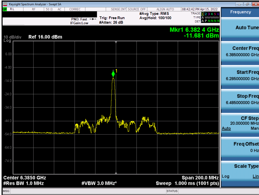
Plot 7-489. Power Spectral Density Plot MIMO ANT1 (80MHz BW 802.11ax (26 Tones) (UNII Band 5) – Ch. 87)
