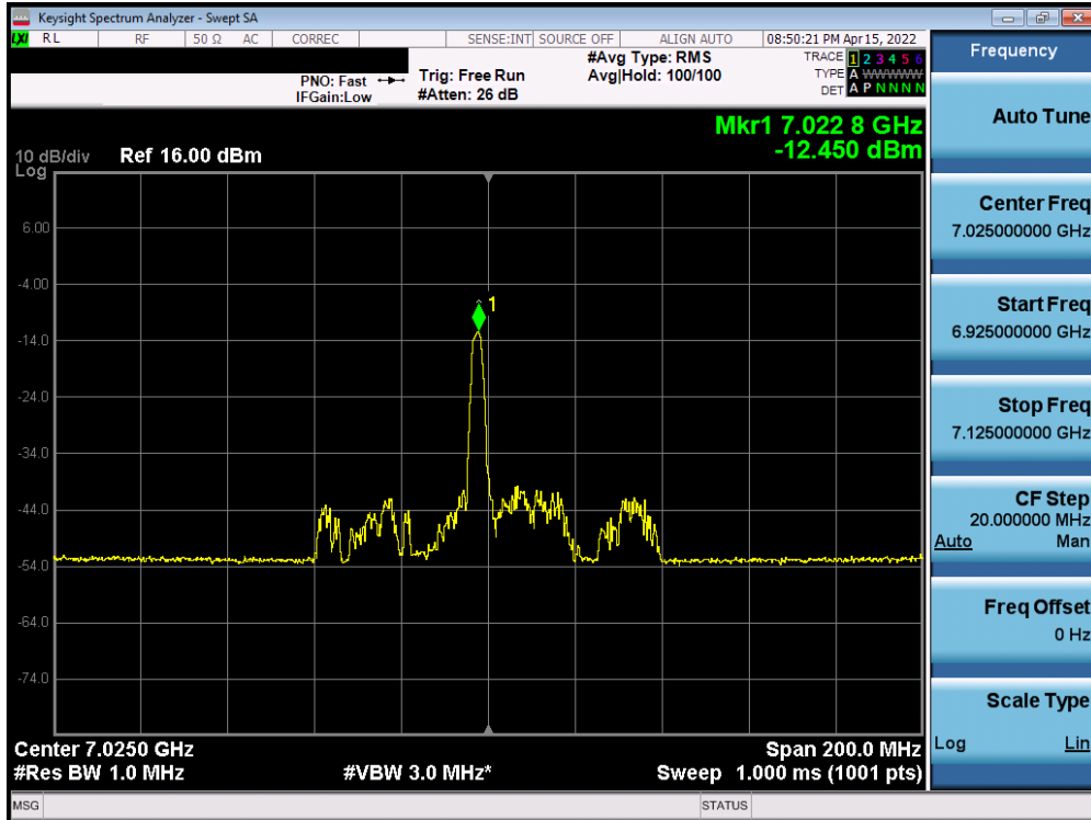
Plot 7-519. Power Spectral Density Plot MIMO ANT1 (80MHz BW 802.11ax (26 Tones) (UNII Band 8) – Ch. 215)
