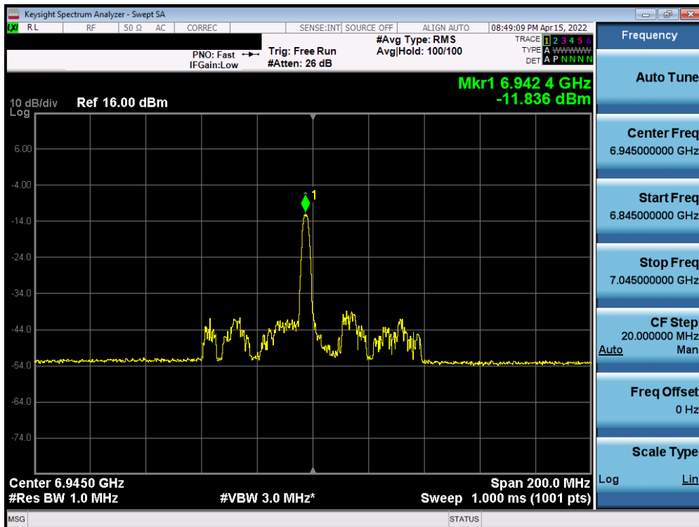
Plot 7-518. Power Spectral Density Plot MIMO ANT1 (80MHz BW 802.11ax (26 Tones) (UNII Band 8) – Ch. 199)
