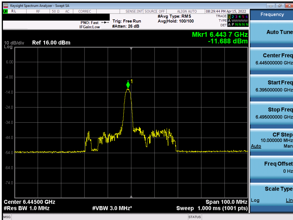
Plot 7-496. Power Spectral Density Plot MIMO ANT1 (40MHz BW 802.11ax (26 Tones) (UNII Band 6) – Ch. 99)
