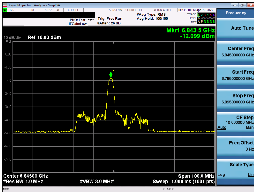
Plot 7-506. Power Spectral Density Plot MIMO ANT1 (40MHz BW 802.11ax (26 Tones) (UNII Band 7) – Ch. 179)
