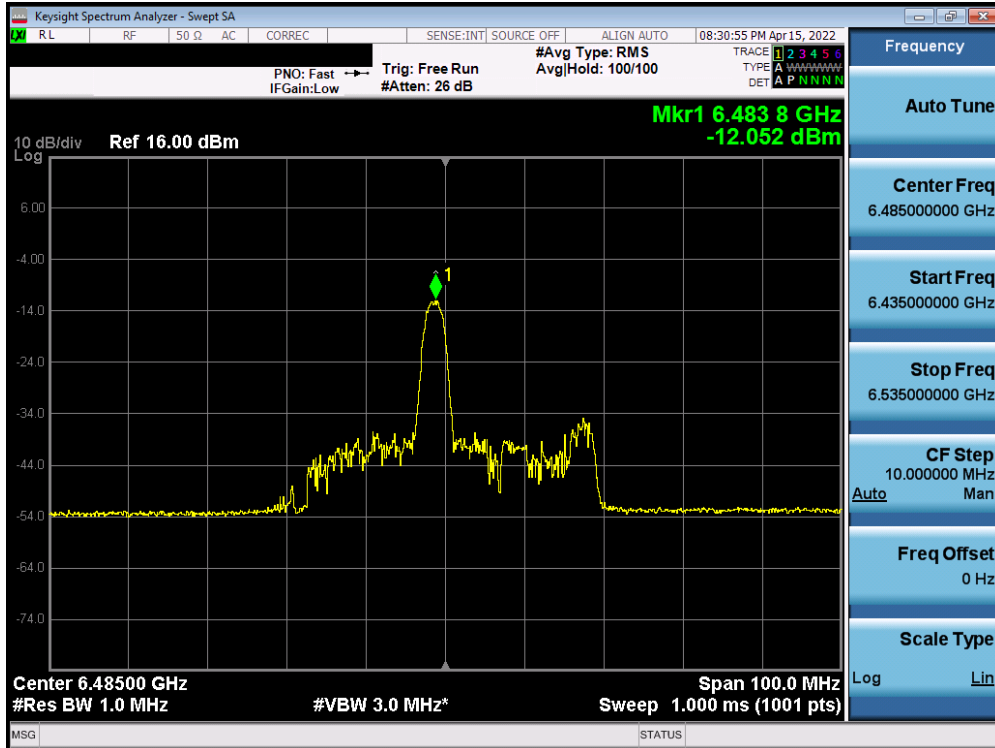
Plot 7-497. Power Spectral Density Plot MIMO ANT1 (40MHz BW 802.11ax (26 Tones) (UNII Band 6) – Ch. 107)
