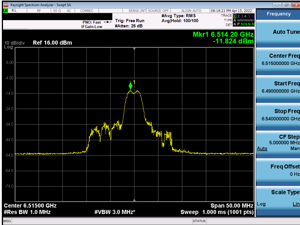
Plot 7-495. Power Spectral Density Plot MIMO ANT1 (20MHz BW 802.11ax (26 Tones) (UNII Band 6) – Ch. 113)
