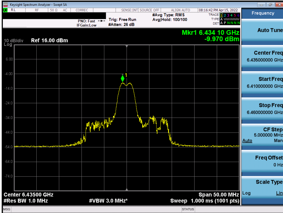
Plot 7-493. Power Spectral Density Plot MIMO ANT1 (20MHz BW 802.11ax (26 Tones) (UNII Band 6) – Ch. 97)
