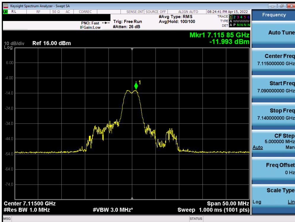
Plot 7-514. Power Spectral Density Plot MIMO ANT1 (20MHz BW 802.11ax (26 Tones) (UNII Band 8) – Ch. 233)
