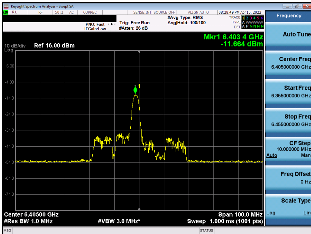
Plot 7-486. Power Spectral Density Plot MIMO ANT1 (40MHz BW 802.11ax (26 Tones) (UNII Band 5) – Ch. 91)
