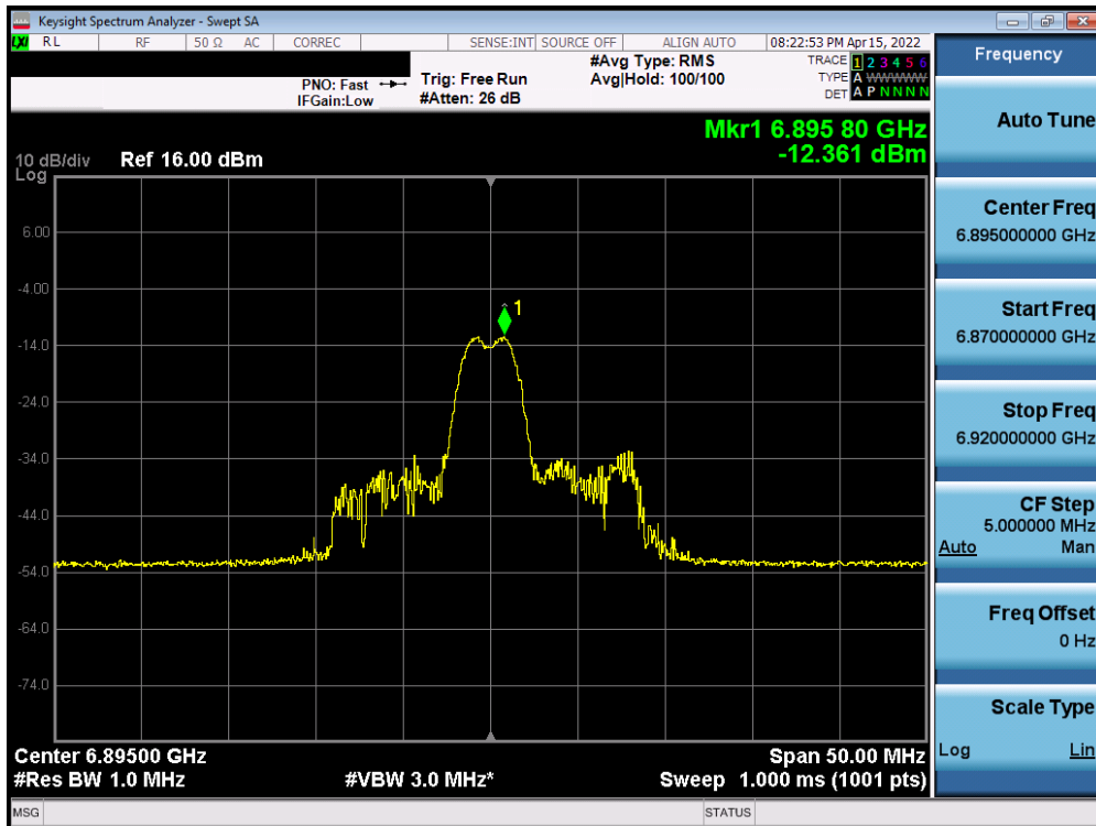
Plot 7-512. Power Spectral Density Plot MIMO ANT1 (20MHz BW 802.11ax (26 Tones) (UNII Band 8) – Ch. 189)
