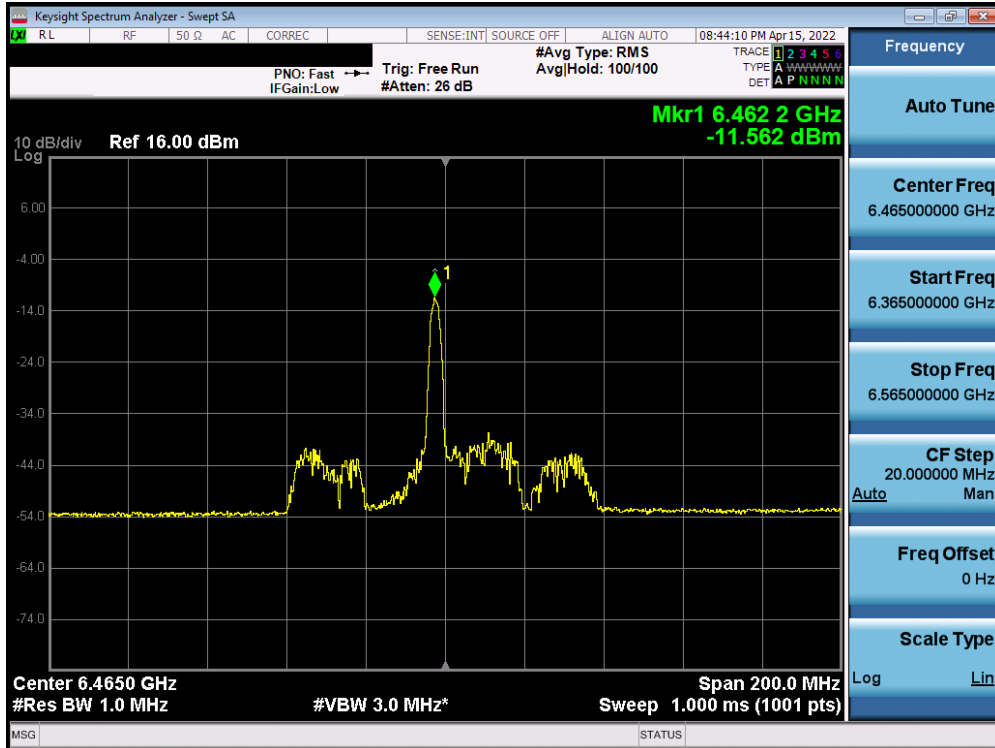
Plot 7-499. Power Spectral Density Plot MIMO ANT1 (80MHz BW 802.11ax (26 Tones) (UNII Band 6) – Ch. 103)
