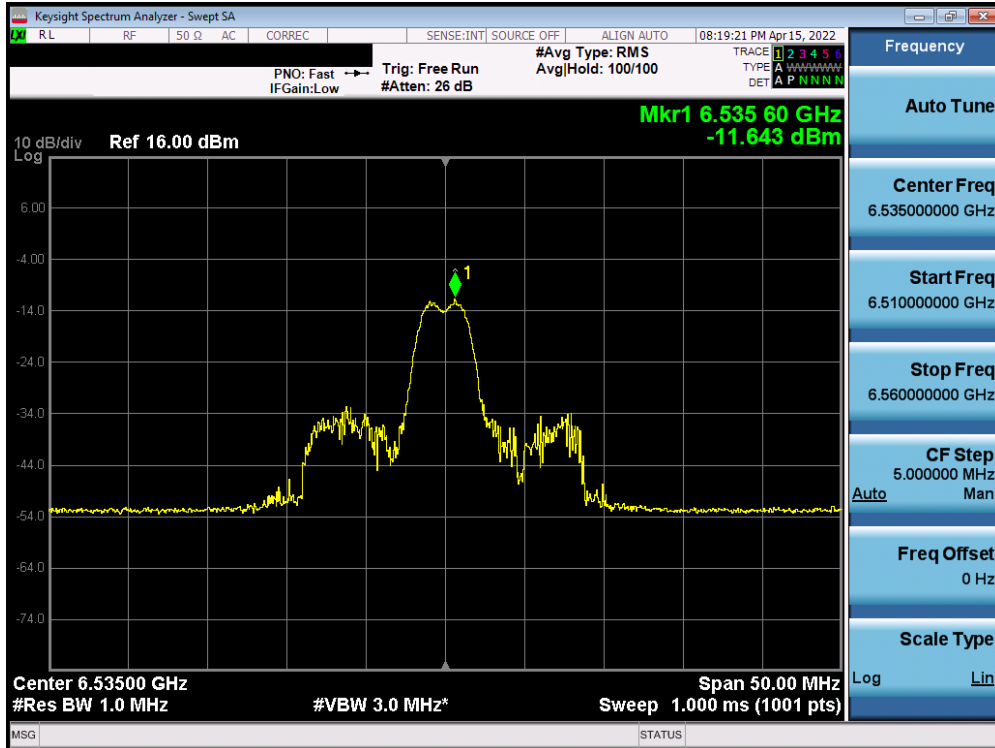
Plot 7-501. Power Spectral Density Plot MIMO ANT1 (20MHz BW 802.11ax (26 Tones) (UNII Band 7) – Ch. 117)
