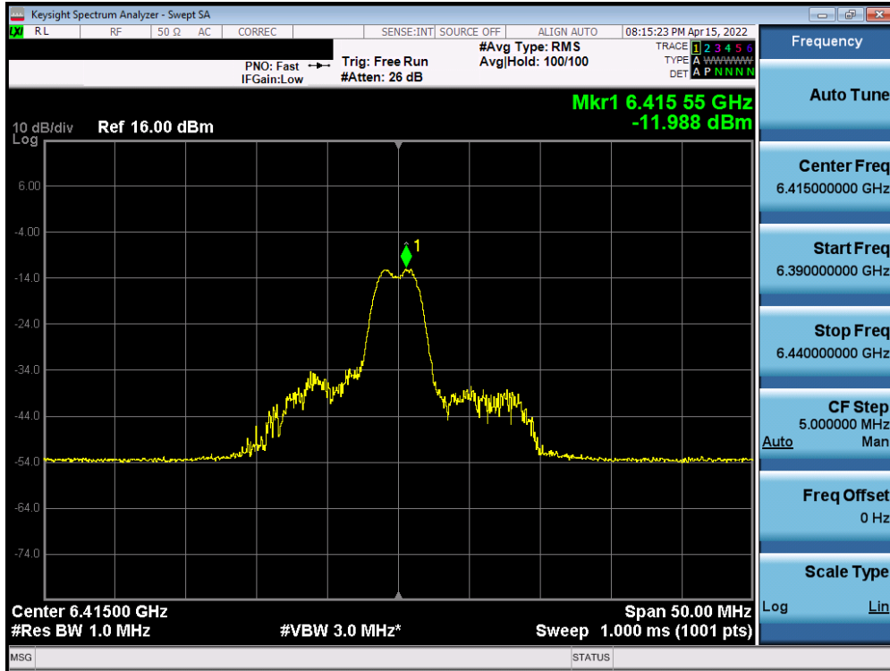
Plot 7-483. Power Spectral Density Plot MIMO ANT1 (20MHz BW 802.11ax (26 Tones) UNII Band 5) – Ch. 93)
