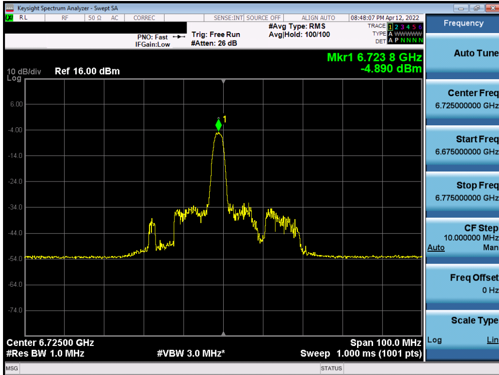
Plot 7-425. Power Spectral Density Plot SISO ANT2 (40MHz BW 802.11ax (26 Tones) (UNII Band 7) – Ch. 155)
