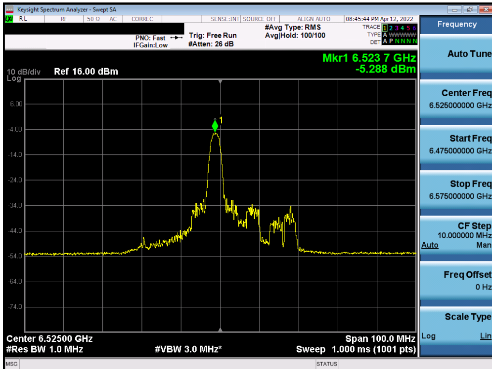
Plot 7-418. Power Spectral Density Plot SISO ANT2 (40MHz BW 802.11ax (26 Tones) (UNII Band 6) – Ch. 115)
