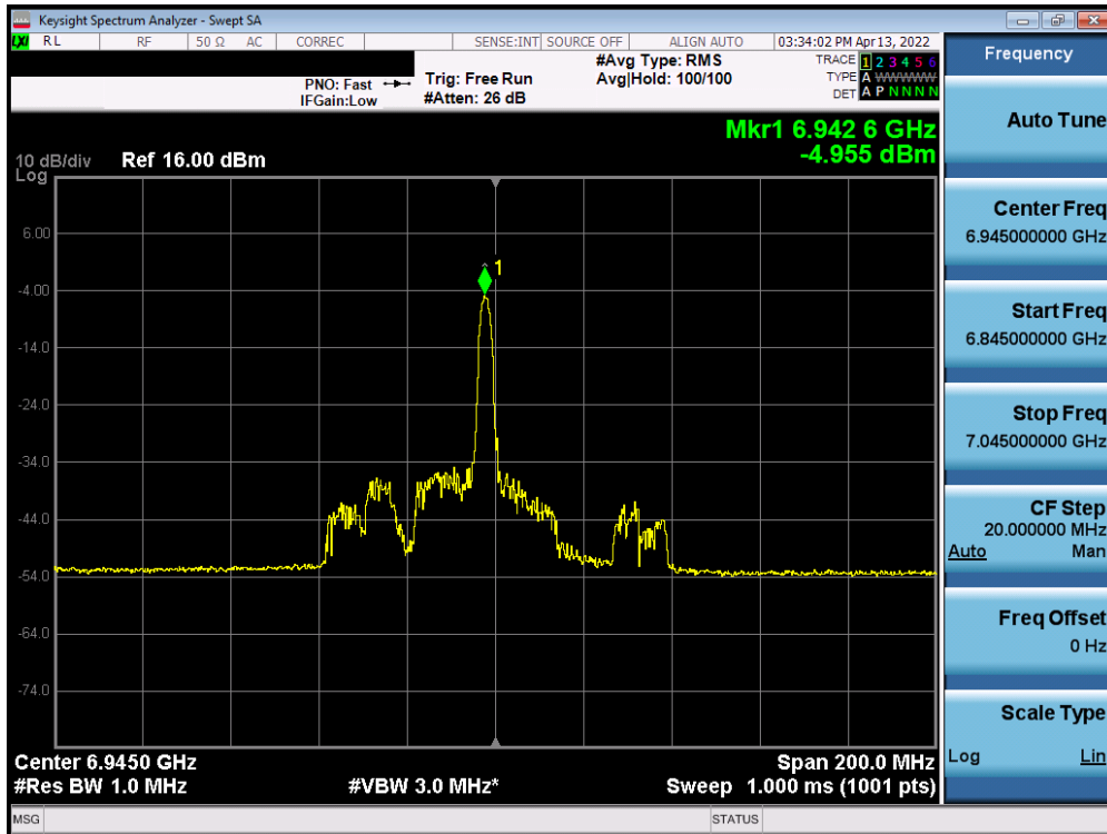
Plot 7-358. Power Spectral Density Plot SISO ANT1 (80MHz BW 802.11ax (26 Tones) (UNII Band 8) – Ch. 199)
