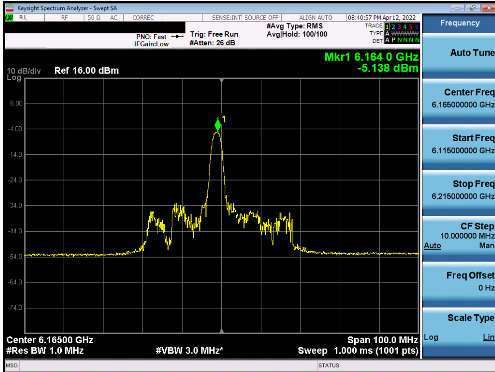
Plot 7-405. Power Spectral Density Plot SISO ANT2 (40MHz BW 802.11ax (26 Tones) (UNII Band 5) – Ch. 43)
