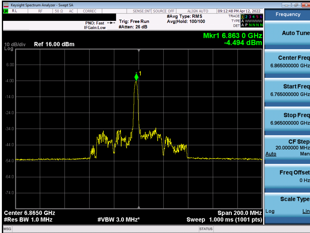
Plot 7-429. Power Spectral Density Plot SISO ANT2 (80MHz BW 802.11ax (26 Tones) (UNII Band 7) – Ch. 183)
