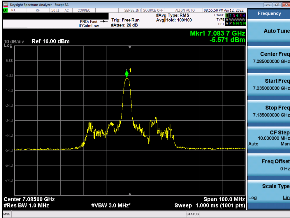
Plot 7-437. Power Spectral Density Plot SISO ANT2 (40MHz BW 802.11ax (26 Tones) (UNII Band 8) – Ch. 227)
