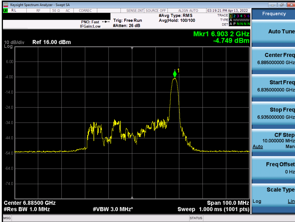
Plot 7-355. Power Spectral Density Plot SISO ANT1 (40MHz BW 802.11ax (26 Tones) (UNII Band 8) – Ch. 187)
