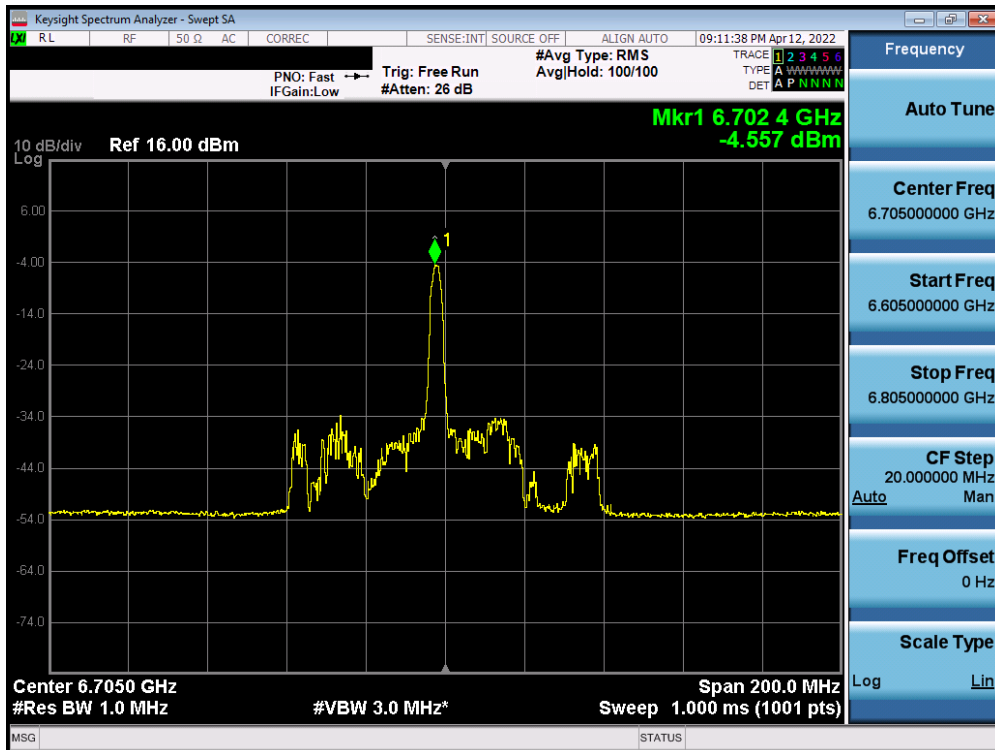
Plot 7-428. Power Spectral Density Plot SISO ANT2 (80MHz BW 802.11ax (26 Tones) (UNII Band 7) – Ch. 151)
