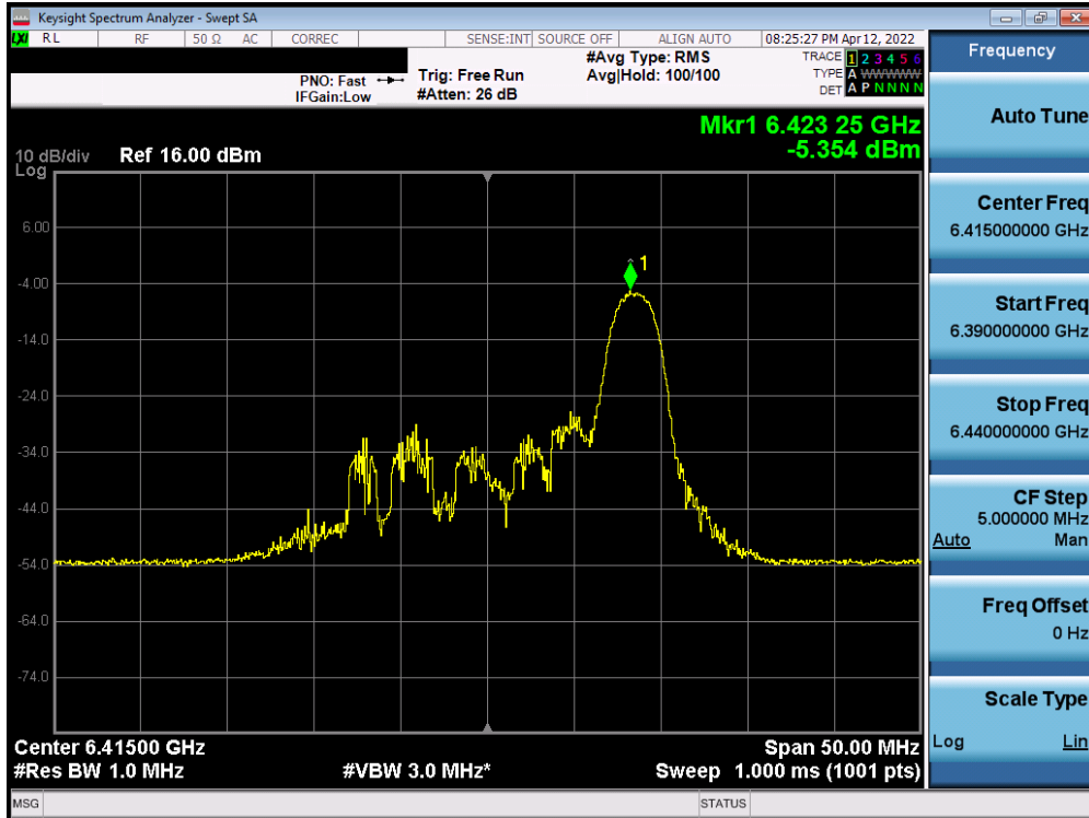
Plot 7-403. Power Spectral Density Plot SISO ANT2 (20MHz BW 802.11ax (26 Tones) UNII Band 5) – Ch. 93)
