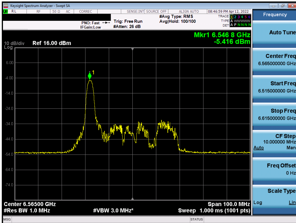
Plot 7-424. Power Spectral Density Plot SISO ANT2 (40MHz BW 802.11ax (26 Tones) (UNII Band 7) – Ch. 123)
