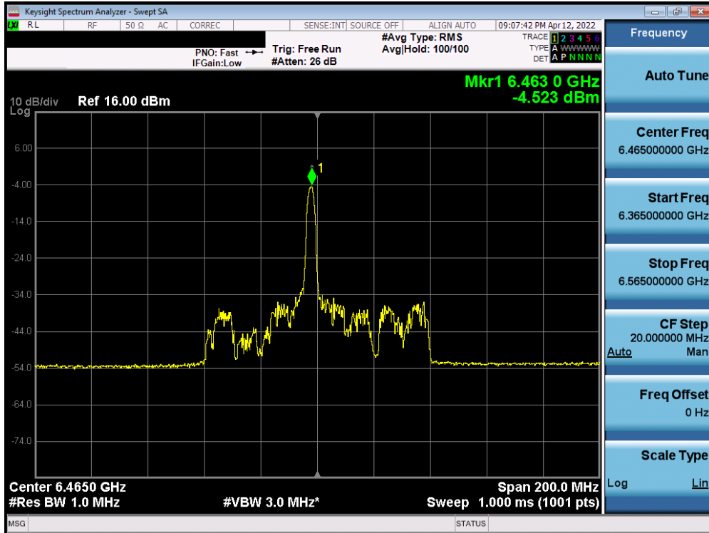
Plot 7-419. Power Spectral Density Plot SISO ANT2 (80MHz BW 802.11ax (26 Tones) (UNII Band 6) – Ch. 103)
