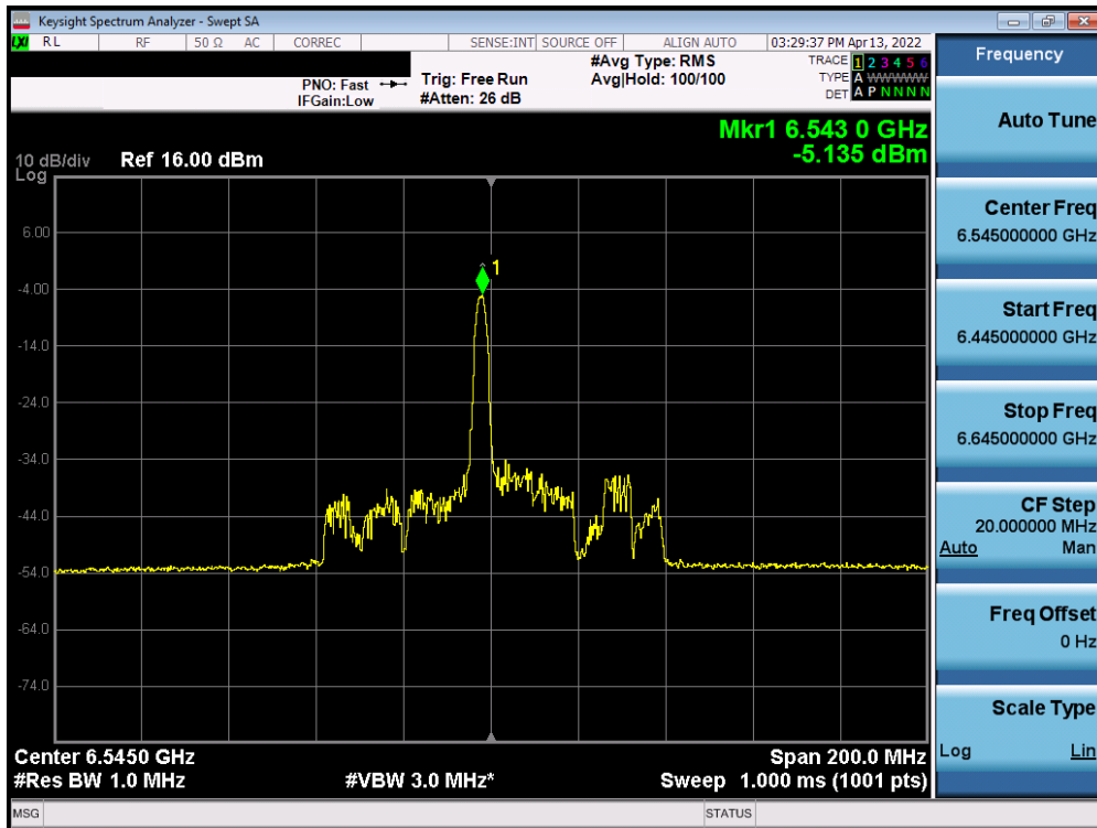
Plot 7-347. Power Spectral Density Plot SISO ANT1 (80MHz BW 802.11ax (26 Tones) (UNII Band 7) – Ch. 119)
