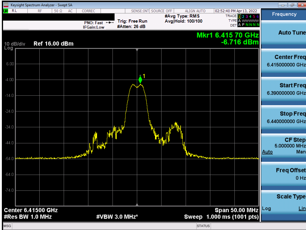
Plot 7-323. Power Spectral Density Plot SISO ANT1 (20MHz BW 802.11ax (26 Tones) UNII Band 5) – Ch. 93)
