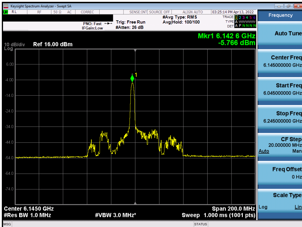
Plot 7-328. Power Spectral Density Plot SISO ANT1 (80MHz BW 802.11ax (26 Tones) (UNII Band 5) – Ch. 39)
