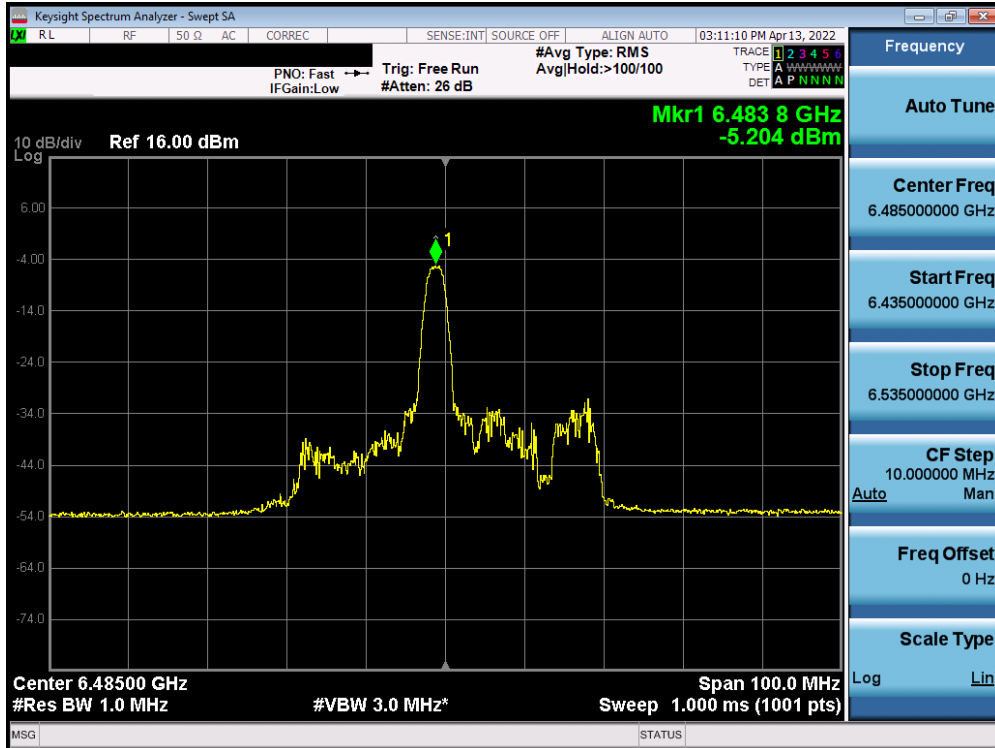
Plot 7-337. Power Spectral Density Plot SISO ANT1 (40MHz BW 802.11ax (26 Tones) (UNII Band 6) – Ch. 107)
