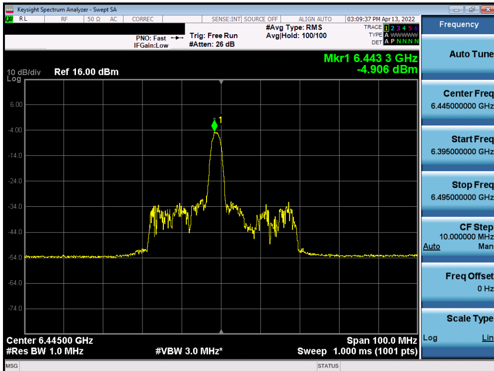
Plot 7-336. Power Spectral Density Plot SISO ANT1 (40MHz BW 802.11ax (26 Tones) (UNII Band 6) – Ch. 99)
