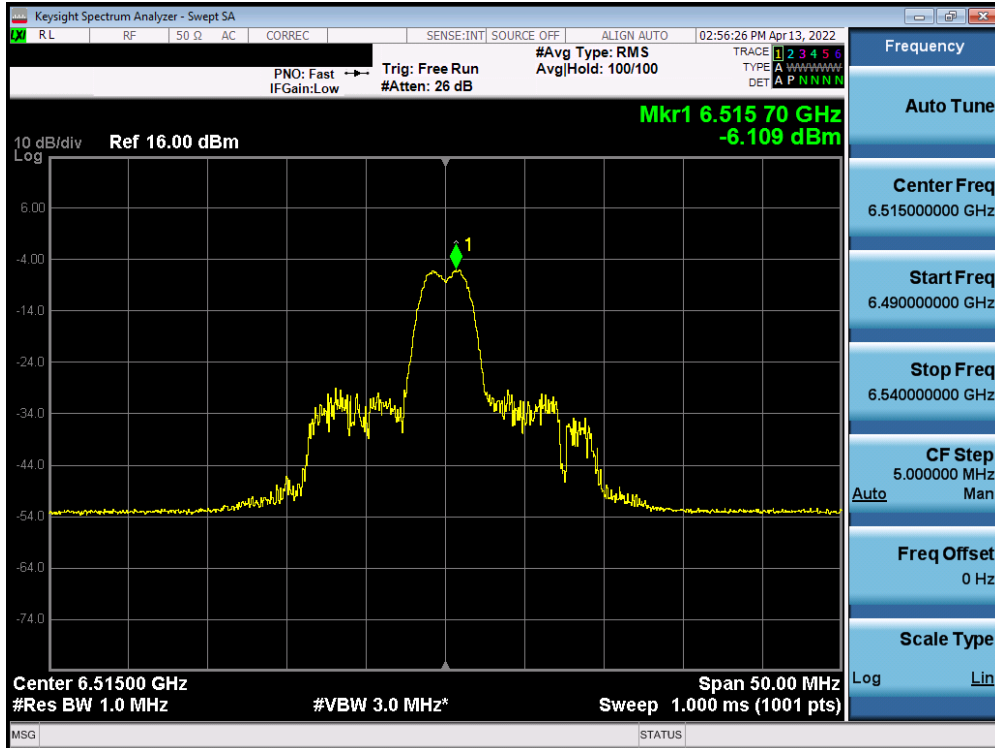
Plot 7-335. Power Spectral Density Plot SISO ANT1 (20MHz BW 802.11ax (26 Tones) (UNII Band 6) – Ch. 113)
