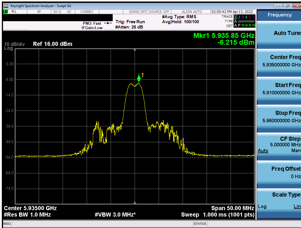
Plot 7-321. Power Spectral Density Plot SISO ANT1 (20MHz BW 802.11ax (26 Tones) UNII Band 5) – Ch. 2
