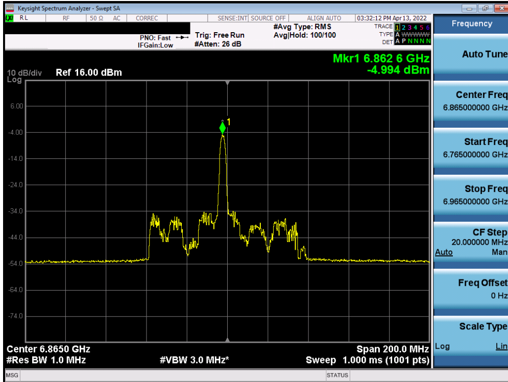
Plot 7-349. Power Spectral Density Plot SISO ANT1 (80MHz BW 802.11ax (26 Tones) (UNII Band 7) – Ch. 183)
