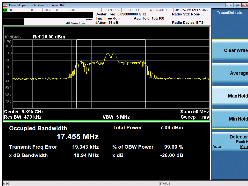
Plot 7-112. Occupied Bandwidth Plot SISO ANT2 (20MHz BW 802.11ax (26 Tones) (UNII Band 8) – Ch. 189)
