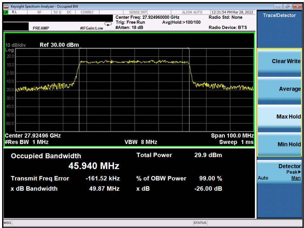
Plot 7-11. Occupied Bandwidth Plot (50MHz-1CC – 16QAM – Mid Channel)
