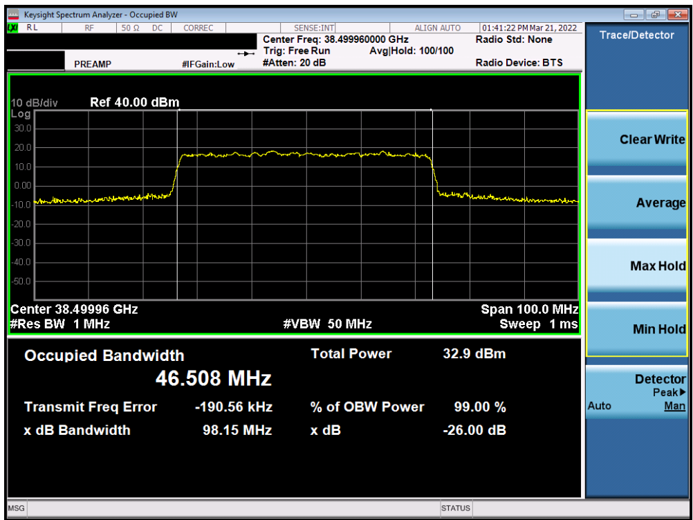
Plot 7-25. Occupied Bandwidth Plot (50MHz-1CC – QPSK – Mid Channel)
