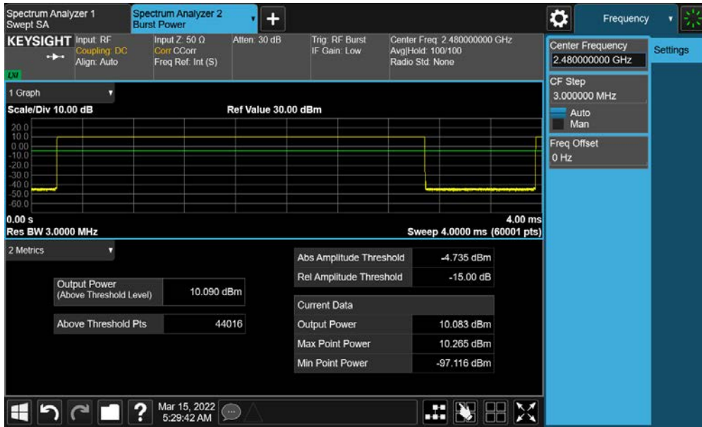
Plot 7-21. Average Conducted Power (1Mbps – Ch. 78)
