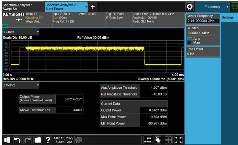
Plot 7-23. Average Conducted Power (2Mbps – Ch. 39)
