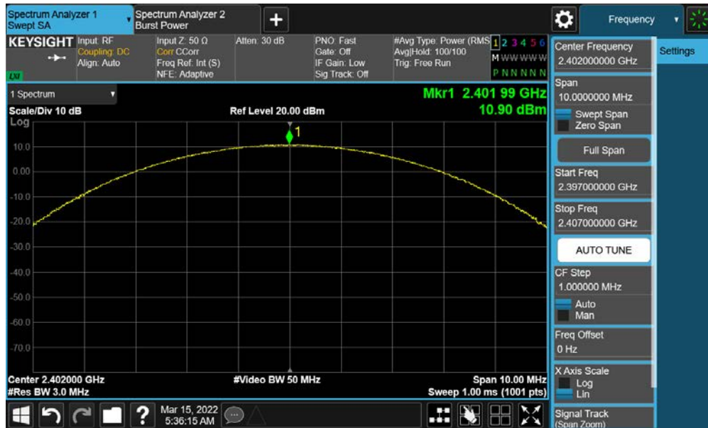
Plot 7-16. Peak Conducted Power (3Mbps – Ch. 0)
