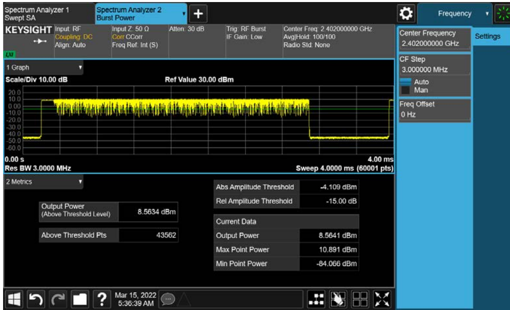
Plot 7-25. Average Conducted Power (3Mbps – Ch. 0)
