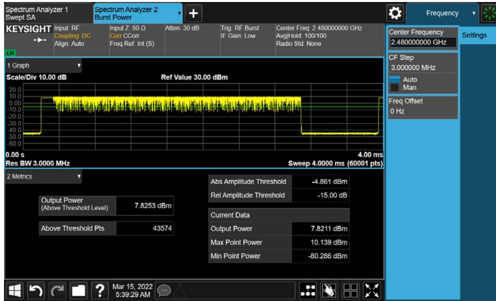
Plot 7-27. Average Conducted Power (3Mbps – Ch. 78)
