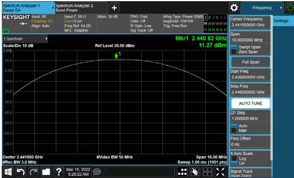
Plot 7-11. Peak Conducted Power (1Mbps – Ch. 39)
