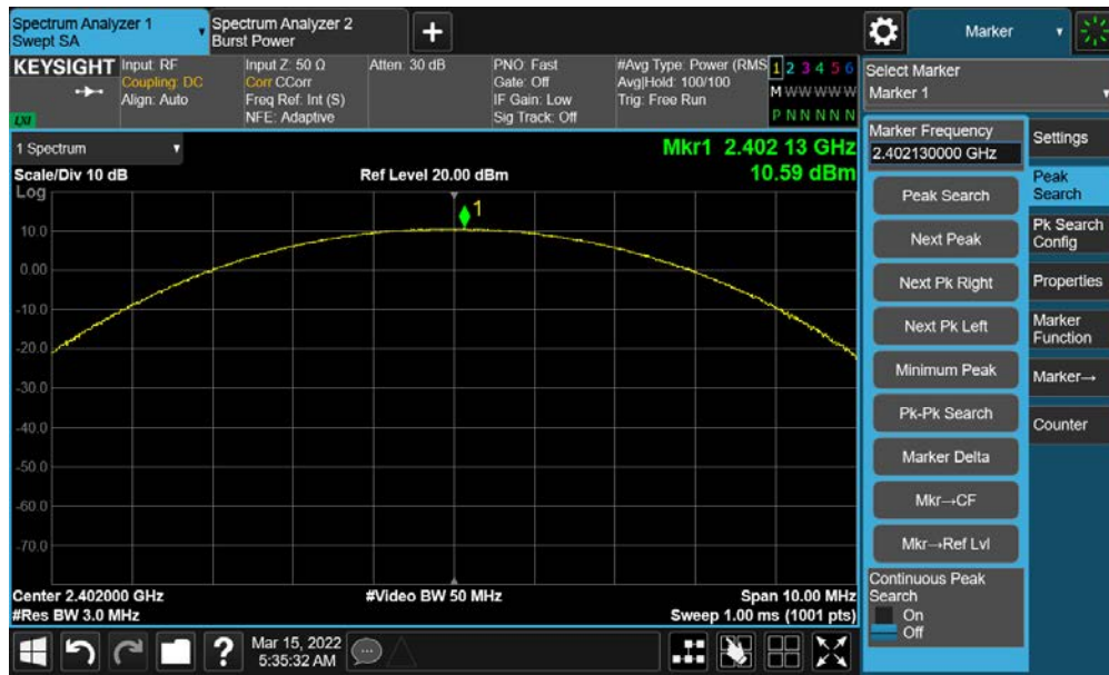
Plot 7-13. Peak Conducted Power (2Mbps – Ch. 0)
