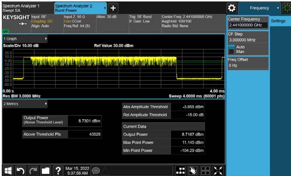
Plot 7-26. Average Conducted Power (3Mbps – Ch. 39)
