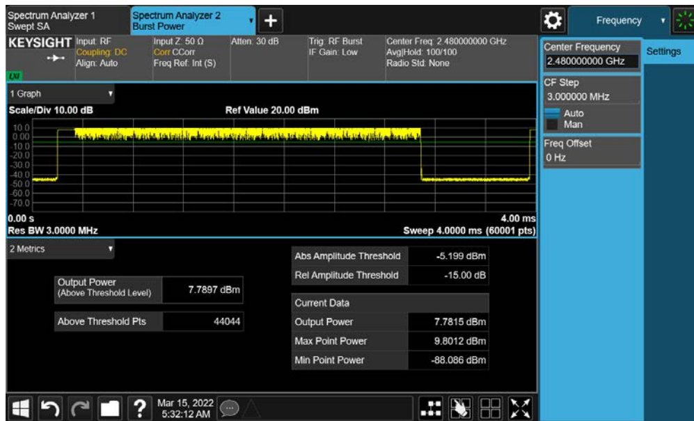
Plot 7-24. Average Conducted Power (2Mbps – Ch. 78)
