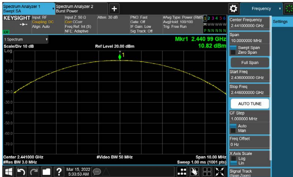
Plot 7-14. Peak Conducted Power (2Mbps – Ch. 39)
