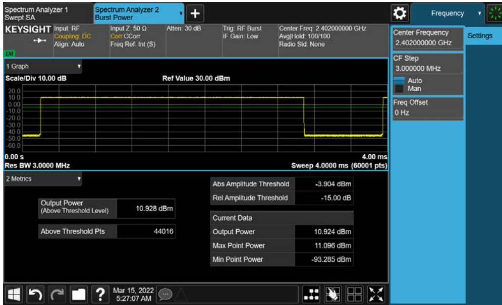
Plot 7-19. Average Conducted Power (1Mbps – Ch. 0)
