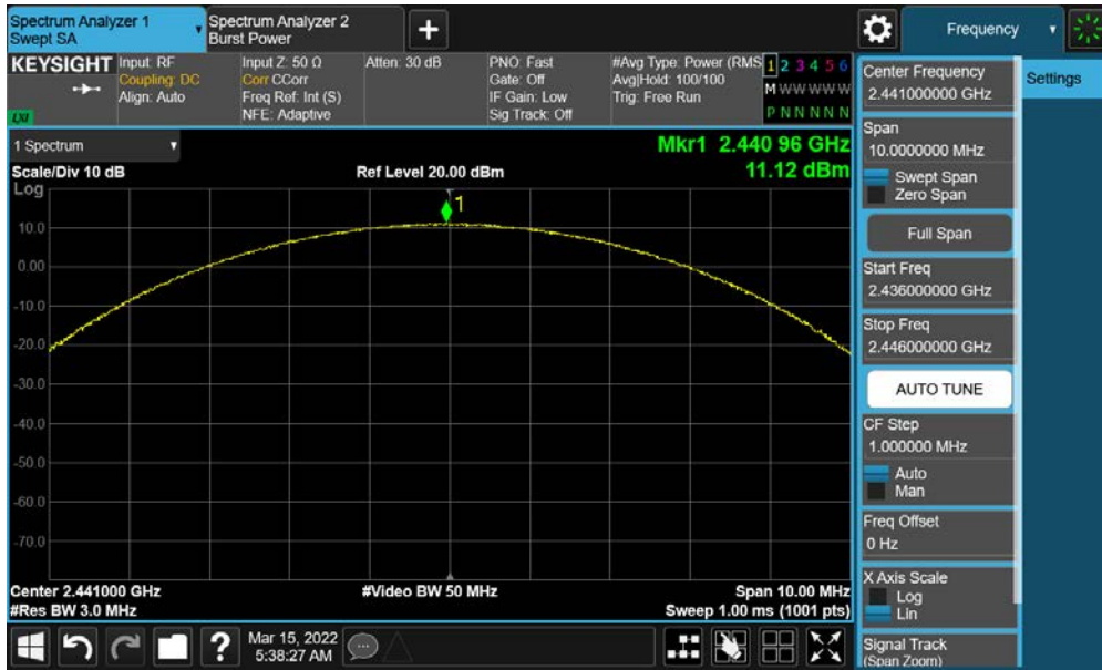
Plot 7-17. Peak Conducted Power (3Mbps – Ch. 39)
