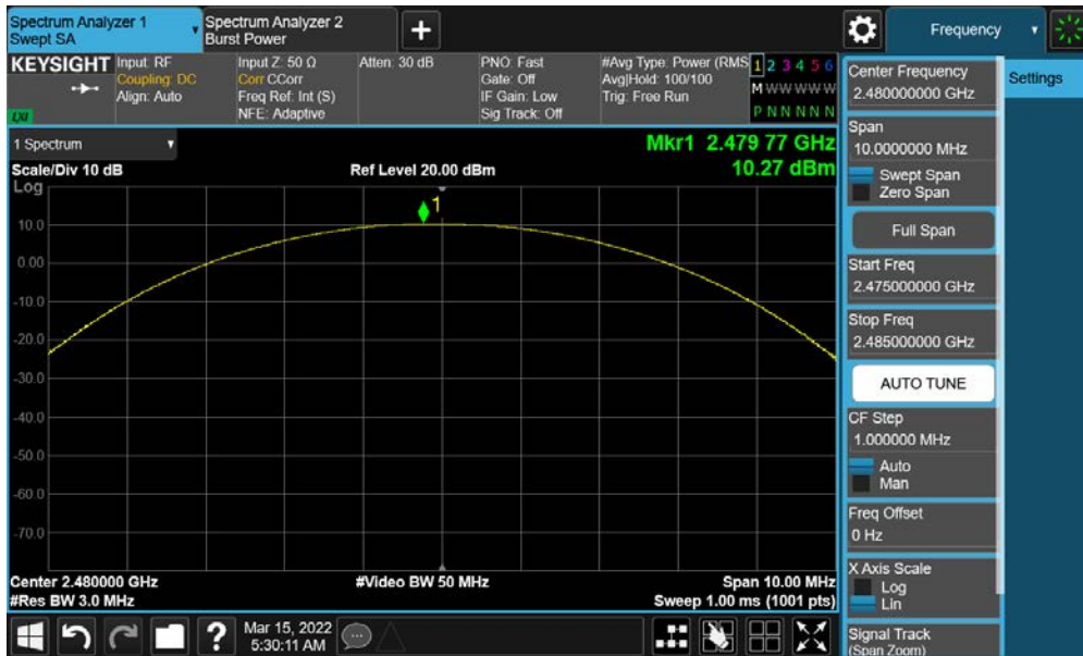
Plot 7-12. Peak Conducted Power (1Mbps – Ch. 78)
