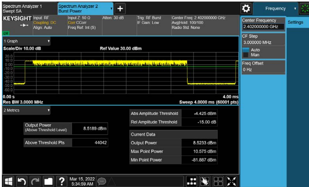
Plot 7-22. Average Conducted Power (2Mbps – Ch. 0)
