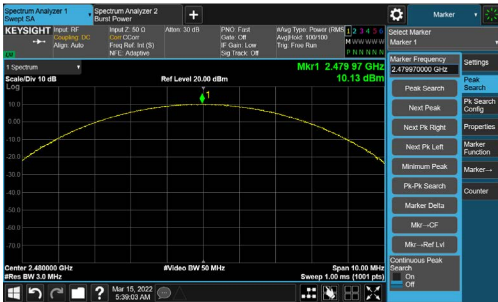
Plot 7-18. Peak Conducted Power (3Mbps – Ch. 78)
