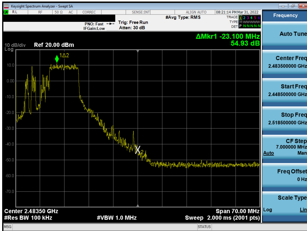
Plot 7-55. Band Edge Plot SISO ANT1 (802.11ax OFDMA – 106 Tones – Ch. 10) – 20MHz
