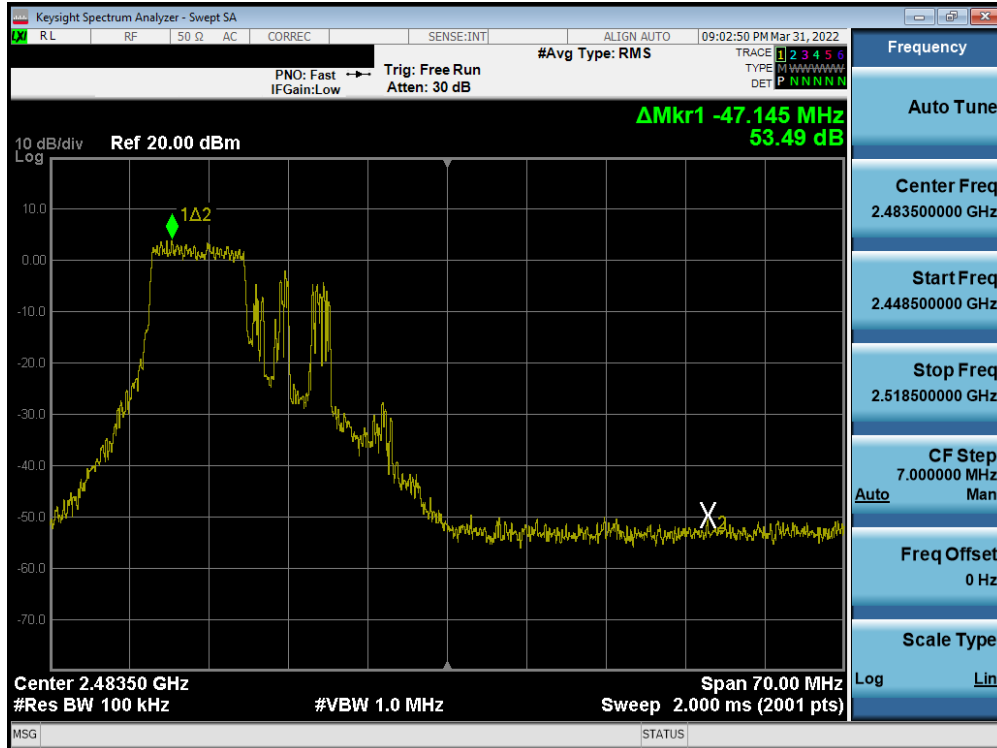
Plot 7-92. Band Edge Plot SISO ANT2 (802.11ax OFDMA – 106 Tones – Ch. 12) – 20MHz
