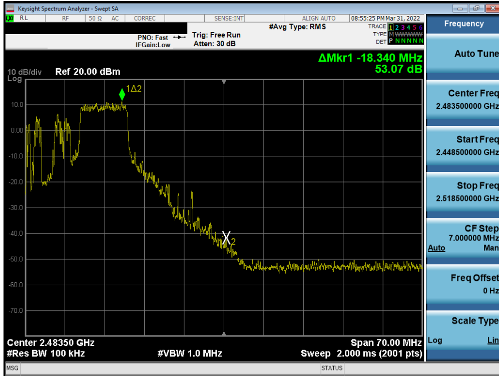
Plot 7-90. Band Edge Plot SISO ANT2 (802.11ax OFDMA – 106 Tones – Ch. 10) – 20MHz
