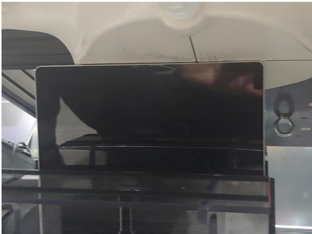
SAR Test Setup Photo 8 – Tablet, Top Edge at 0 mm – Antenna 1 & 2
