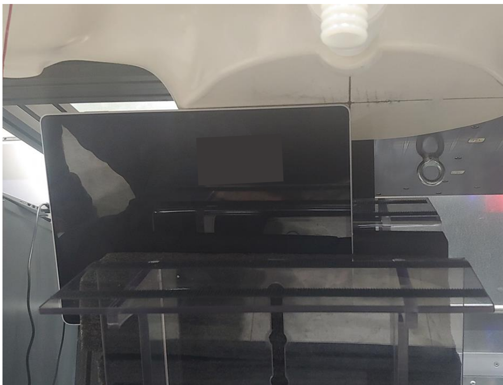
SAR Test Setup Photo 16 – Tablet, Bottom Edge at 0mm – Antenna 5 & 6
