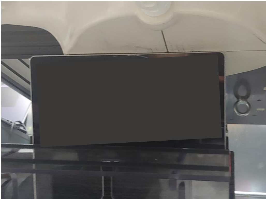
SAR Test Setup Photo 15 – Tablet, Bottom Edge at 0mm – Antenna 3 & 4
