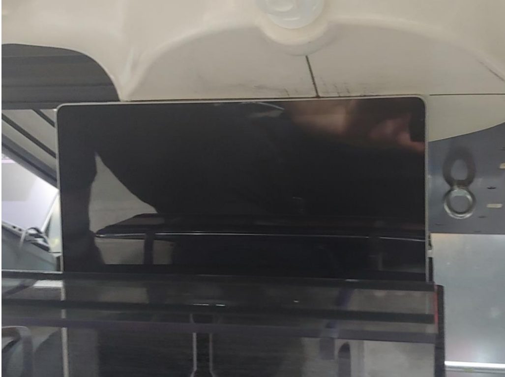
SAR Test Setup Photo 9 – Tablet with keyboard accessory, Top Edge at 0 mm – Antenna 1 & 2
