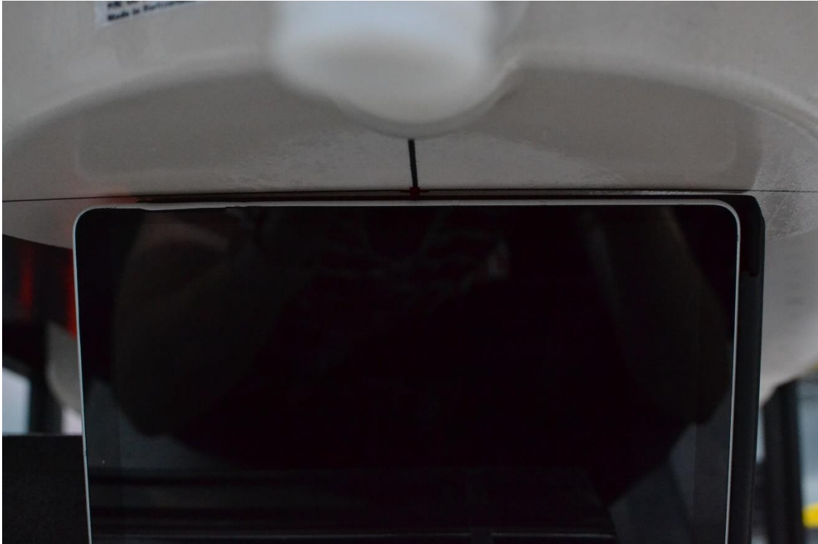
SAR Test Setup Photo 23 – Tablet with keyboard accessory, Right Edge at 0 mm – All Antennas
