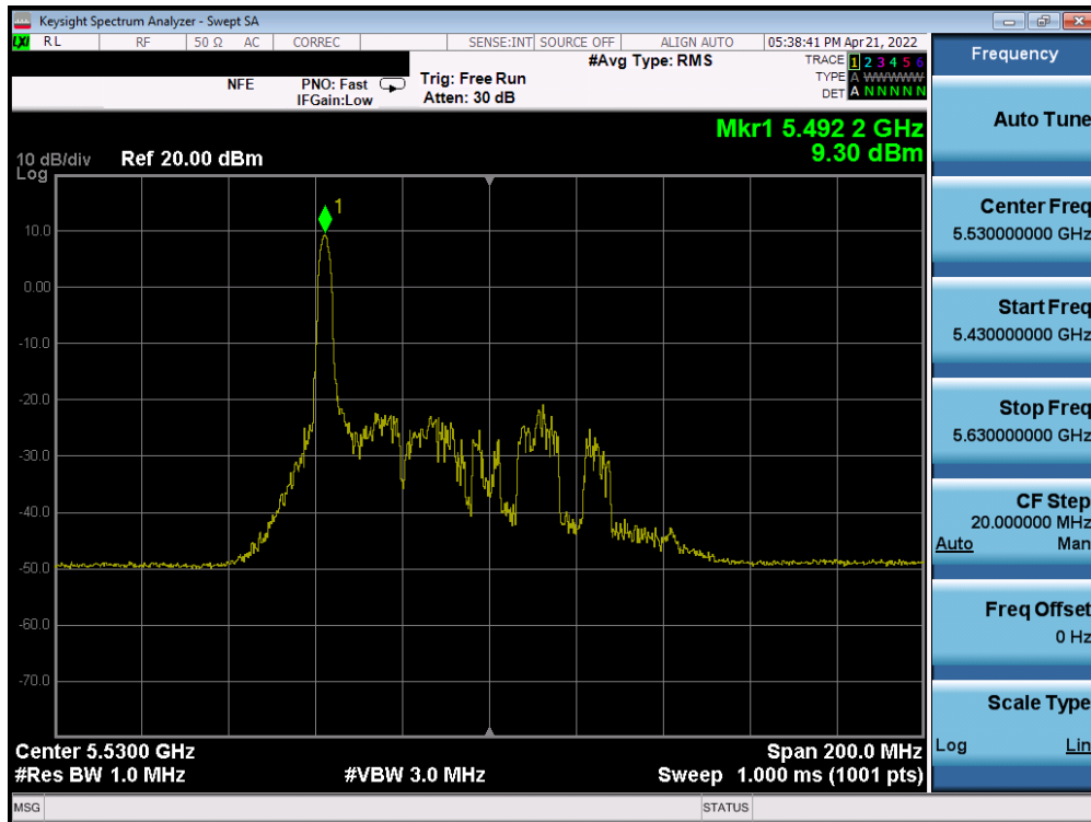
Plot 7-197. Power Spectral Density Plot SISO ANT2 (80MHz BW 802.11ax – 26 Tones (UNII Band 2C) – Ch. 106)
