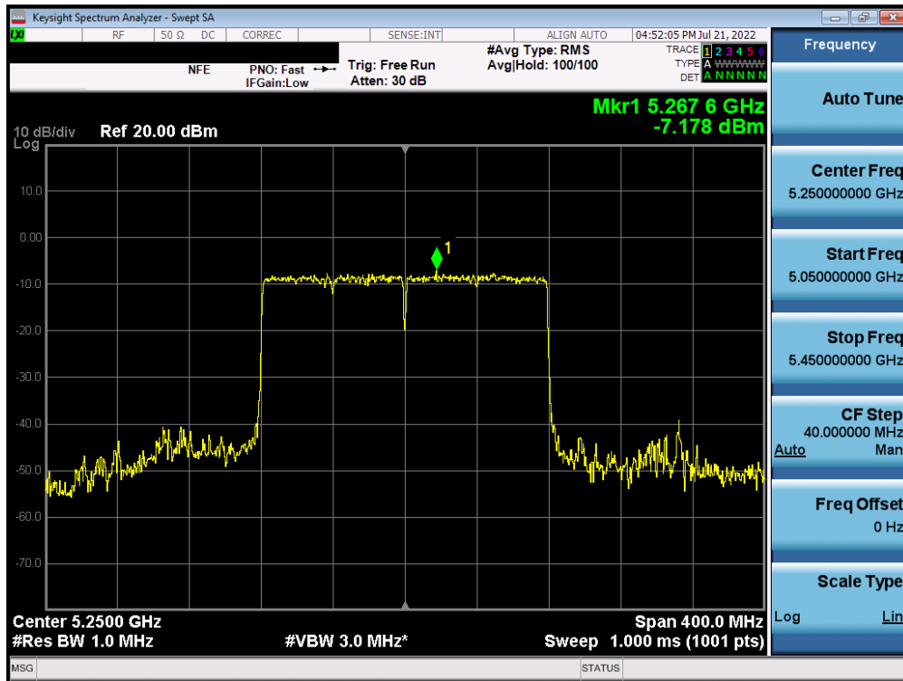
Plot 7-214. Power Spectral Density Plot SISO ANT2 (160MHz BW 802.11ax – Full Tones (UNII Band 1/2A) – Ch. 50)
