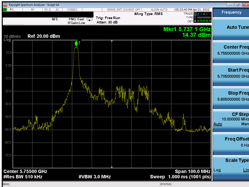
Plot 7-205. Power Spectral Density Plot SISO ANT2 (40MHz BW 802.11ax – 26 Tones (UNII Band 3) – Ch. 151)
