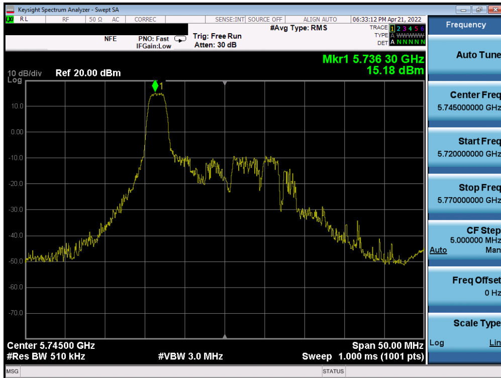
Plot 7-142. Power Spectral Density Plot SISO ANT1 (20MHz BW 802.11ax – 26 Tones (UNII Band 3) – Ch. 149)
