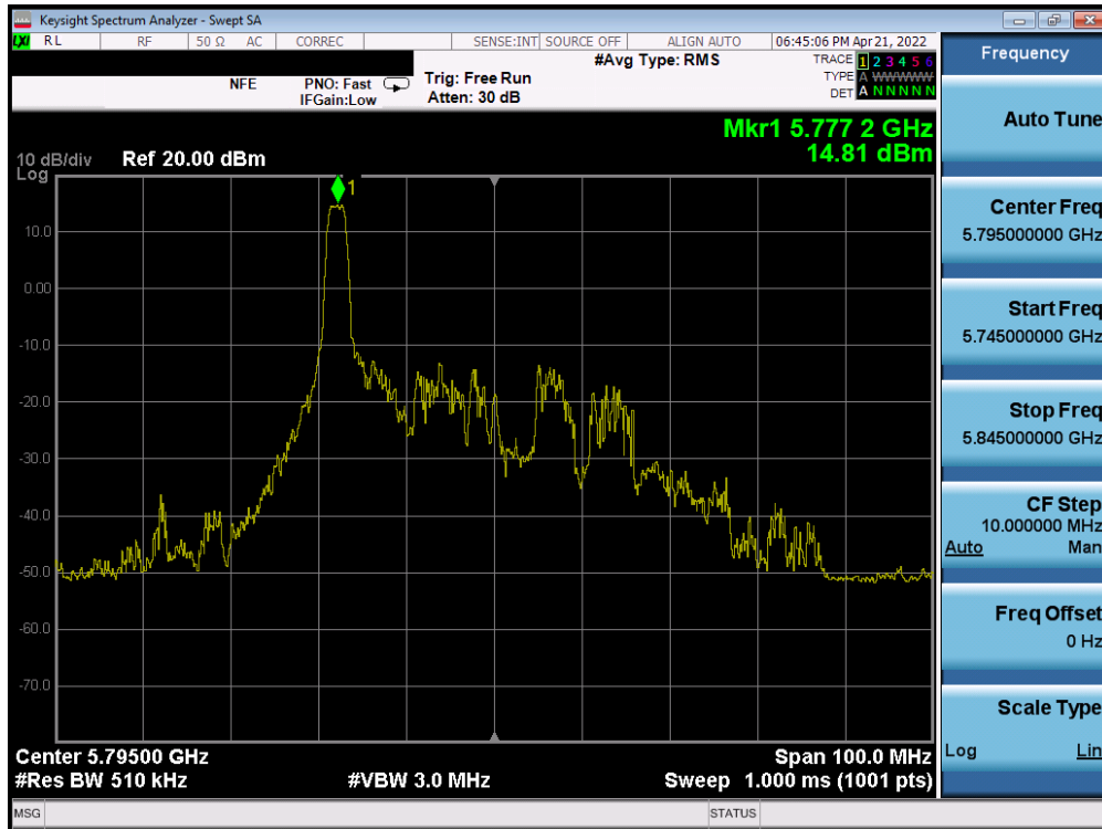
Plot 7-146. Power Spectral Density Plot SISO ANT1 (40MHz BW 802.11ax – 26 Tones (UNII Band 3) – Ch. 159)
