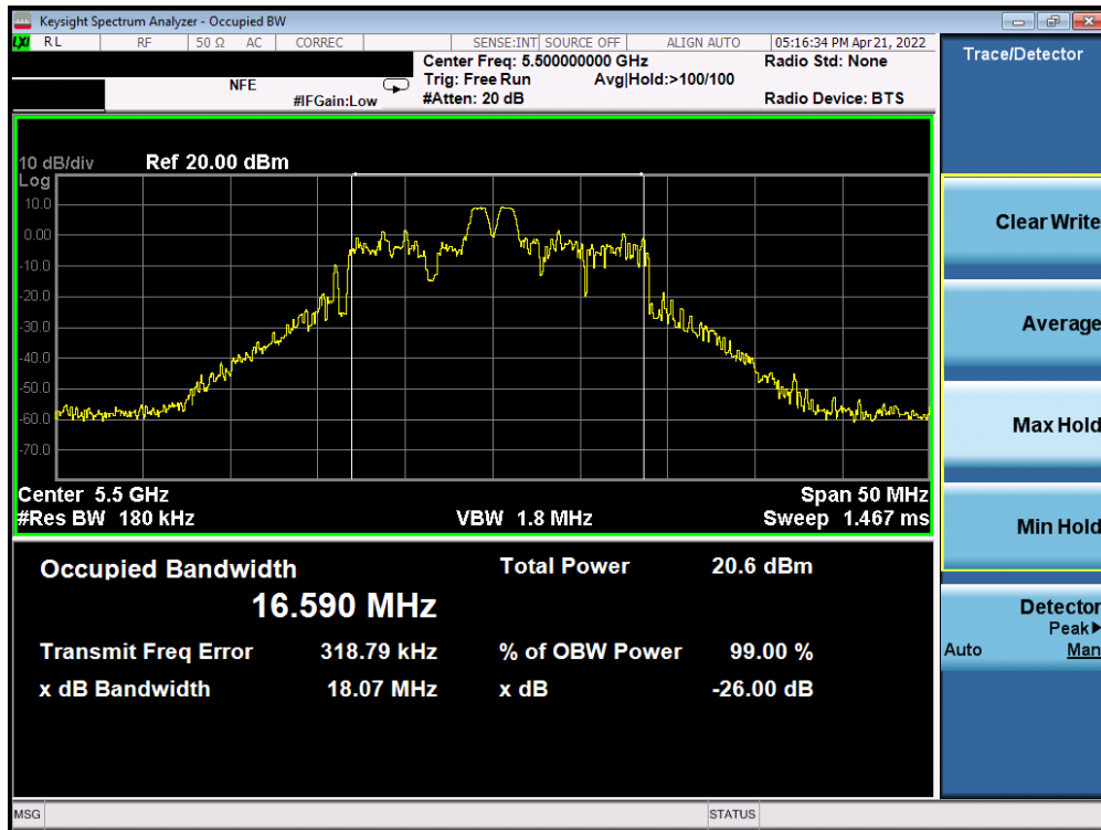
Plot 7-61. 26dB Bandwidth Plot SISO ANT2 (20MHz BW 802.11ax – 26 Tones (UNII Band 2C) – Ch. 100)
