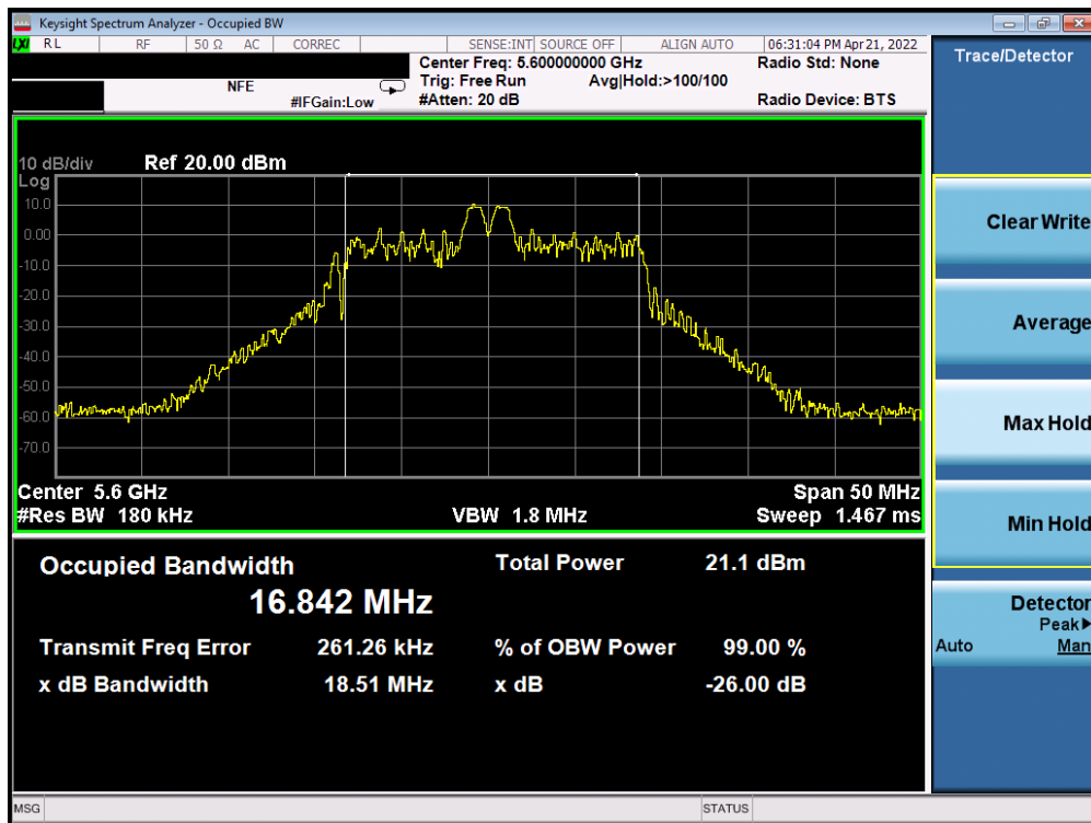
Plot 7-16. 26dB Bandwidth Plot SISO ANT1 (20MHz BW 802.11ax – 26 Tones (UNII Band 2C) – Ch. 120)
