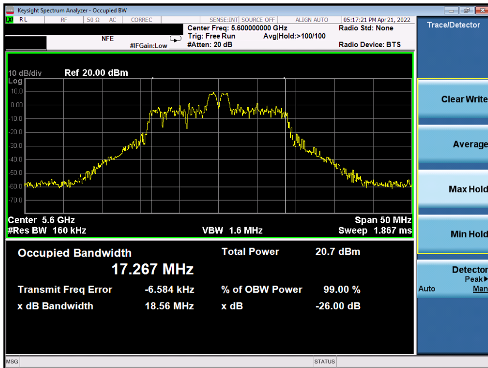
Plot 7-62. 26dB Bandwidth Plot SISO ANT2 (20MHz BW 802.11ax – 26 Tones (UNII Band 2C) – Ch. 120)
