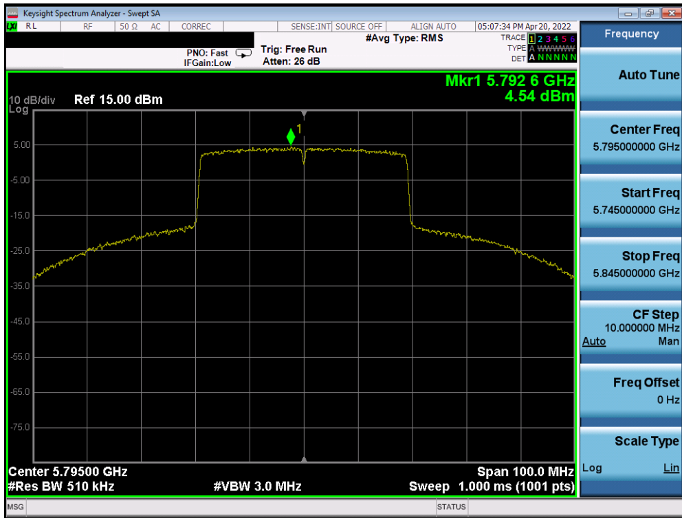
Plot 7-278. Power Spectral Density Plot SISO ANT2 (40MHz BW 802.11ax (UNII Band 3) – Ch. 159)
