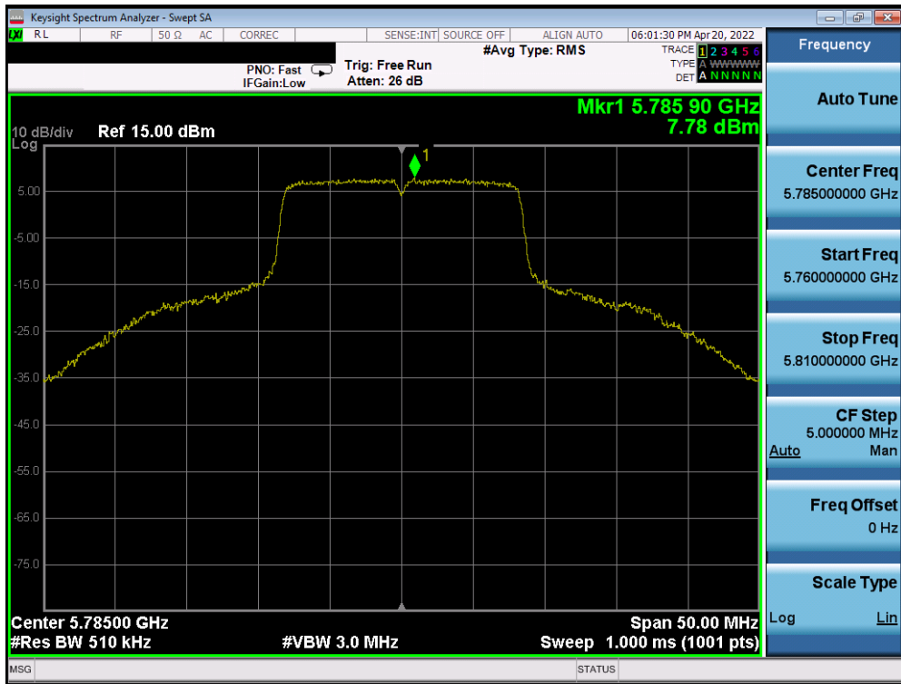
Plot 7-197. Power Spectral Density Plot SISO ANT1 (802.11a (UNII Band 3) – Ch. 157)
