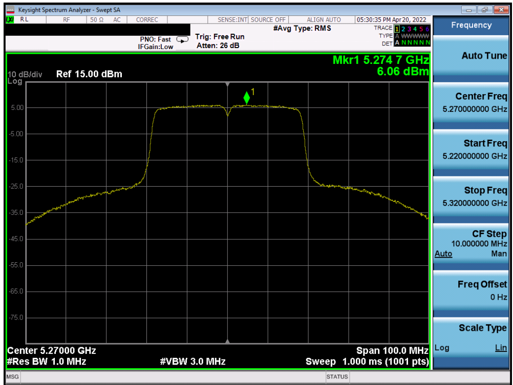
Plot 7-237. Power Spectral Density Plot SISO ANT2 (40MHz BW 802.11n (UNII Band 2A) – Ch. 54)
