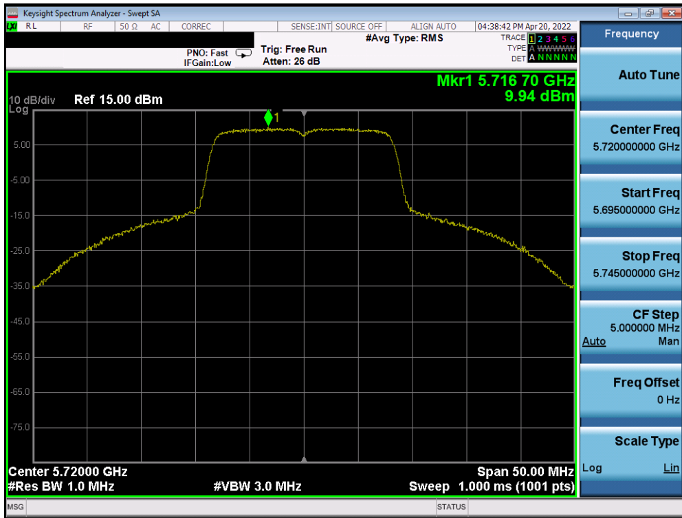
Plot 7-245. Power Spectral Density Plot SISO ANT2 (802.11a (UNII Band 2C) – Ch. 144)
