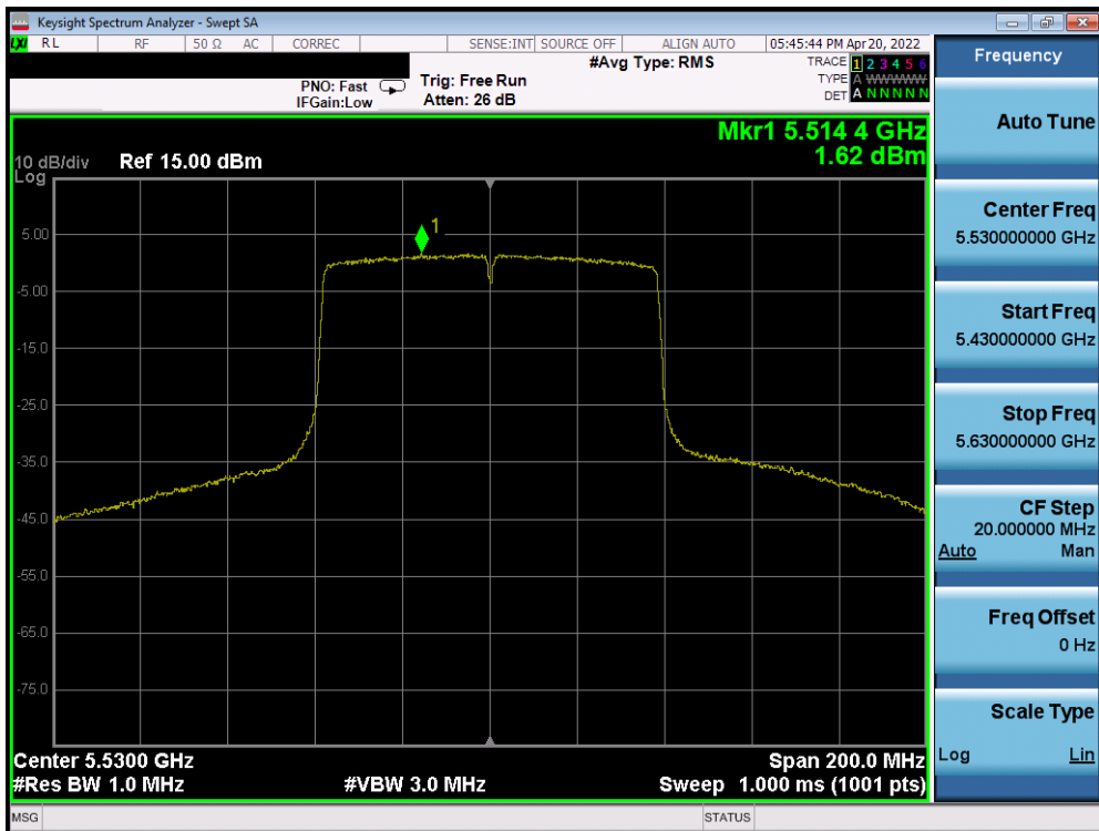
Plot 7-258. Power Spectral Density Plot SISO ANT2 (80MHz BW 802.11ac (UNII Band 2C) – Ch. 106)
