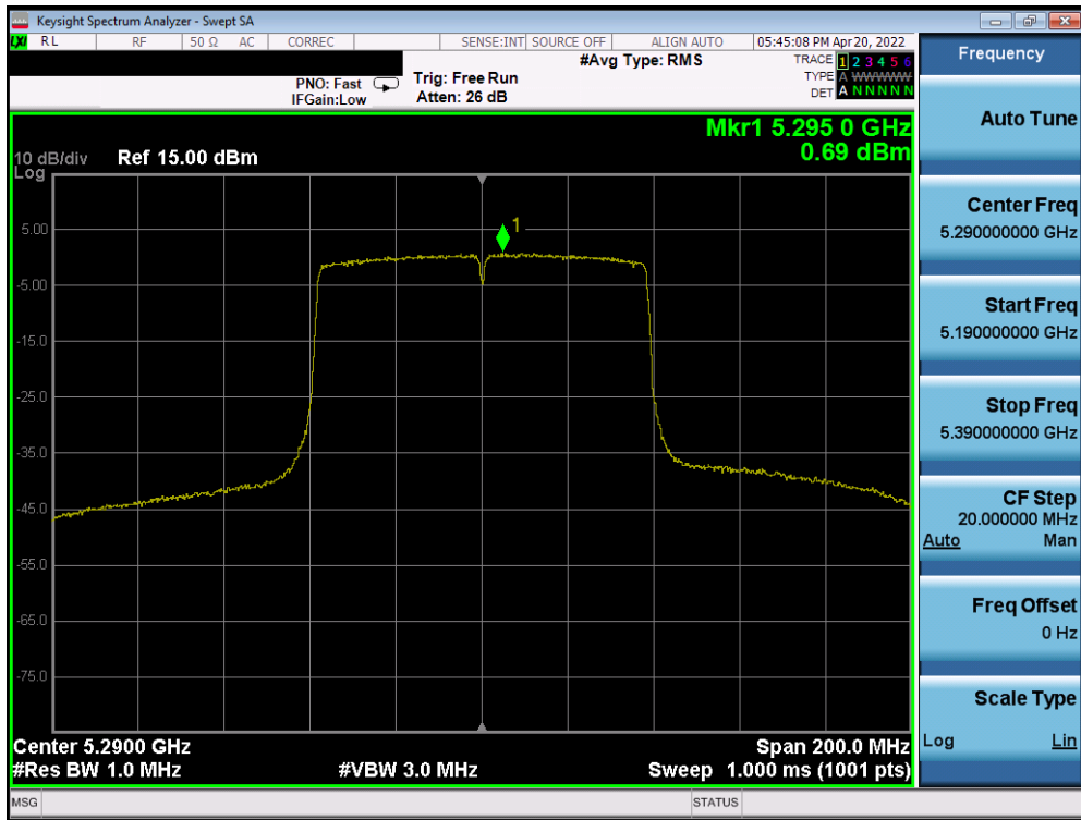
Plot 7-241. Power Spectral Density Plot SISO ANT2 (80MHz BW 802.11ac (UNII Band 2A) – Ch. 58)
