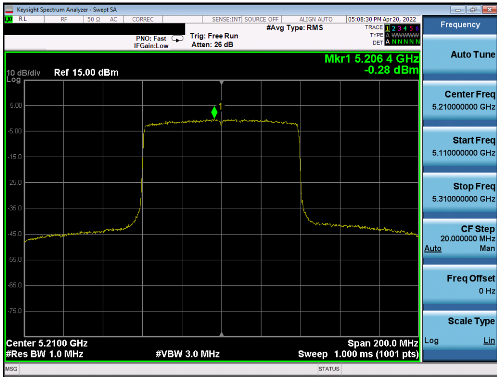
Plot 7-225. Power Spectral Density Plot SISO ANT2 (80MHz BW 802.11ax (UNII Band 1) – Ch. 42)
