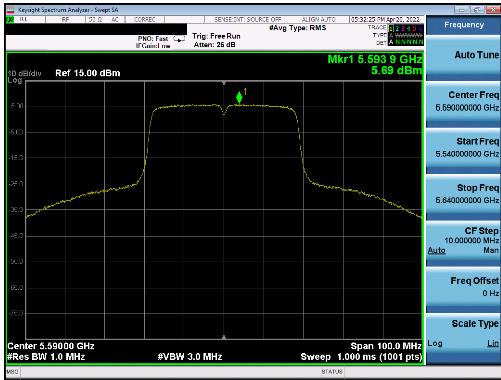
Plot 7-253. Power Spectral Density Plot SISO ANT2 (40MHz BW 802.11n (UNII Band 2C) – Ch. 118)
