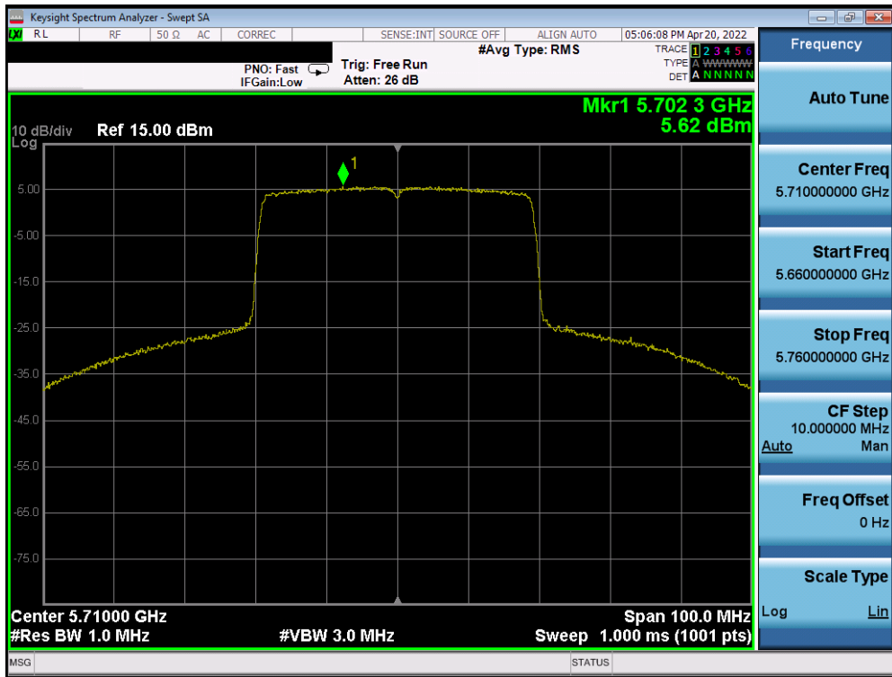
Plot 7-257. Power Spectral Density Plot SISO ANT2 (40MHz BW 802.11ax (UNII Band 2C) – Ch. 142)
