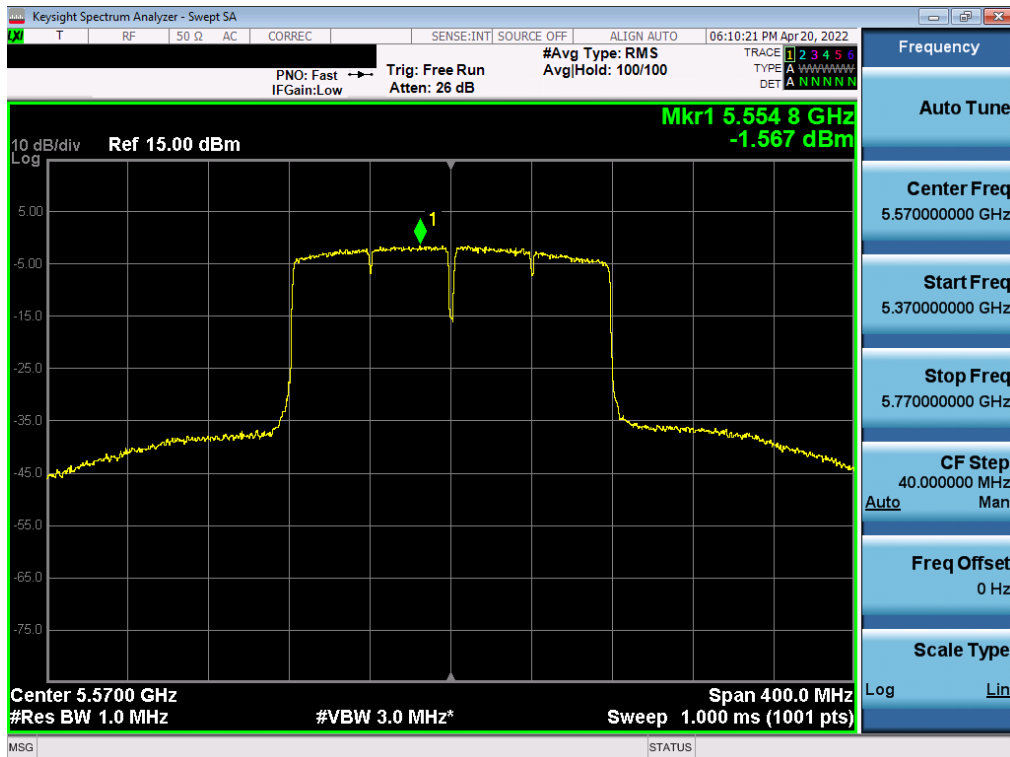
Plot 7-264. Power Spectral Density Plot SISO ANT2 (160MHz BW 802.11ac (UNII Band 2C) – Ch. 114)
