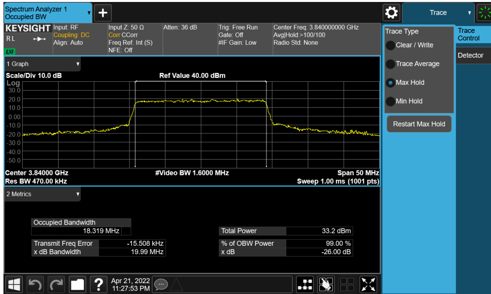
Plot 7-26. Occupied Bandwidth Plot (NR Band n77 - 20MHz QPSK - Full RB - ANT2)
