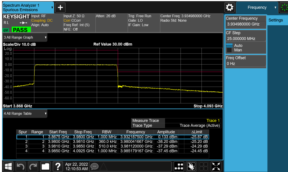
Plot 7-76. Upper ACP Plot (NR Band n77 - 90MHz CP-OFDM-QPSK – Full RB - ANT2)
