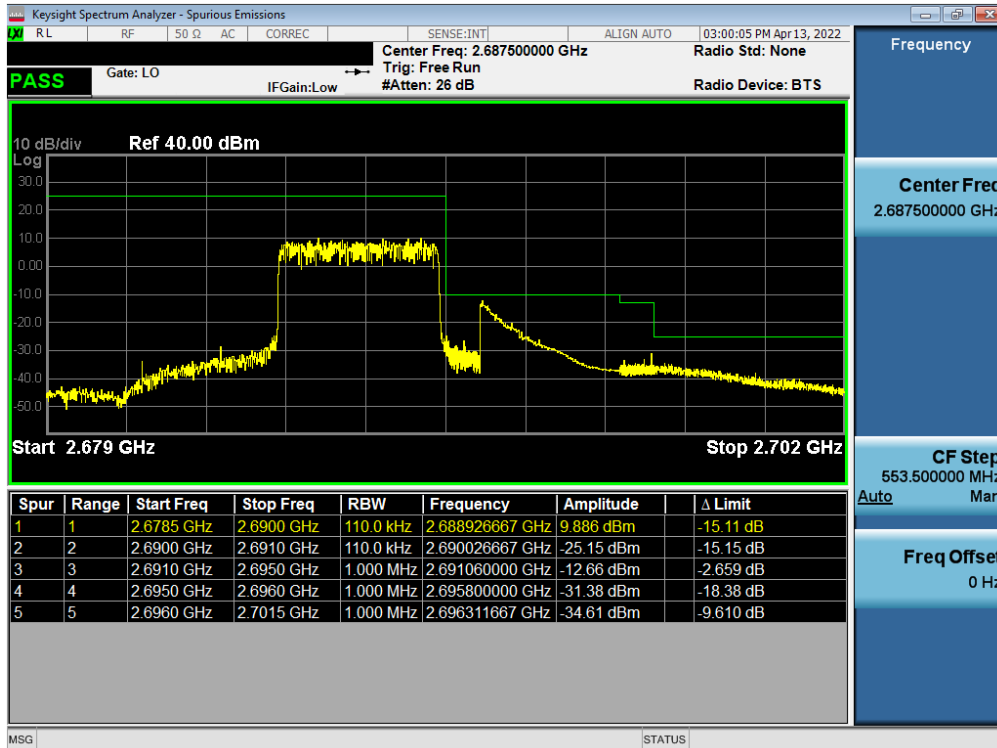
Plot 7-191. Upper ACP Plot (LTE Band 41(PC2) - 5MHz QPSK - Full RB - Ant1)
