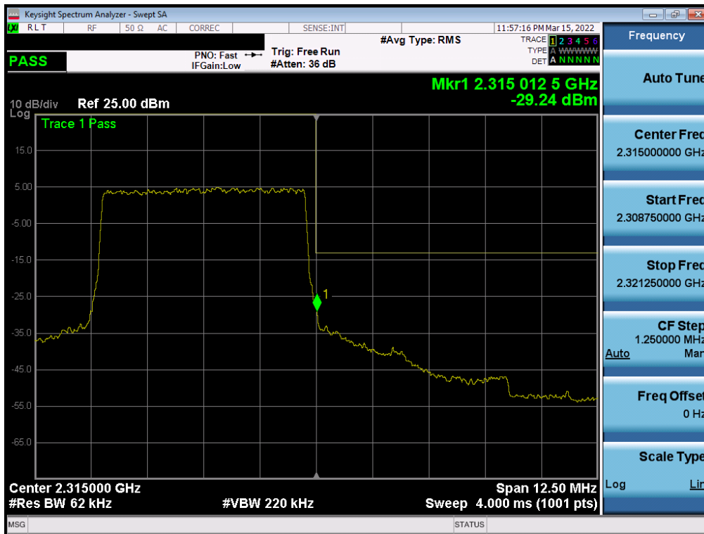
Plot 7-174. Upper Band Edge Plot (LTE Band 30 - 5MHz QPSK – Full RB - Ant1)
